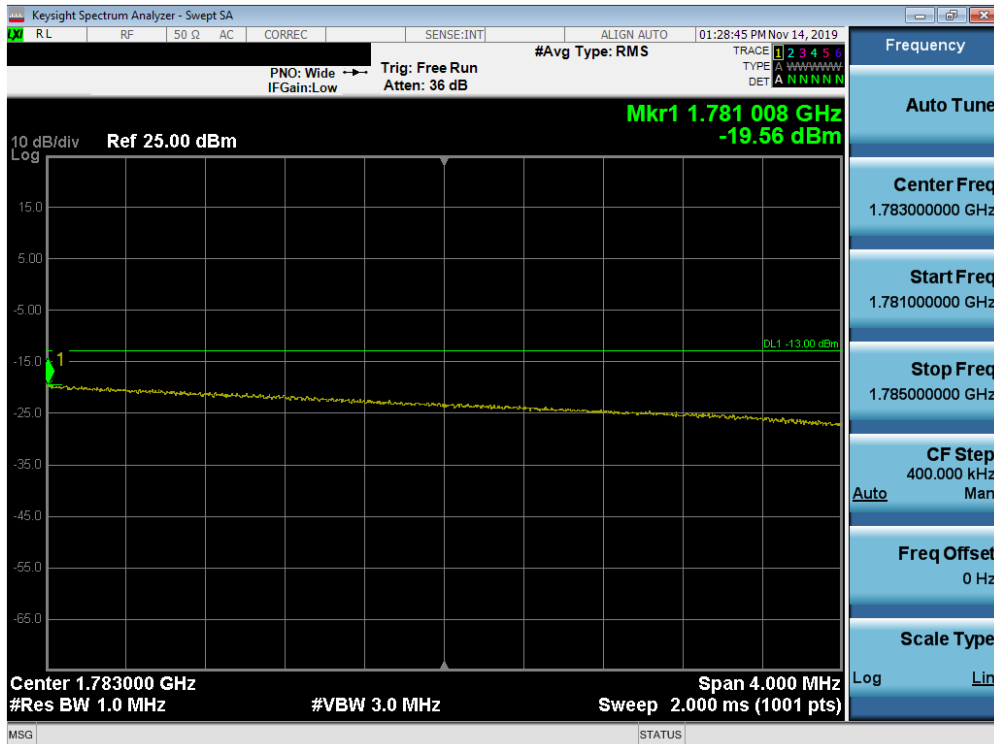
Plot 7-674. Upper Extended Band Edge Plot (Band n66 - 10.0MHz CP-OFDM-QPSK - Full RB Configuration)
