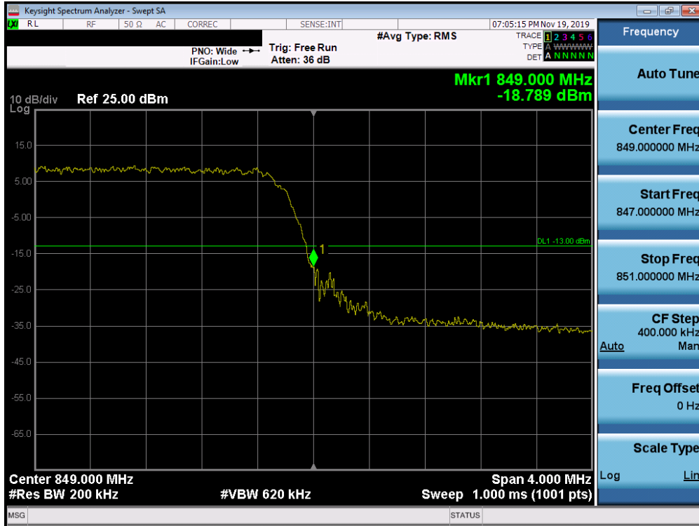
Plot 7-652. Upper Band Edge Plot (n5 - 5MHz CP-OFDM-QPSK - Full RB Configuration)
