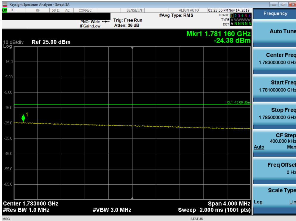
Plot 7-678. Upper Extended Band Edge Plot (Band n66 - 15.0MHz CP-OFDM-QPSK - Full RB Configuration)
