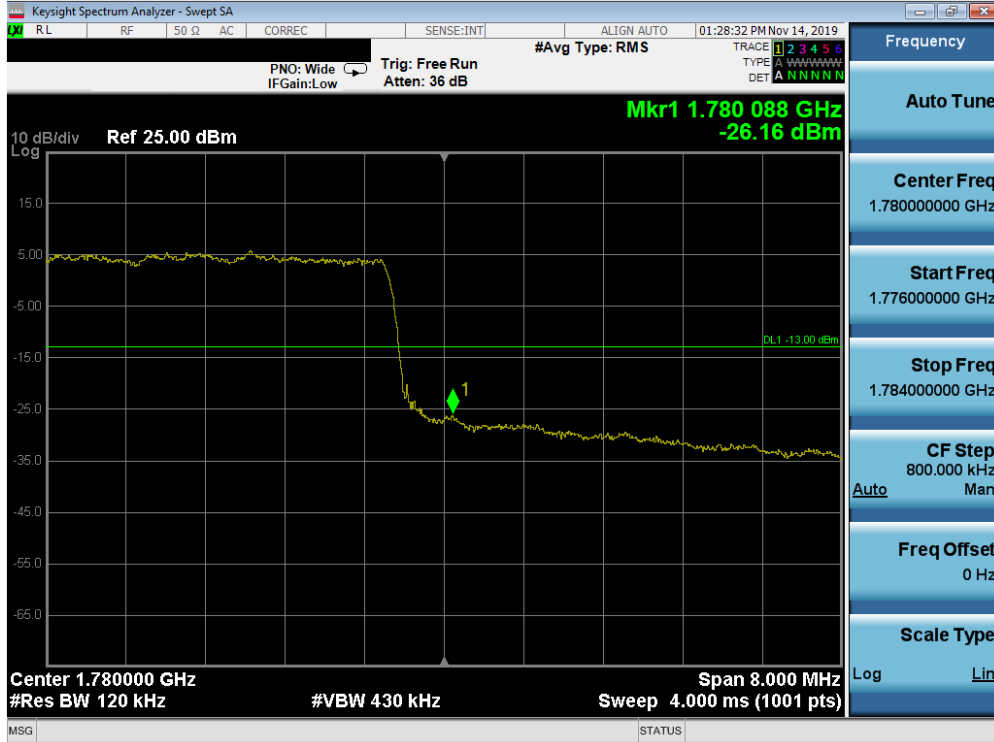
Plot 7-673. Upper Band Edge Plot (Band n66 - 10.0MHz CP-OFDM-QPSK - Full RB Configuration)
