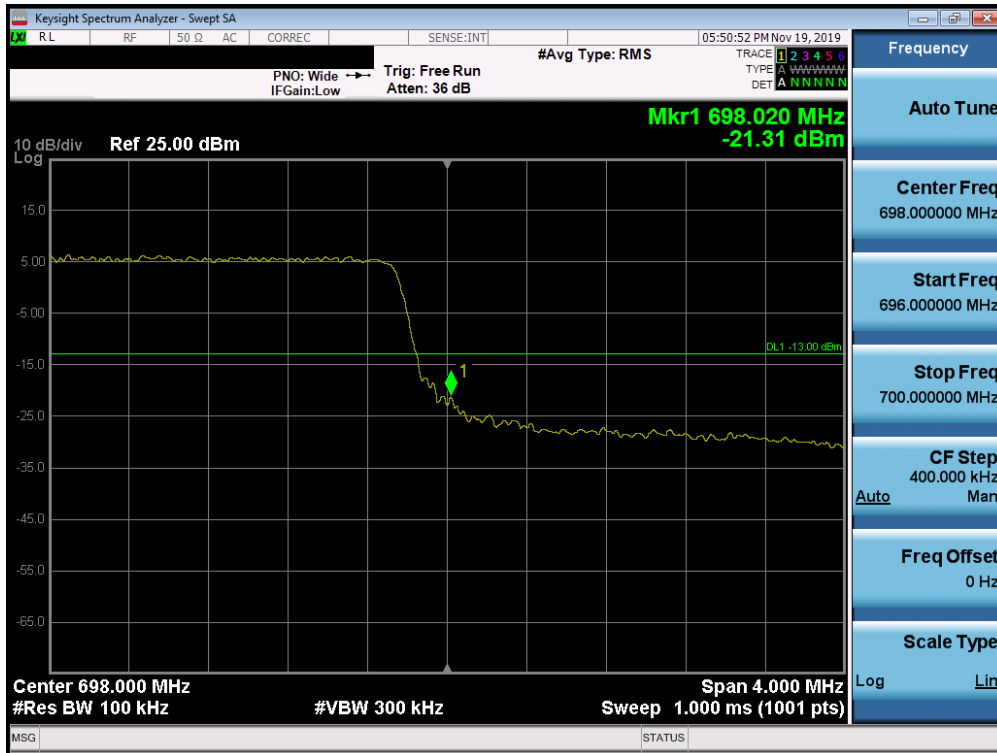
Plot 7-660. Upper Band Edge Plot (n71 - 5MHz CP-OFDM-QPSK - Full RB Configuration)
