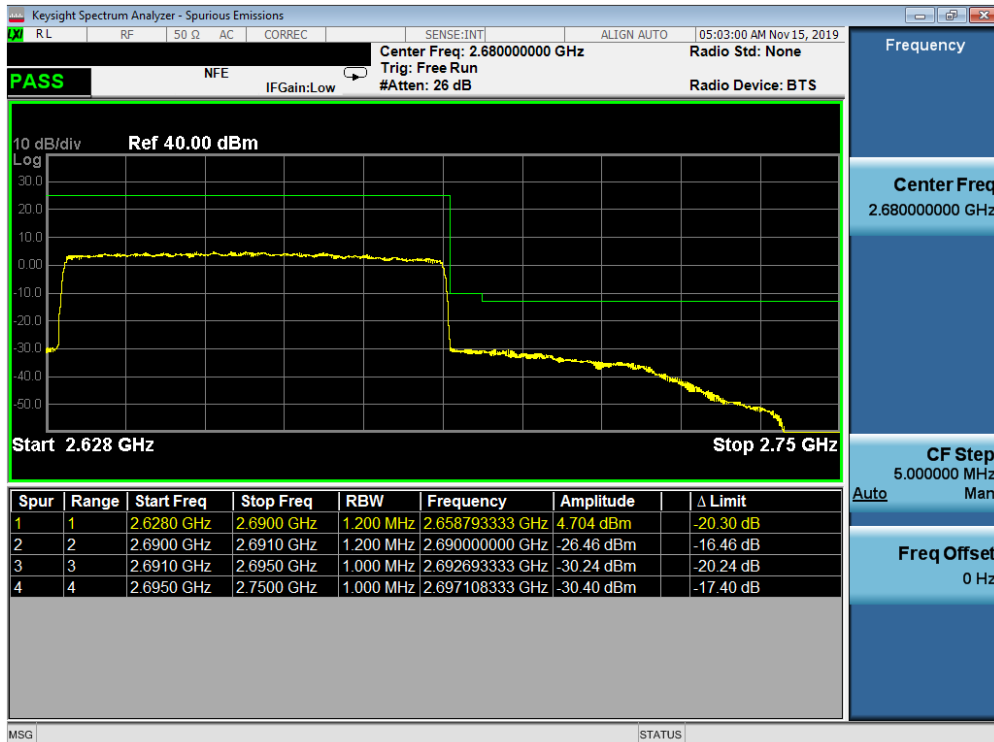
Plot 7-706. Upper ACP Plot (n41 - 60MHz CP-OFDM-QPSK - Full RB Configuration)
