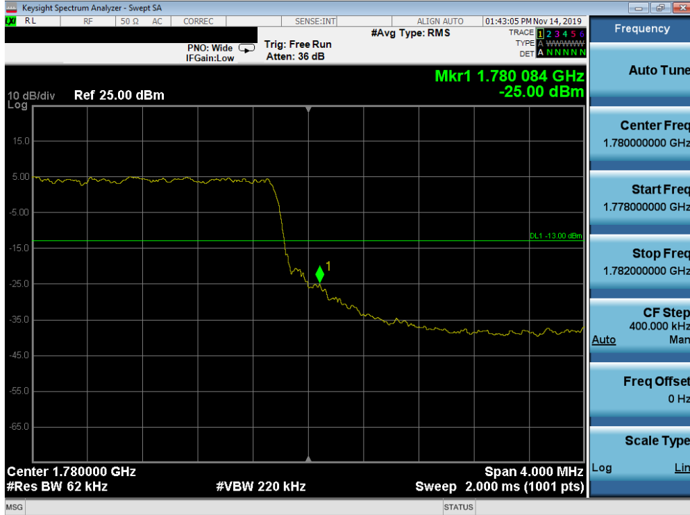
Plot 7-669. Upper Band Edge Plot (Band n66 - 5.0MHz CP-OFDM-QPSK - Full RB Configuration)
