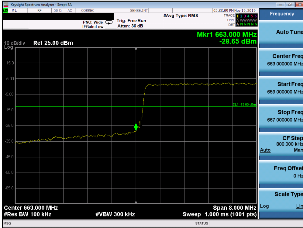
Plot 7-661. Lower Band Edge Plot (n71 - 10MHz CP-OFDM-QPSK - Full RB Configuration)
