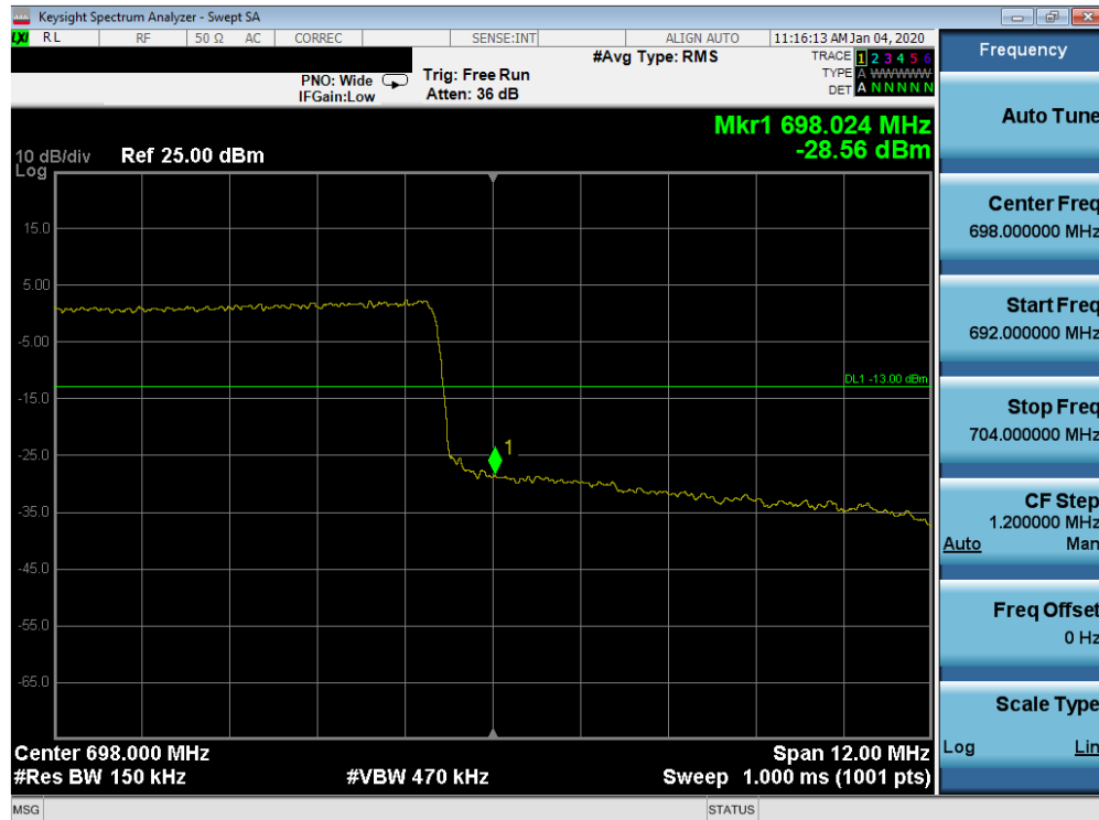
Plot 7-664. Upper Band Edge Plot (n71 - 15MHz CP-OFDM-QPSK - Full RB Configuration)
