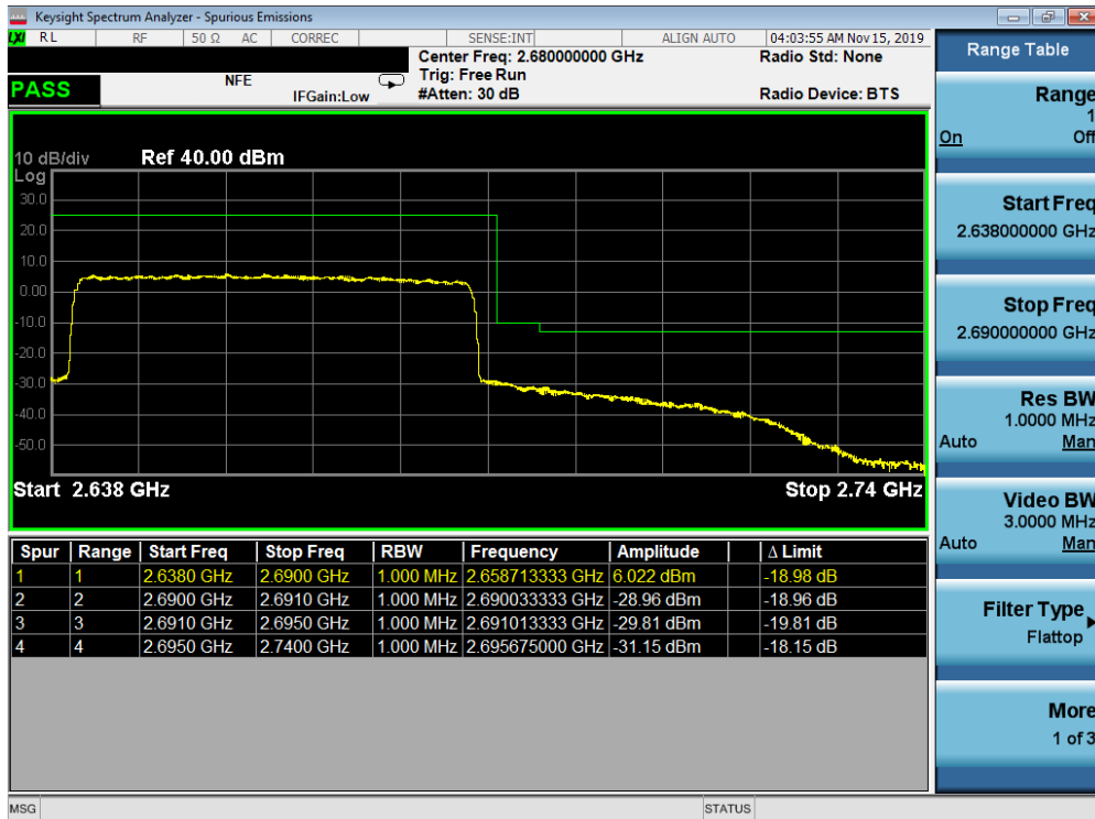
Plot 7-704. Upper ACP Plot (n41 - 50MHz CP-OFDM-QPSK - Full RB Configuration)
