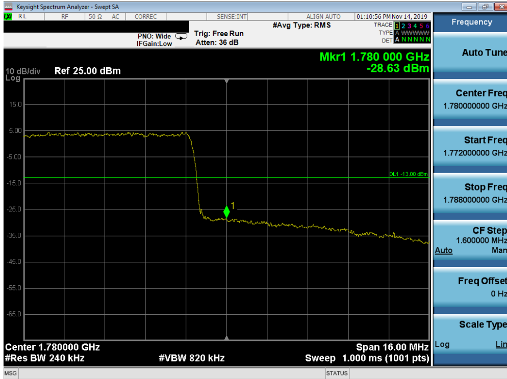
Plot 7-681. Upper Band Edge Plot (Band n66 - 20.0MHz CP-OFDM-QPSK - Full RB Configuration)
