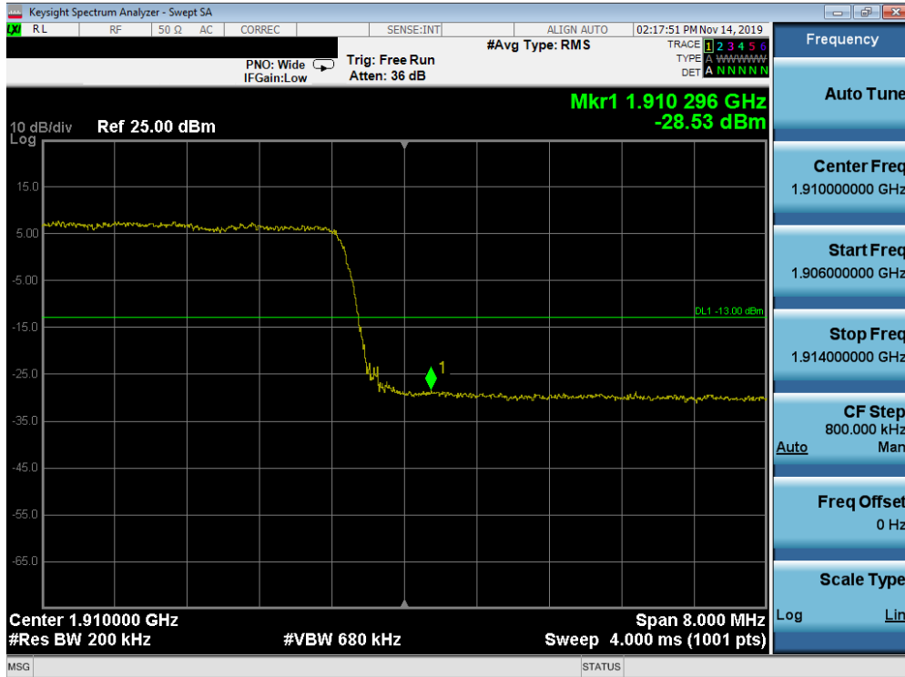
Plot 7-689. Upper Band Edge Plot (Band n2 - 10.0MHz CP-OFDM-QPSK - Full RB Configuration)
