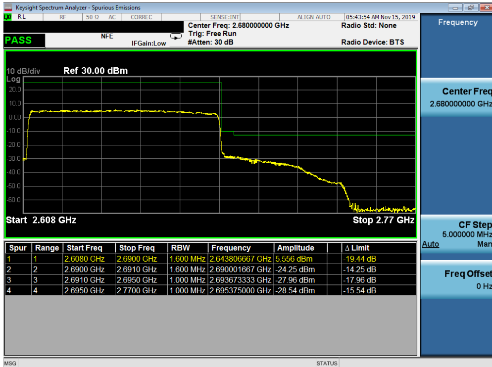
Plot 7-708. Upper ACP Plot (n41 - 80MHz CP-OFDM-QPSK - Full RB Configuration)
