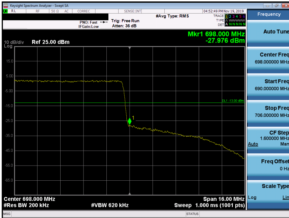
Plot 7-666. Upper Band Edge Plot (n71- 20MHz CP-OFDM-QPSK - Full RB Configuration)
