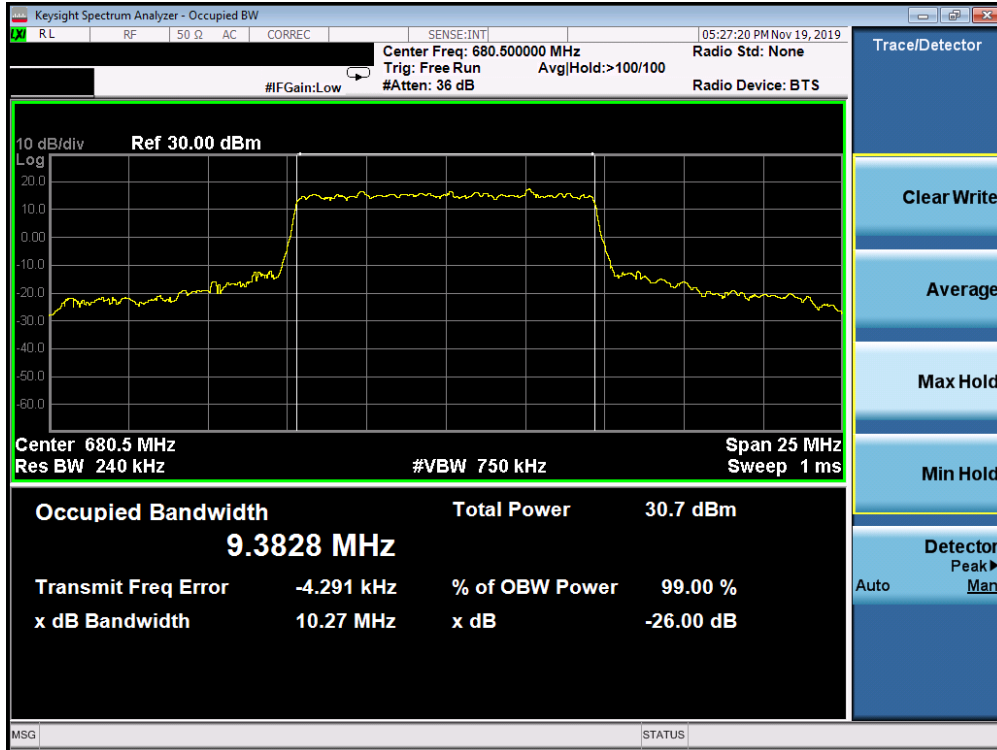
Plot 7-534. Occupied Bandwidth Plot (n71 10MHz QPSK-CP-OFDM - Full RB Configuration)
