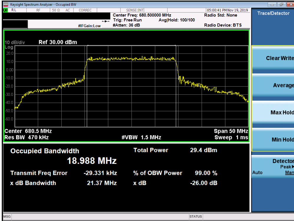
Plot 7-544. Occupied Bandwidth Plot (n71 20MHz 64QAM-CP-OFDM- Full RB Configuration)
