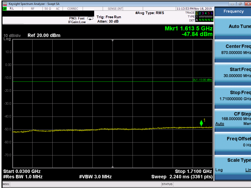
Plot 7-451. Conducted Spurious Plot (Band 66 – 20.0MHz QPSK – PCC 1/99 SCC 1/0 – Mid Channel)
