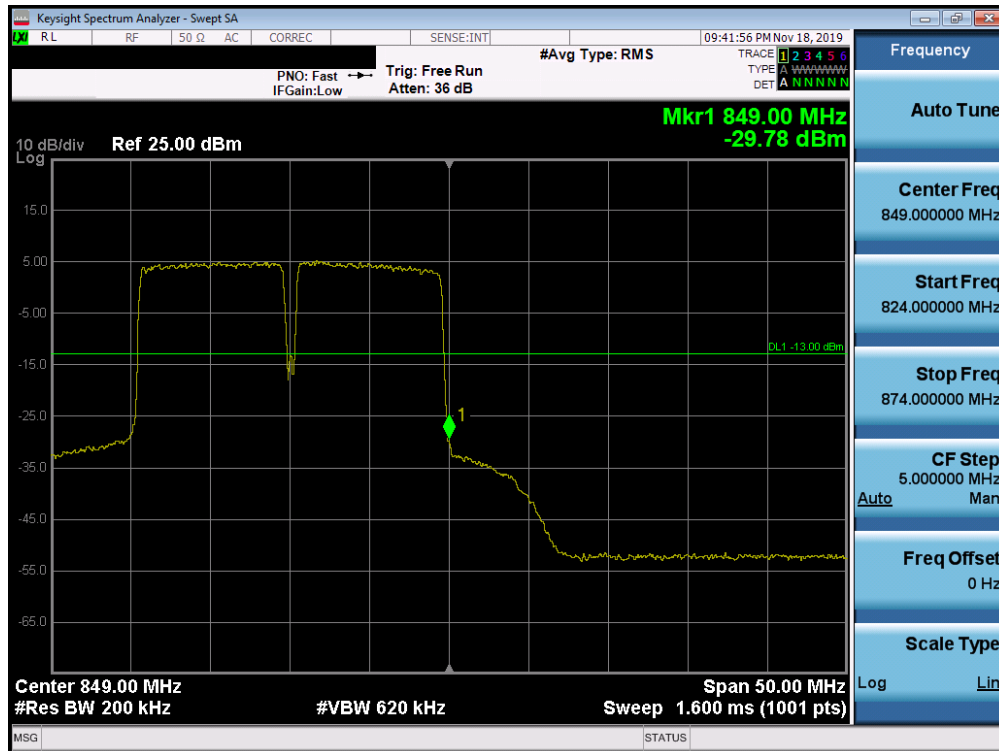
Plot 7-446. Upper Band Edge Plot (Band 5 QPSK – PCC:10 MHz SCC:10 MHz – Full RB)
