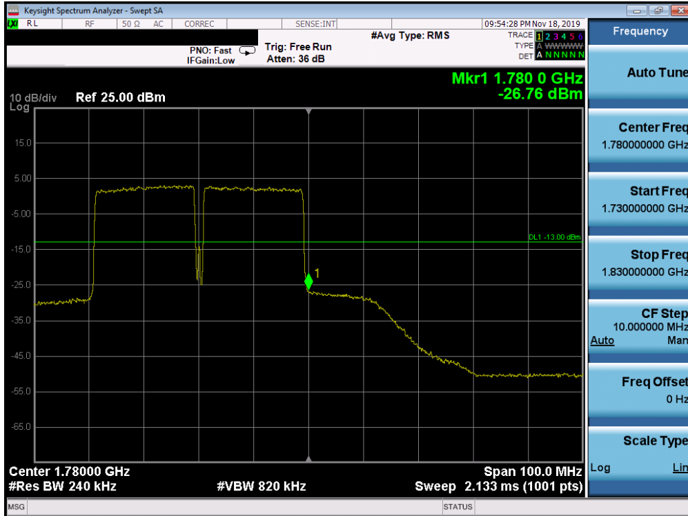
Plot 7-461. Upper Band Edge Plot (Band 66 QPSK – PCC:20 MHz SCC:20 MHz – Full RB)
