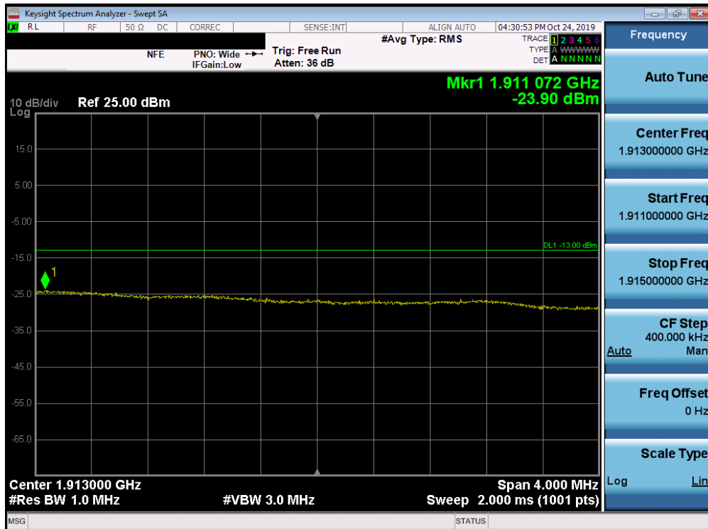
Plot 7-340. Upper Extended Band Edge Plot (Band 2 - 15.0MHz QPSK - Full RB Configuration)
