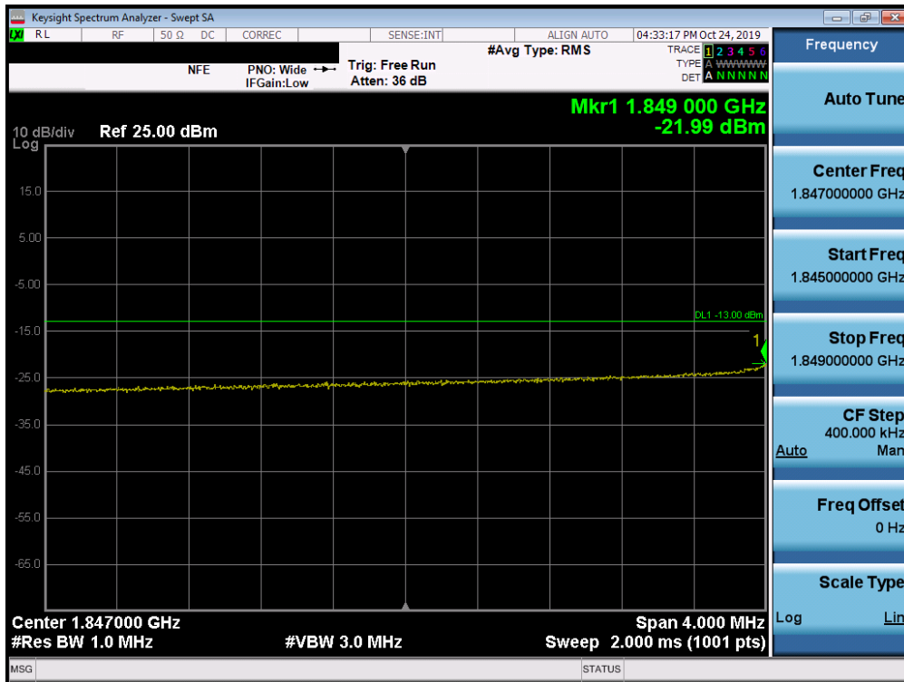
Plot 7-332. Lower Extended Band Edge Plot (Band 25/2 – 10.0MHz QPSK - Full RB Configuration)
