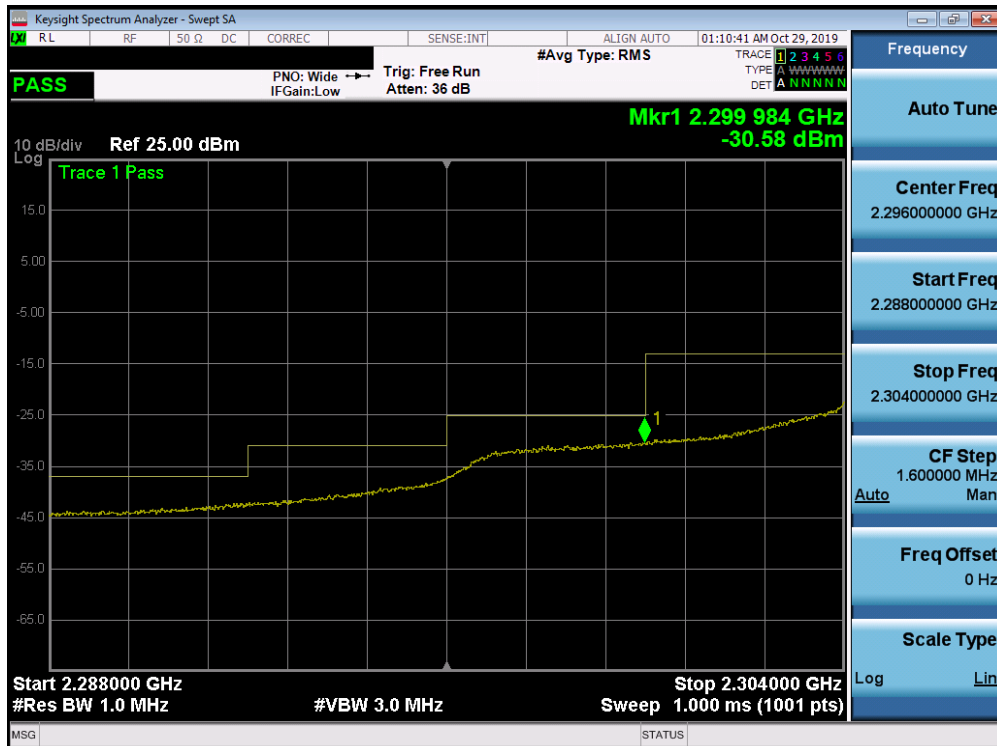
Plot 7-354. Lower Extended Band Edge Plot (Band 30 - 10.0MHz QPSK - Full RB Configuration)
