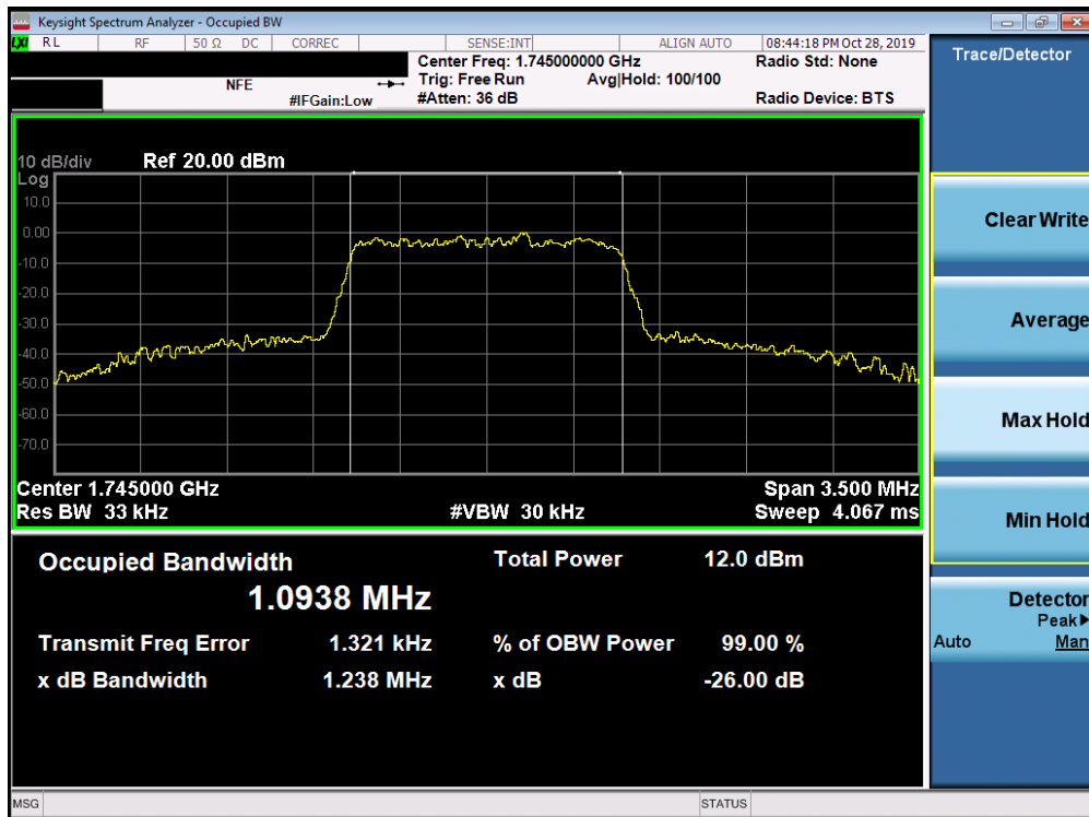
Plot 7-62. Occupied Bandwidth Plot (Band 66/4 - 1.4MHz 16-QAM - Full RB Configuration)
