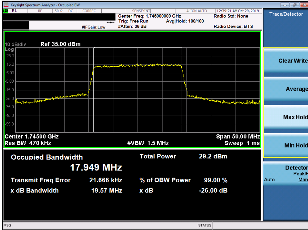
Plot 7-83. Occupied Bandwidth Plot (Band 66/4 - 20.0MHz 64-QAM - Full RB Configuration)
