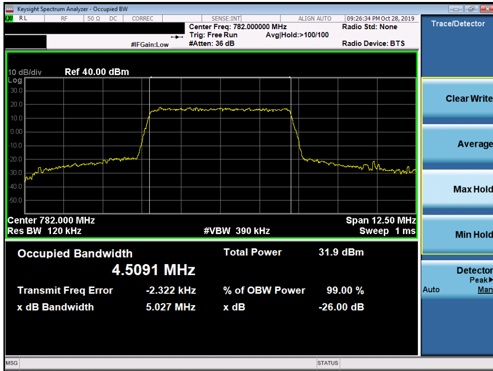
Plot 7-33. Occupied Bandwidth Plot (Band 13 - 5.0MHz QPSK - Full RB Configuration)
