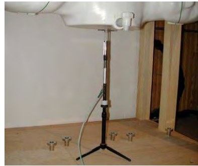
Figure 10-2 System Verification Setup Photo
