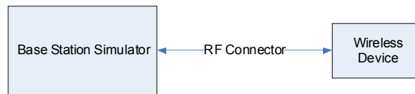
Figure 9-3 Power Measurement Setup
