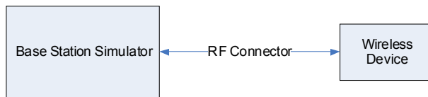
Figure 9-1 Power Measurement Setup
