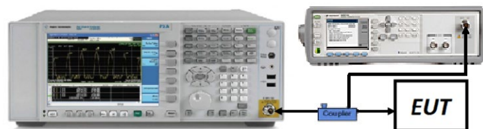
Figure 7-3. Test Instrument & Measurement Setup
