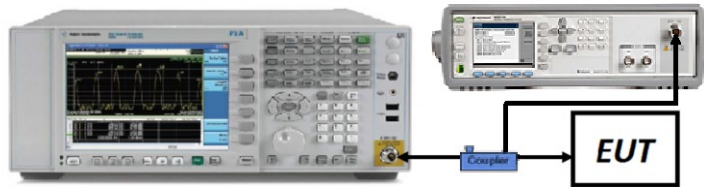
Figure 7-4. Test Instrument & Measurement Setup
