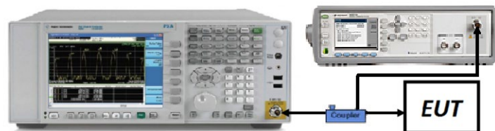
Figure 7-6. Test Instrument & Measurement Setup
