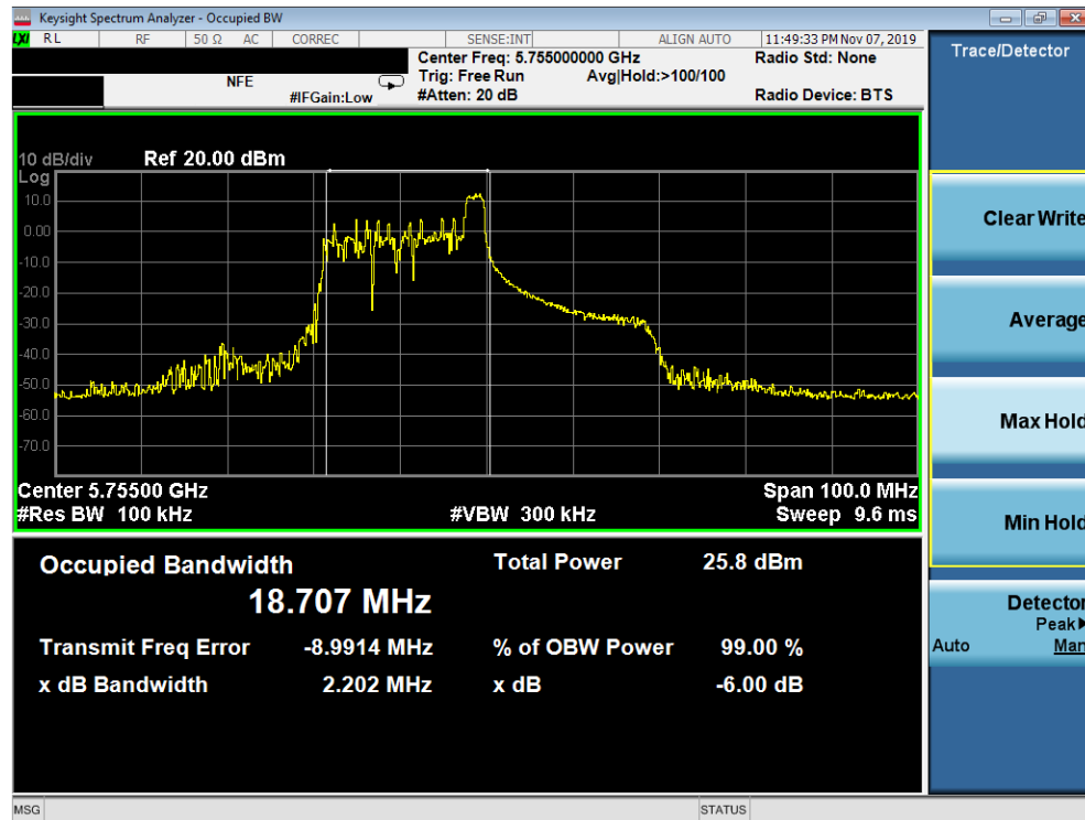
Plot 7-52. 6dB Bandwidth Plot SISO ANT2 (40MHz BW 802.11ax – 26 Tones (UNII Band 3) – Ch. 151)
