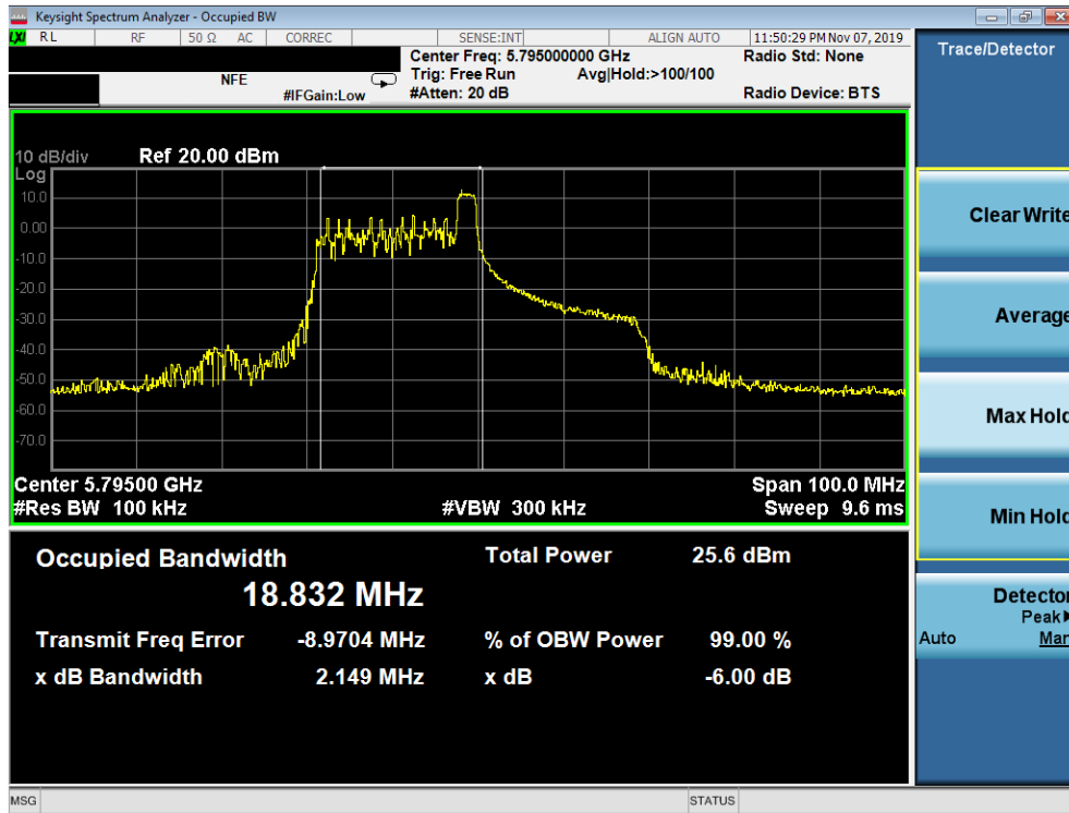
Plot 7-53. 6dB Bandwidth Plot SISO ANT2 (40MHz BW 802.11ax – 26 Tones (UNII Band 3) – Ch. 159)
