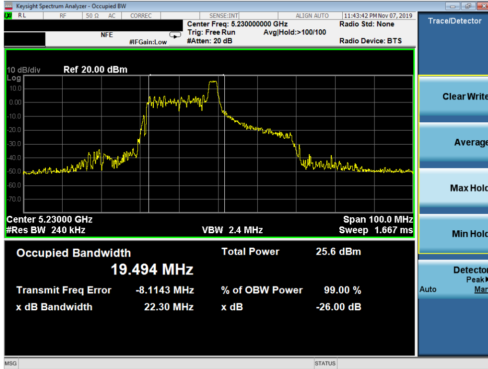
Plot 7-26. 26dB Bandwidth Plot SISO ANT2 (40MHz BW 802.11ax – 26 Tones (UNII Band 1) – Ch. 46)
