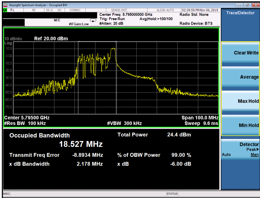
Plot 7-47. 6dB Bandwidth Plot SISO ANT1 (40MHz BW 802.11ax – 26 Tones (UNII Band 3) – Ch. 159)
