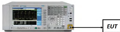
Figure 7-4. Test Instrument & Measurement Setup
