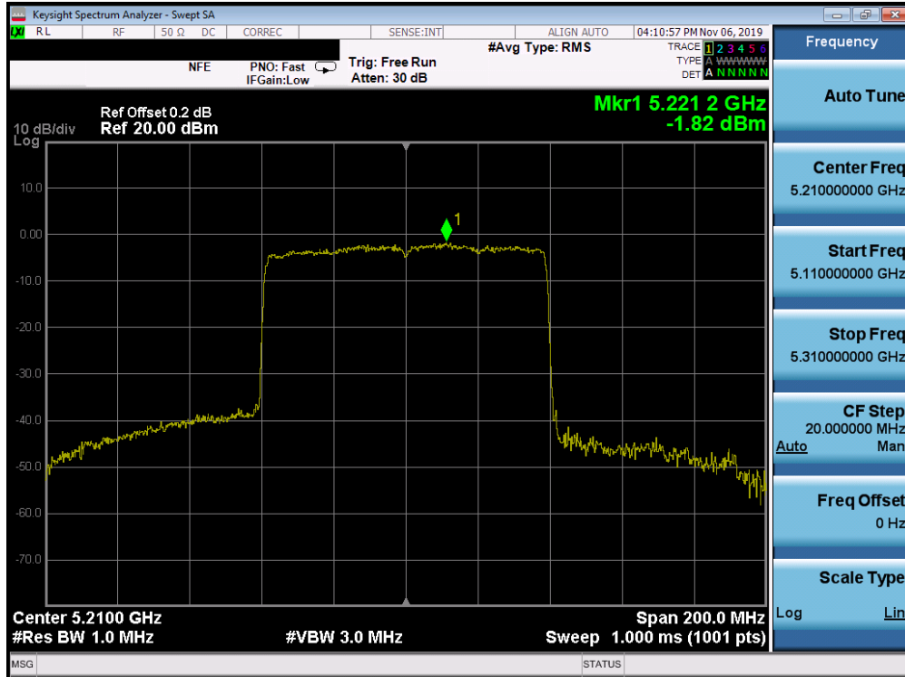
Plot 7-147. Power Spectral Density Plot SISO ANT1 (80MHz BW 802.11ax (UNII Band 1) – Ch. 42)
