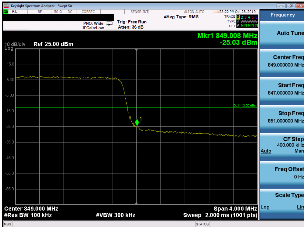
Plot 7-117. Upper Band Edge Plot (Band 5 - 5.0MHz QPSK - Full RB Configuration)
