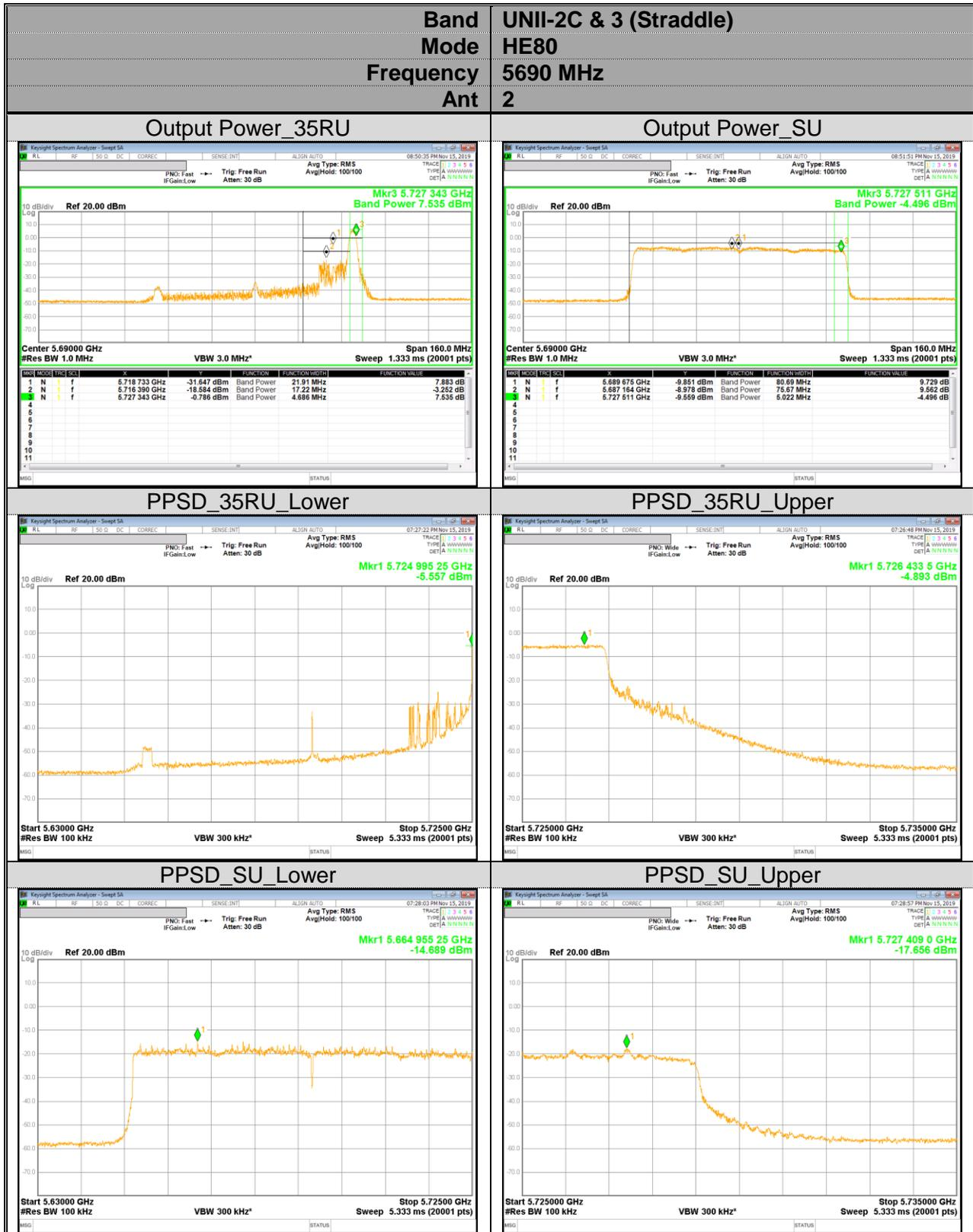
10.2.20. TEST PLOT\_802.11ax 2Tx (MIMO) MODE 5.8 GHz BAND
