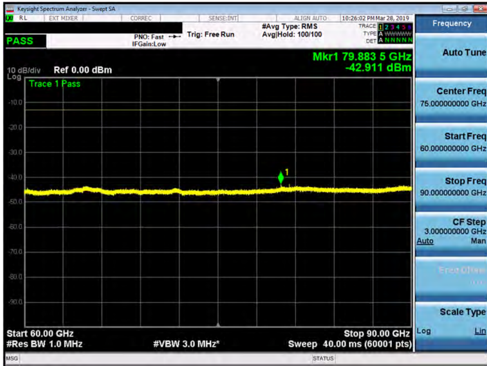
Plot 7-187. L Patch Radiated Spurious Plot 60-90 GHz (1CC QPSK High Channel H Beam)
