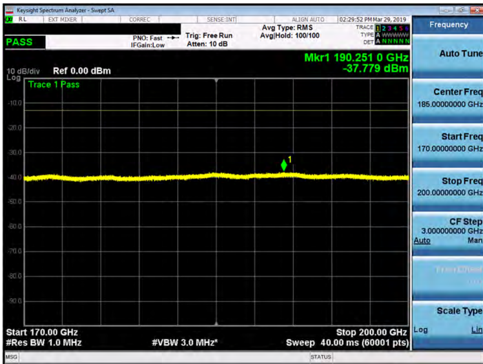
Plot 7-166. K Patch Radiated Spurious Plot 170-200 GHz (1CC QPSK Low Channel V Beam)
