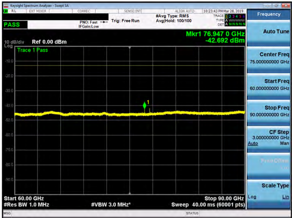
Plot 7-186. L Patch Radiated Spurious Plot 60-90 GHz (1CC QPSK Mid Channel H Beam)
