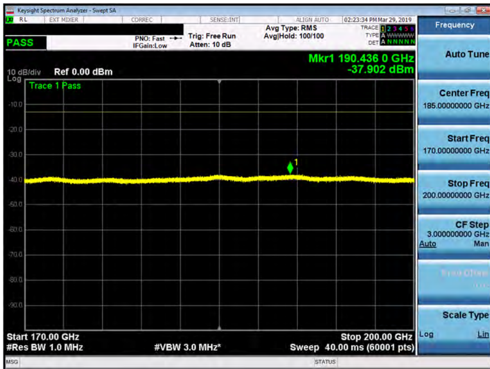
Plot 7-126. J Patch Radiated Spurious Plot 170-200 GHz (1CC QPSK Low Channel V Beam)
