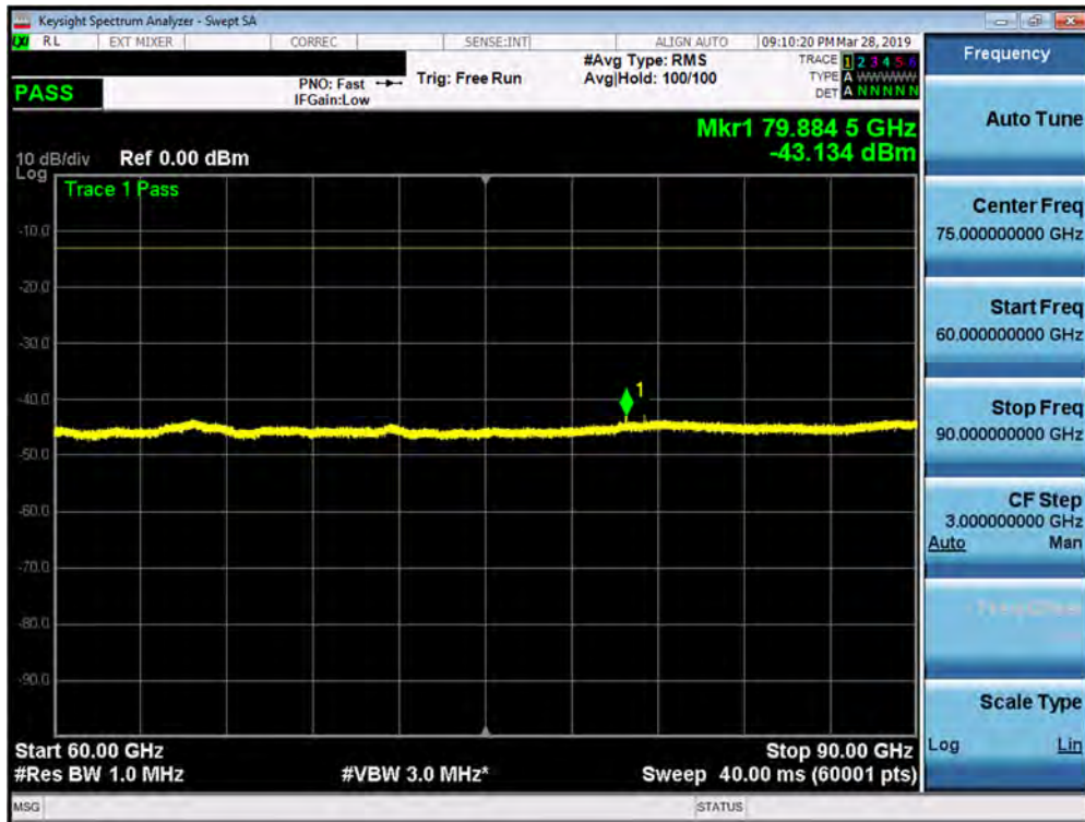
Plot 7-70. J Dipole Radiated Spurious Plot 60-90 GHz (1CC QPSK High Channel V Beam)
