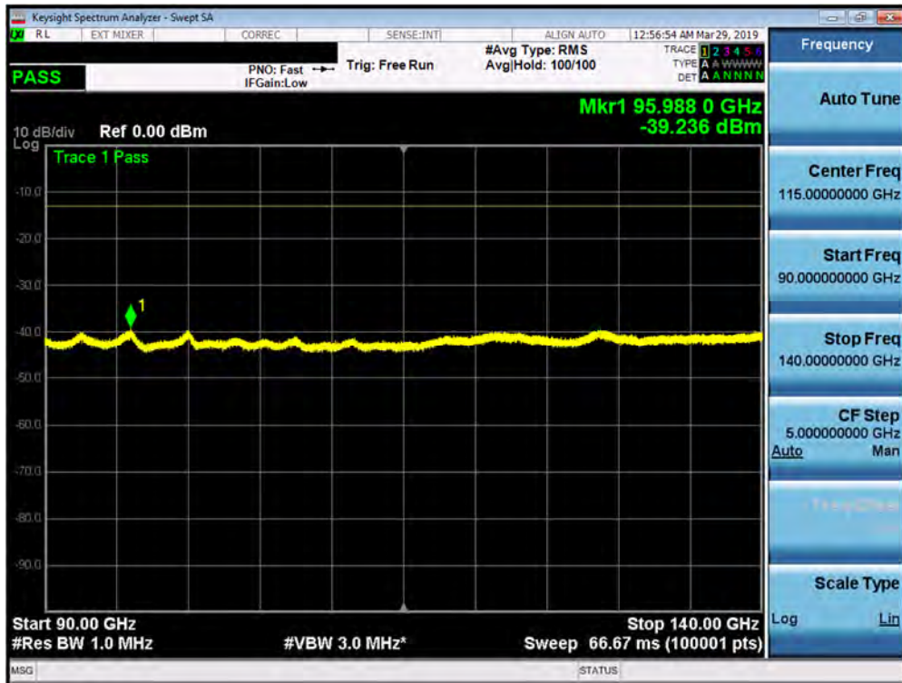
Plot 7-76. J Dipole Radiated Spurious Plot 90-140 GHz (1CC QPSK High Channel V Beam)
