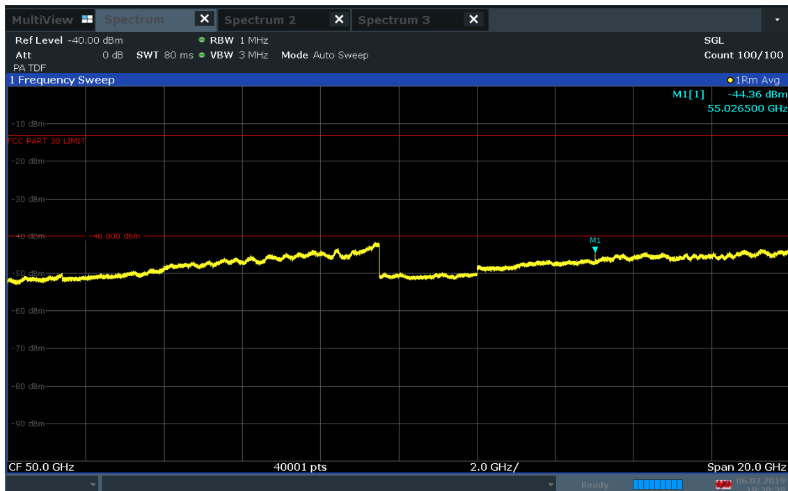
Plot 7-170. L Patch Radiated Spurious Plot 40-60 GHz (1CC QPSK Low Channel V Beam)
