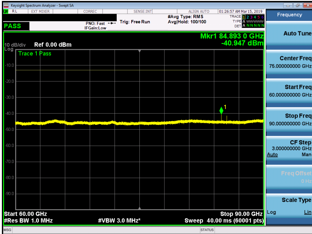
Plot 7-178. L Patch Radiated Spurious Plot 60-90 GHz (1CC QPSK High Channel V Beam)
