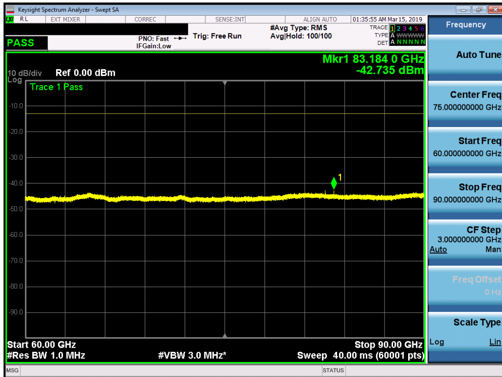
Plot 7-173. L Patch Radiated Spurious Plot 60-90 GHz (1CC QPSK Low Channel H Beam)
