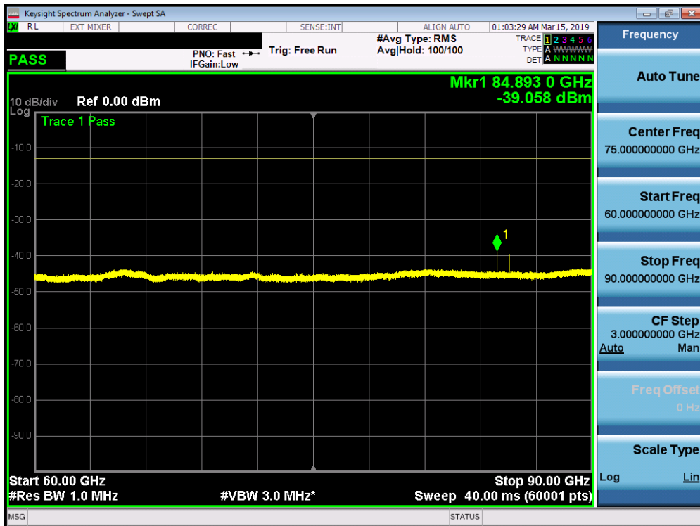
Plot 7-144. K Patch Radiated Spurious Plot 60-90 GHz (1CC QPSK High Channel V Beam)
