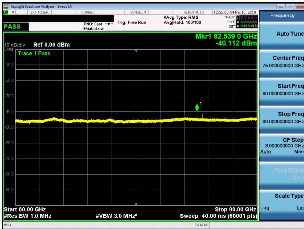
Plot 7-142. K Patch Radiated Spurious Plot 60-90 GHz (1CC QPSK Low Channel V Beam)
