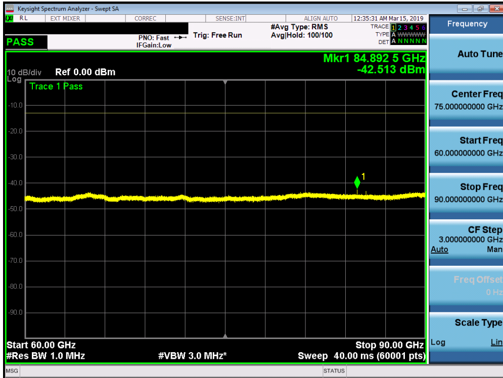
Plot 7-141. K Patch Radiated Spurious Plot 60-90 GHz (1CC QPSK High Channel H Beam)
