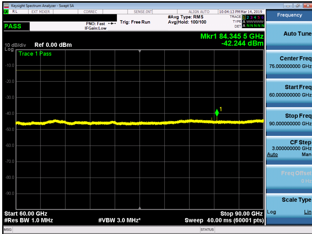
Plot 7-75. J Dipole Radiated Spurious Plot 60-90 GHz (1CC 16QAM Mid Channel V Beam)
