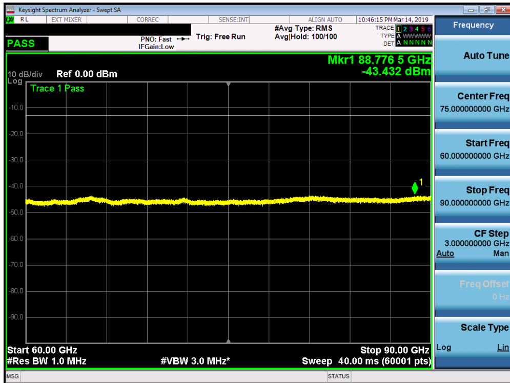
Plot 7-105. J Patch Radiated Spurious Plot 60-90 GHz (1CC 16QAM Low Channel H Beam)
