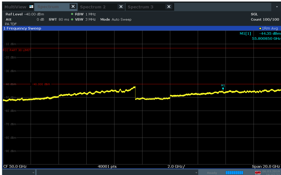
Plot 7-66. J Dipole Radiated Spurious Plot 40-60 GHz (1CC 16QAM Mid Channel H Beam)
