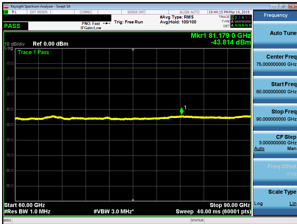
Plot 7-106. J Patch Radiated Spurious Plot 60-90 GHz (1CC 16QAM Mid Channel H Beam)
