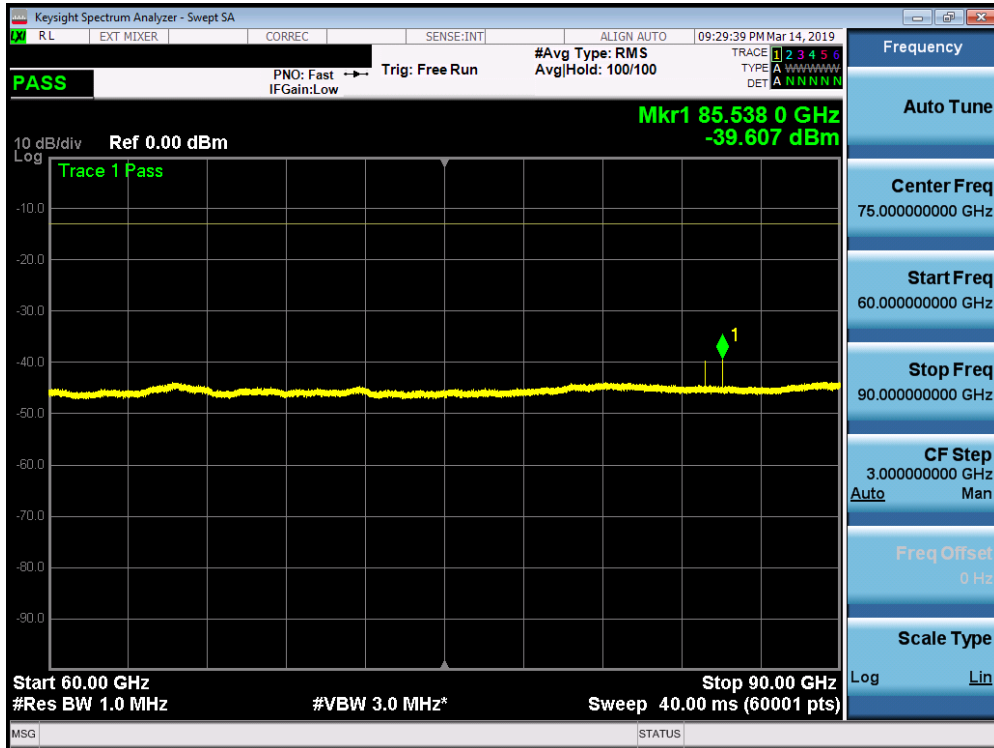
Plot 7-73. J Dipole Radiated Spurious Plot 60-90 GHz (1CC 16QAM High Channel H Beam)
