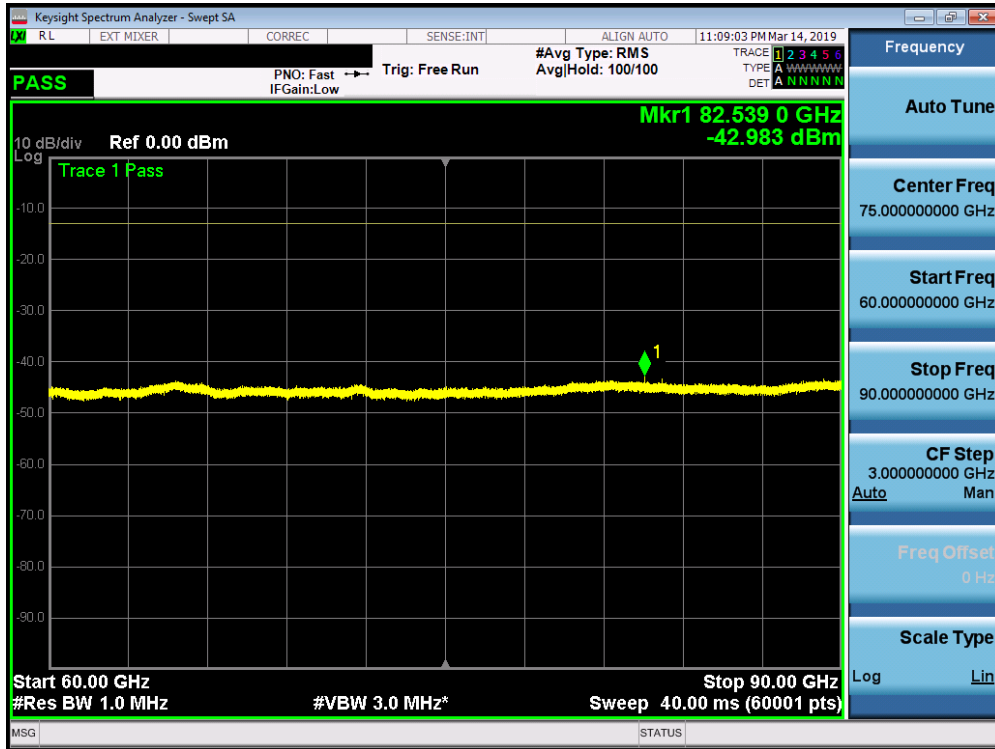
Plot 7-139. K Patch Radiated Spurious Plot 60-90 GHz (1CC QPSK Low Channel H Beam)
