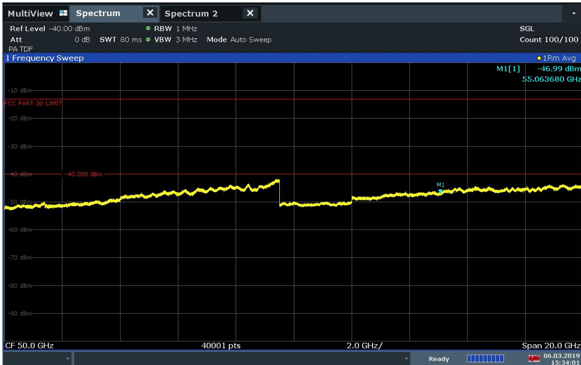
Plot 7-101. J Patch Radiated Spurious Plot 40-60 GHz (1CC 16QAM High Channel H Beam)
