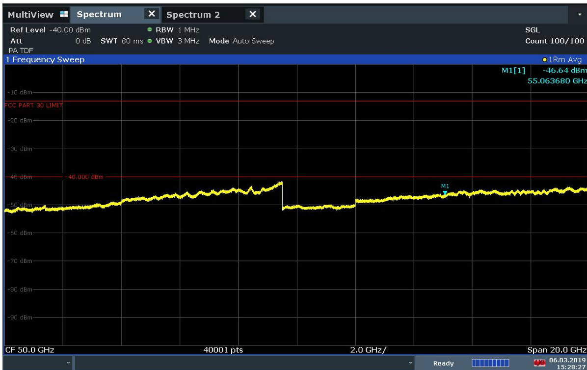
Plot 7-102. J Patch Radiated Spurious Plot 40-60 GHz (1CC 16QAM Low Channel V Beam)
