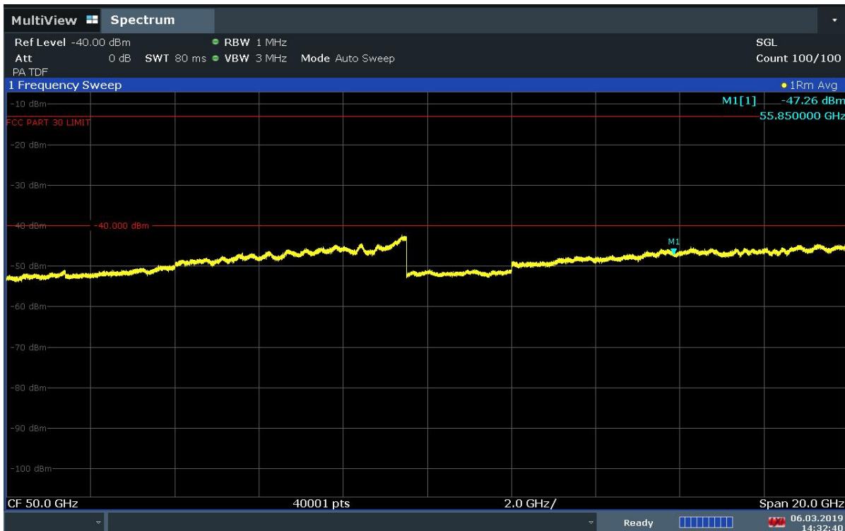
Plot 7-100. J Patch Radiated Spurious Plot 40-60 GHz (1CC 16QAM Mid Channel H Beam)
