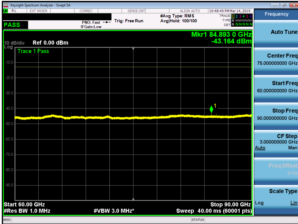
Plot 7-107. J Patch Radiated Spurious Plot 60-90 GHz (1CC 16QAM High Channel H Beam)
