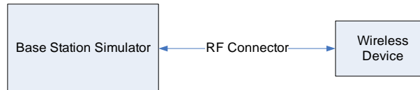
Figure 9-4 Power Measurement Setup
