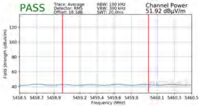
Plot 7-314. Radiated Lower Band Edge Plot SISO ANT1 (Average – UNII Band 2C)
