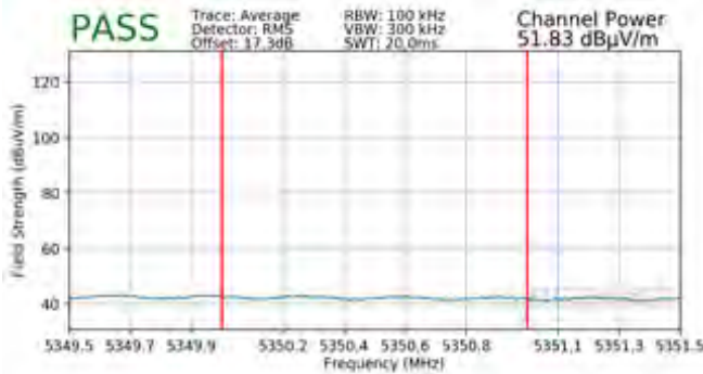
Plot 7-321. Radiated Upper Band Edge Plot SISO ANT2 (Average – UNII Band 2A)
