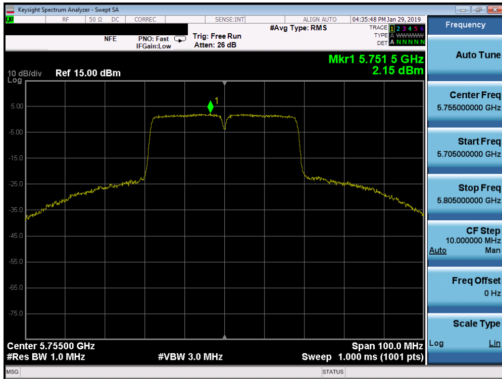
Plot 7-193. Power Spectral Density Plot SISO ANT1 (40MHz BW 802.11n (UNII Band 3) – Ch. 151)
