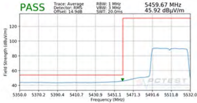
Plot 7-347. Radiated Lower Band Edge Plot SISO ANT2 (Average – UNII Band 2C – 484 Tones)
