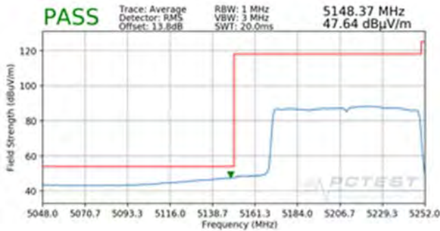
Plot 7-352. Radiated Lower Band Edge Plot SISO ANT2 (Average – UNII Band 1 – 996 Tones)
