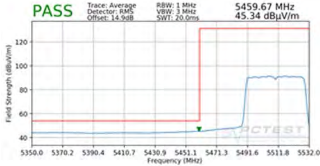
Plot 7-374. Radiated Lower Band Edge Plot MIMO (Average – UNII Band 2C – 484 Tones)
