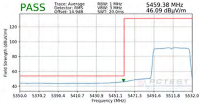
Plot 7-320. Radiated Lower Band Edge Plot SISO ANT1 (Average – UNII Band 2C – 484 Tones)
