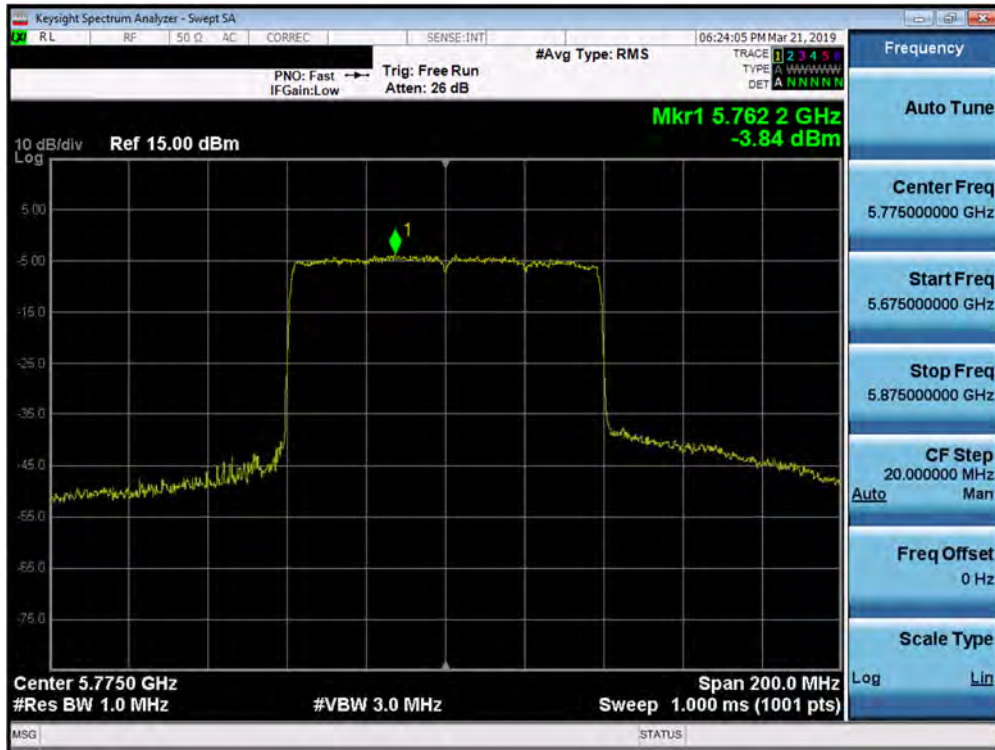
Plot 7-216. Power Spectral Density Plot SISO ANT2 (80MHz BW 802.11ax – Full Tones (UNII Band 3) – Ch. 155)
