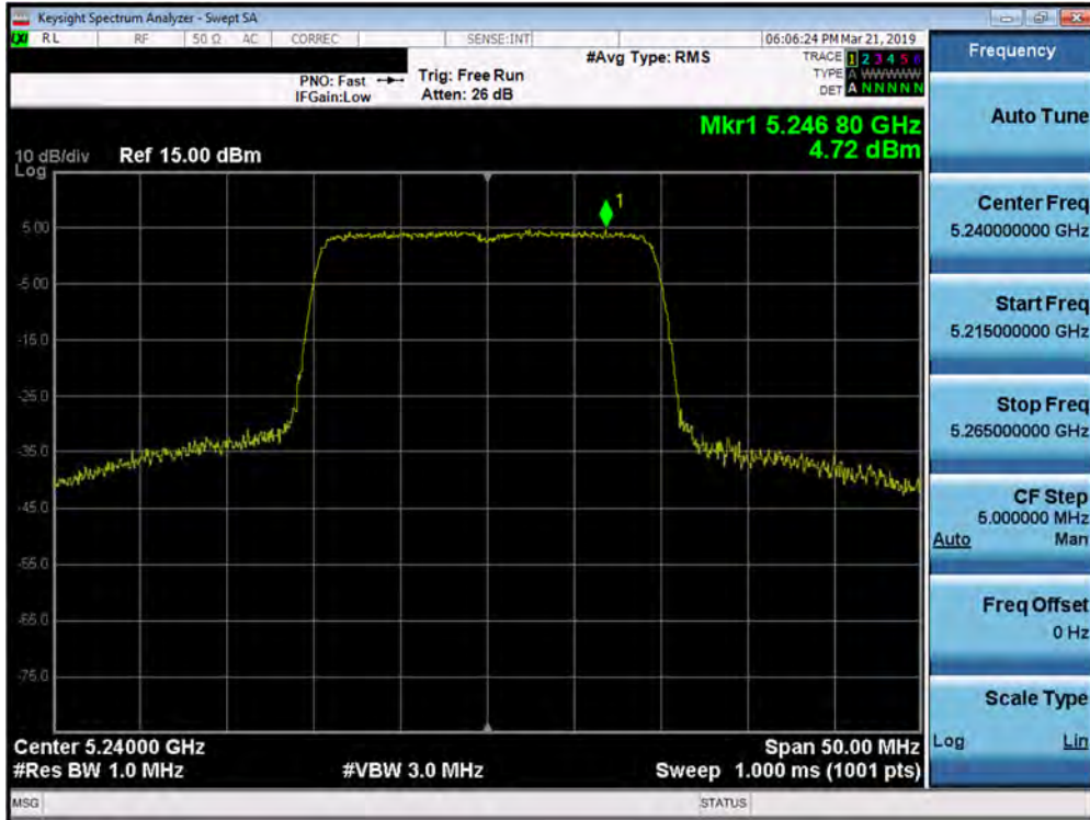
Plot 7-192. Power Spectral Density Plot SISO ANT2 (20MHz BW 802.11ax – Full Tones (UNII Band 1) – Ch. 48)
