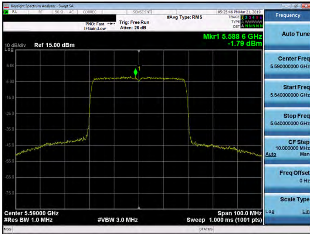
Plot 7-152. Power Spectral Density Plot SISO ANT1 (40MHz BW 802.11ax – Full Tones (UNII Band 2C) – Ch. 118)
