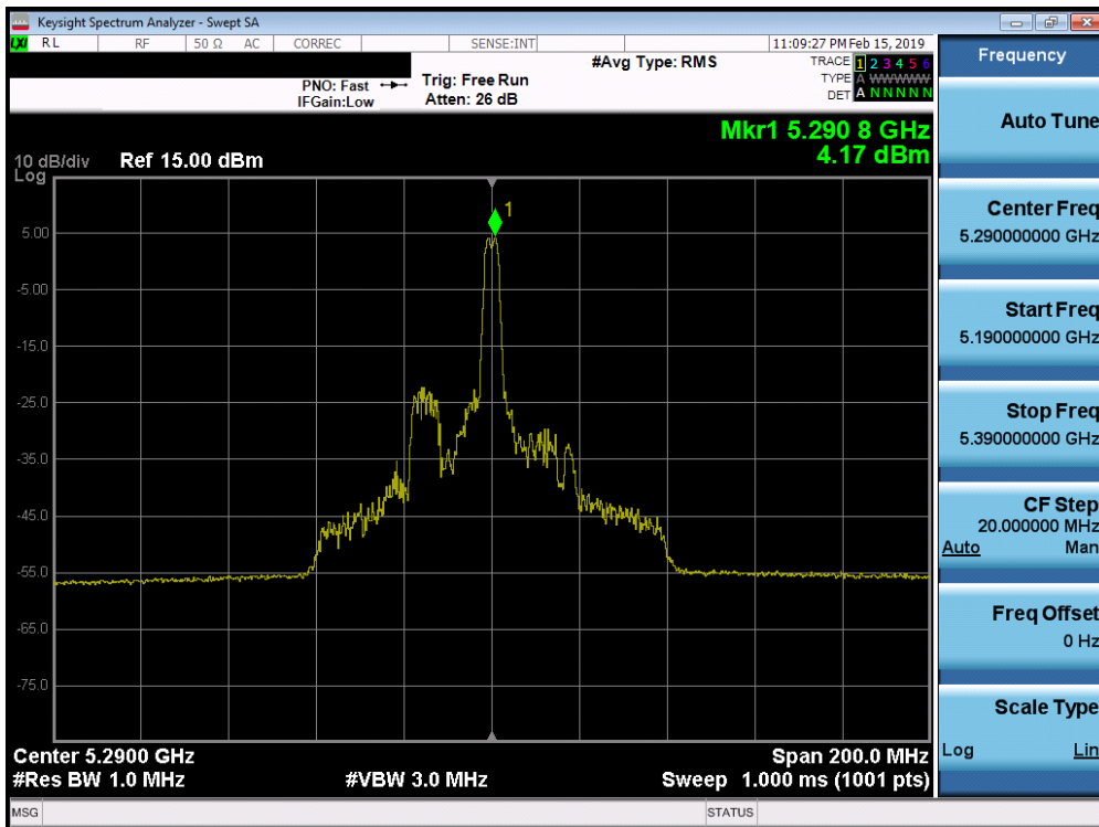
Plot 7-228. Power Spectral Density Plot MIMO ANT1 (80MHz BW 802.11ax – 26 Tones (UNII Band 2A) – Ch. 58)
