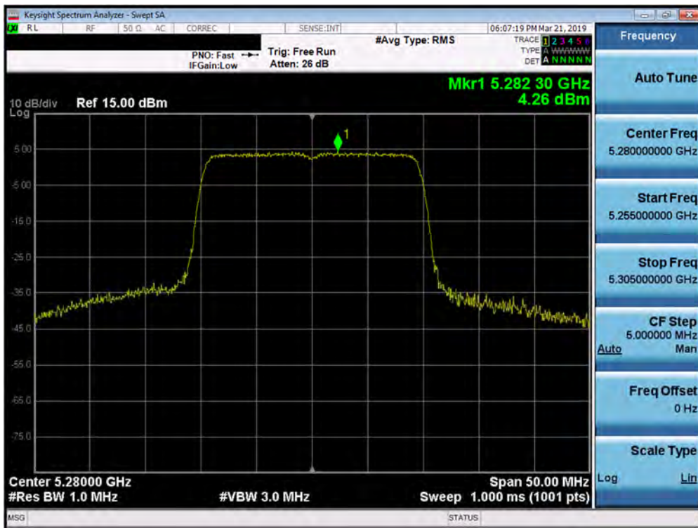
Plot 7-197. Power Spectral Density Plot SISO ANT2 (20MHz BW 802.11ax – Full Tones (UNII Band 2A) – Ch. 56)
