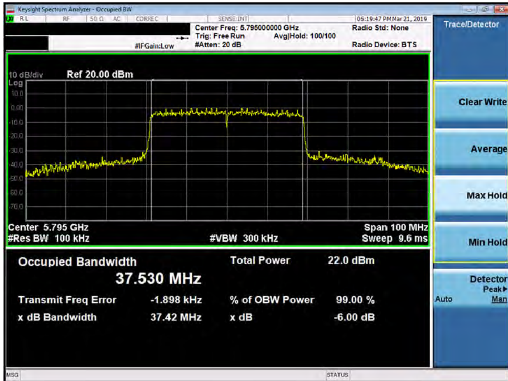
Plot 7-107. 6dB Bandwidth Plot SISO ANT2 (40MHz BW 802.11ax – Full Tones (UNII Band 3) – Ch. 159)
