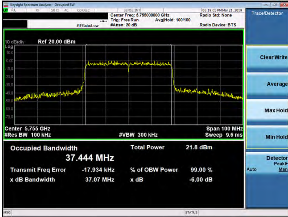
Plot 7-106. 6dB Bandwidth Plot SISO ANT2 (40MHz BW 802.11ax – Full Tones (UNII Band 3) – Ch. 151)
