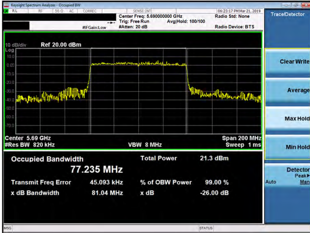
Plot 7-84. 26dB Bandwidth Plot SISO ANT2 (80MHz BW 802.11ax – Full Tones (UNII Band 2C) – Ch. 138)
