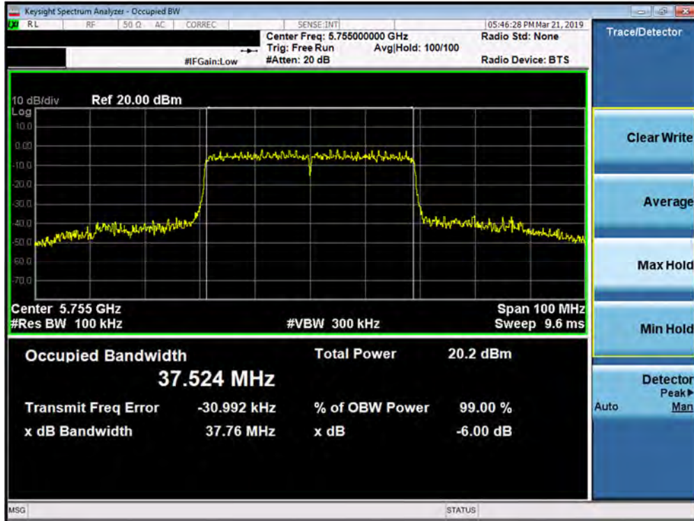
Plot 7-94. 6dB Bandwidth Plot SISO ANT1 (40MHz BW 802.11ax – Full Tones (UNII Band 3) – Ch. 151)
