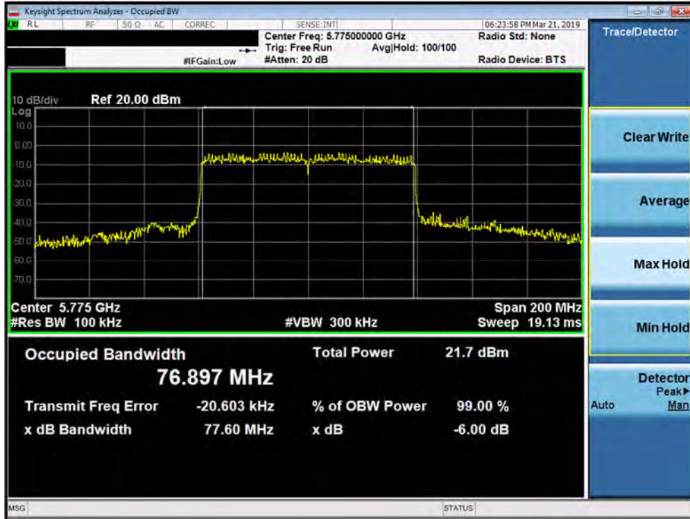
Plot 7-108. 6dB Bandwidth Plot SISO ANT2 (80MHz BW 802.11ax – Full Tones (UNII Band 3) – Ch. 155)
