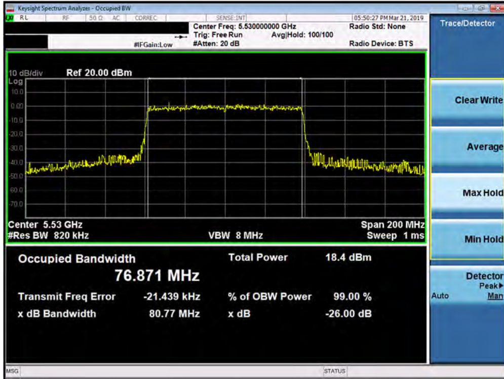
Plot 7-40. 26dB Bandwidth Plot SISO ANT1 (80MHz BW 802.11ax – Full Tones (UNII Band 2C) – Ch. 106)
