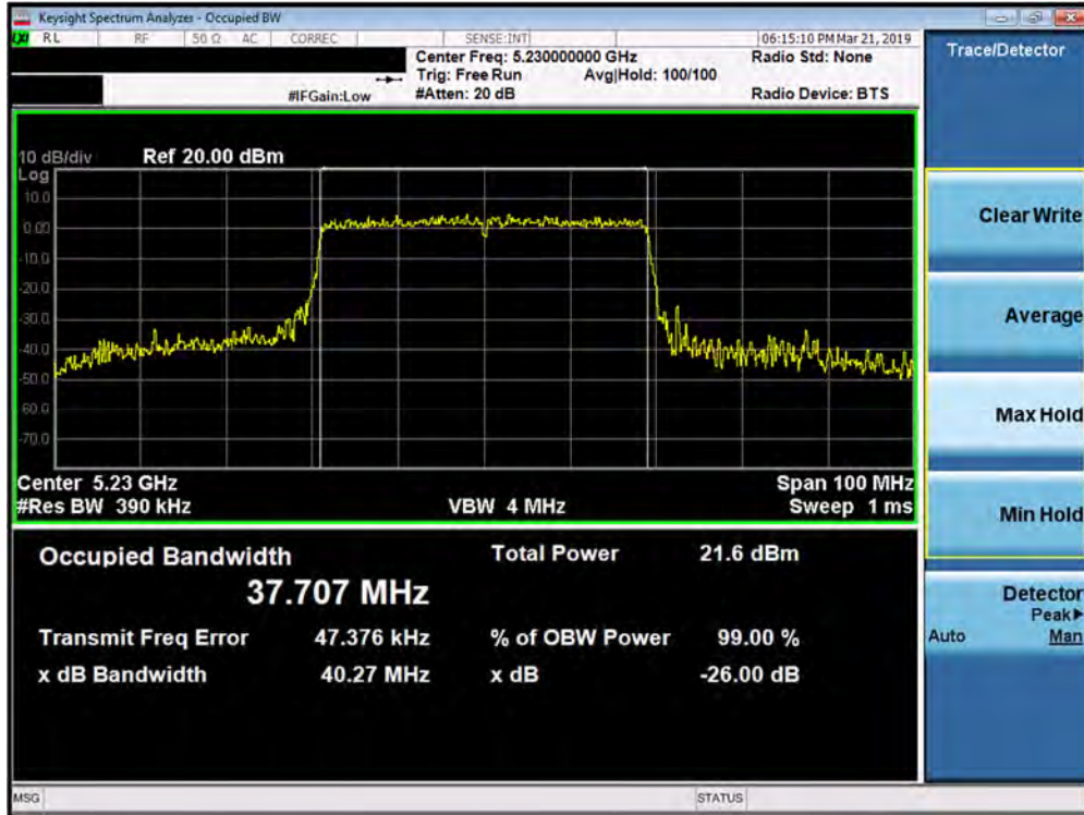
Plot 7-68. 26dB Bandwidth Plot SISO ANT2 (40MHz BW 802.11ax – Full Tones (UNII Band 1) – Ch. 46)
