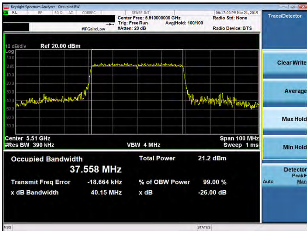
Plot 7-79. 26dB Bandwidth Plot SISO ANT2 (40MHz BW 802.11ax – Full Tones (UNII Band 2C) – Ch. 102)
