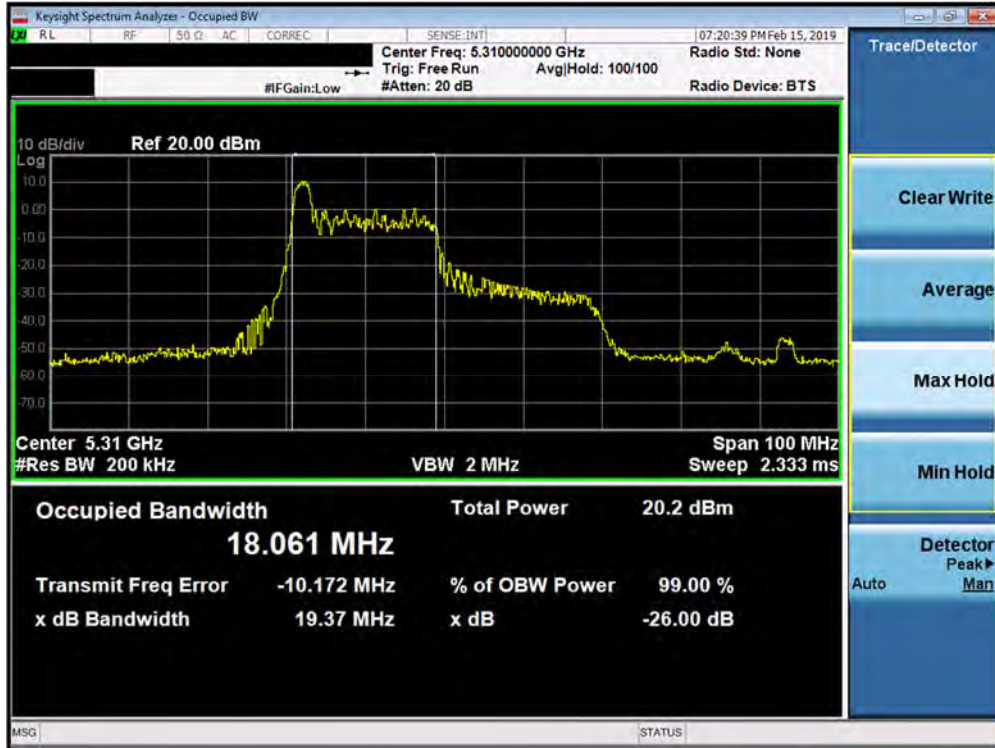
Plot 7-53. 26dB Bandwidth Plot SISO ANT2 (40MHz BW 802.11ax – 26 Tones (UNII Band 2A) – Ch. 62)
