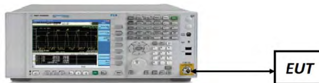
Figure 7-1. Test Instrument & Measurement Setup
