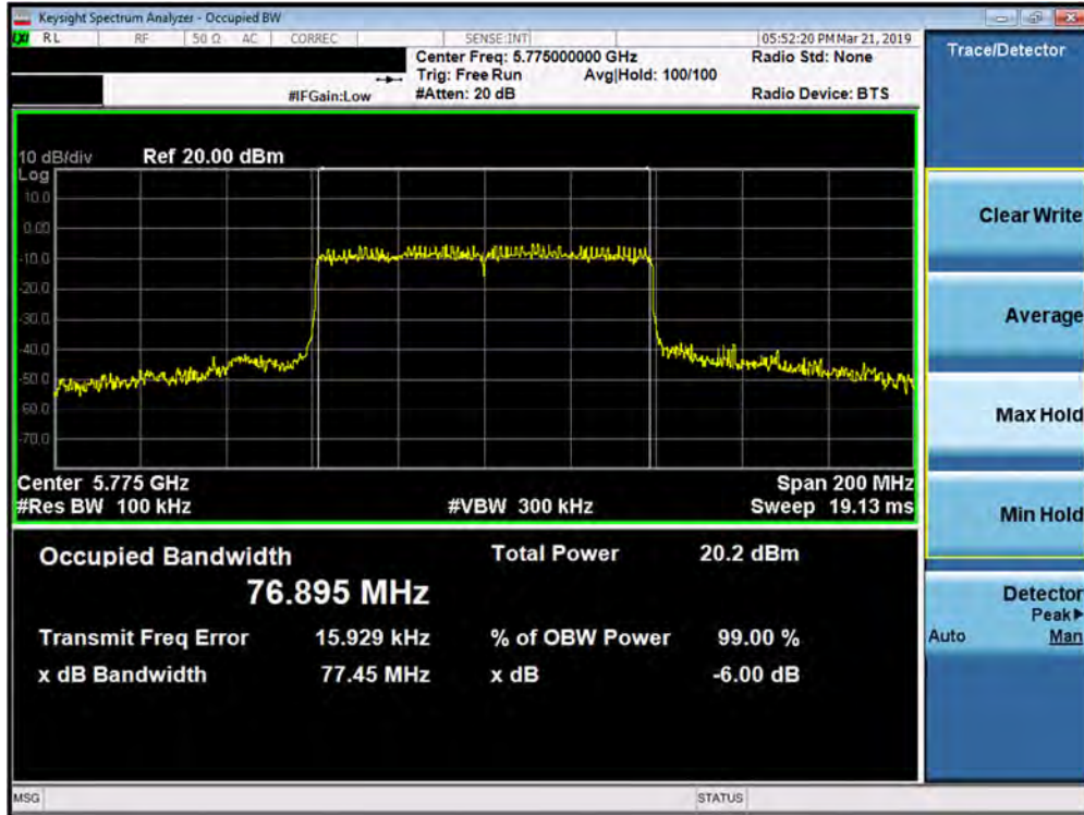
Plot 7-96. 6dB Bandwidth Plot SISO ANT1 (80MHz BW 802.11ax – Full Tones (UNII Band 3) – Ch. 155)
