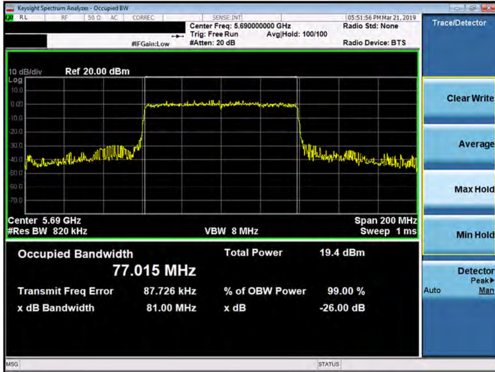
Plot 7-42. 26dB Bandwidth Plot SISO ANT1 (80MHz BW 802.11ax – Full Tones (UNII Band 2C) – Ch. 138)
