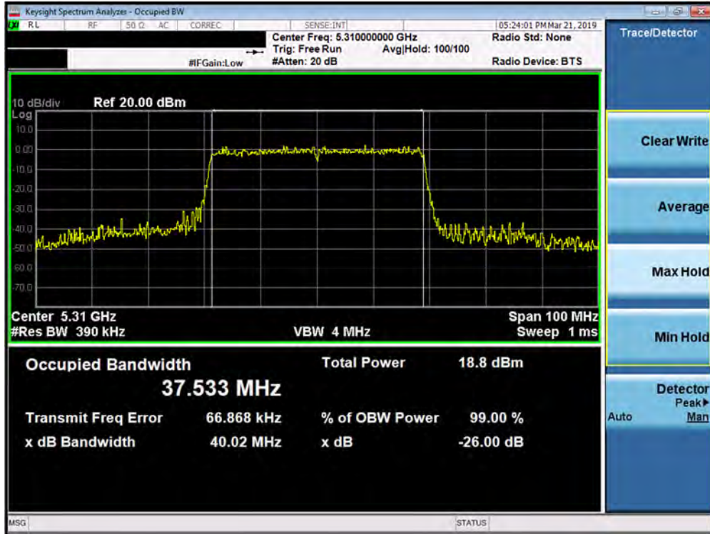
Plot 7-32. 26dB Bandwidth Plot SISO ANT1 (40MHz BW 802.11ax – Full Tones (UNII Band 2A) – Ch. 62)
