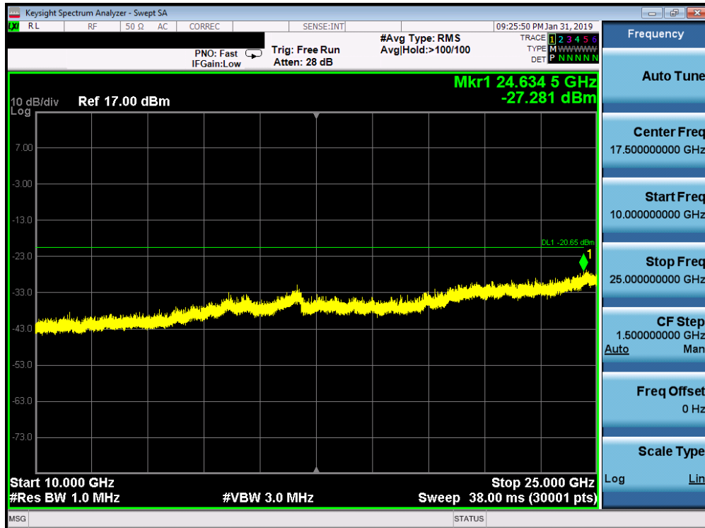
Plot 7-68. Conducted Spurious Plot SISO ANT1 (802.11b – Ch. 6)
