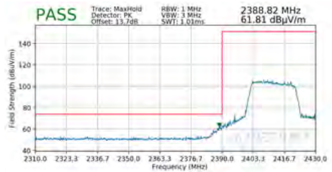
Plot 7-92. Radiated Restricted Band Edge Measurement SISO ANT1 with WCP (Peak – 242 Tones)
