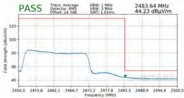
Plot 7-109. Radiated Restricted Band Edge Measurement SISO ANT2 with WCP (Average – 242 Tones)
