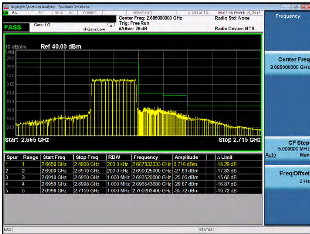
Plot 7-304. Upper ACP Plot (Band 41 PC3 - 10.0MHz QPSK - Full RB Configuration)
