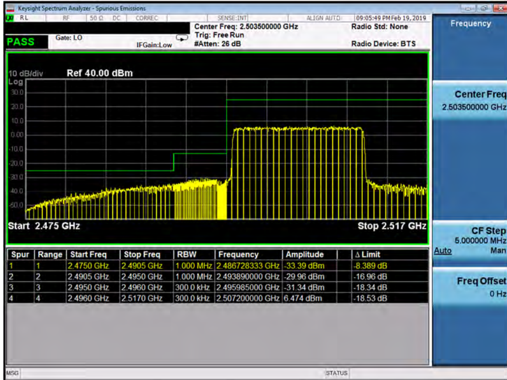
Plot 7-305. Lower ACP Plot (Band 41 PC3 - 15.0MHz QPSK - Full RB Configuration)
