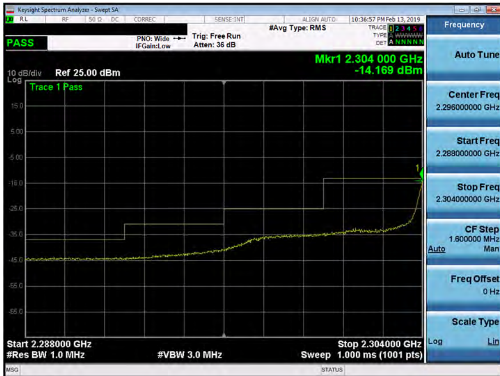
Plot 7-286. Lower Extended Band Edge Plot (Band 30 - 5.0MHz QPSK - Full RB Configuration)
