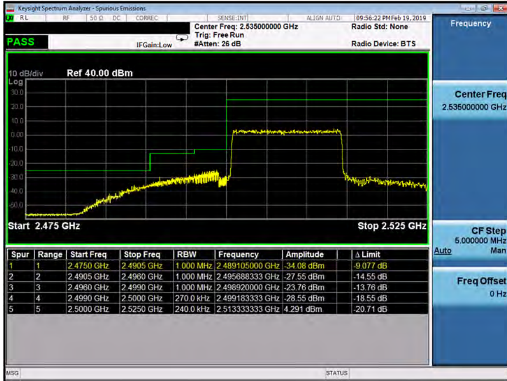
Plot 7-297. Lower ACP Plot (Band 7 - 15.0MHz QPSK - Full RB Configuration)
