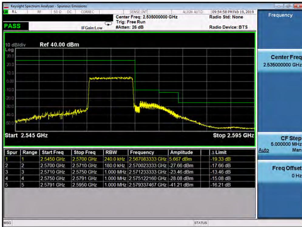
Plot 7-296. Upper ACP Plot (Band 7 - 10.0MHz QPSK - Full RB Configuration)
