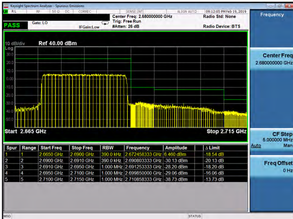
Plot 7-308. Upper ACP Plot (Band 41 PC3 - 20.0MHz QPSK - Full RB Configuration)
