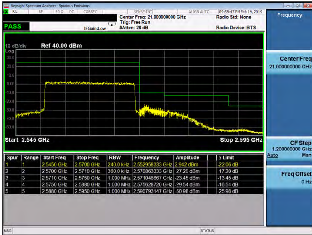
Plot 7-300. Upper ACP Plot (Band 7 - 20.0MHz QPSK - Full RB Configuration)
