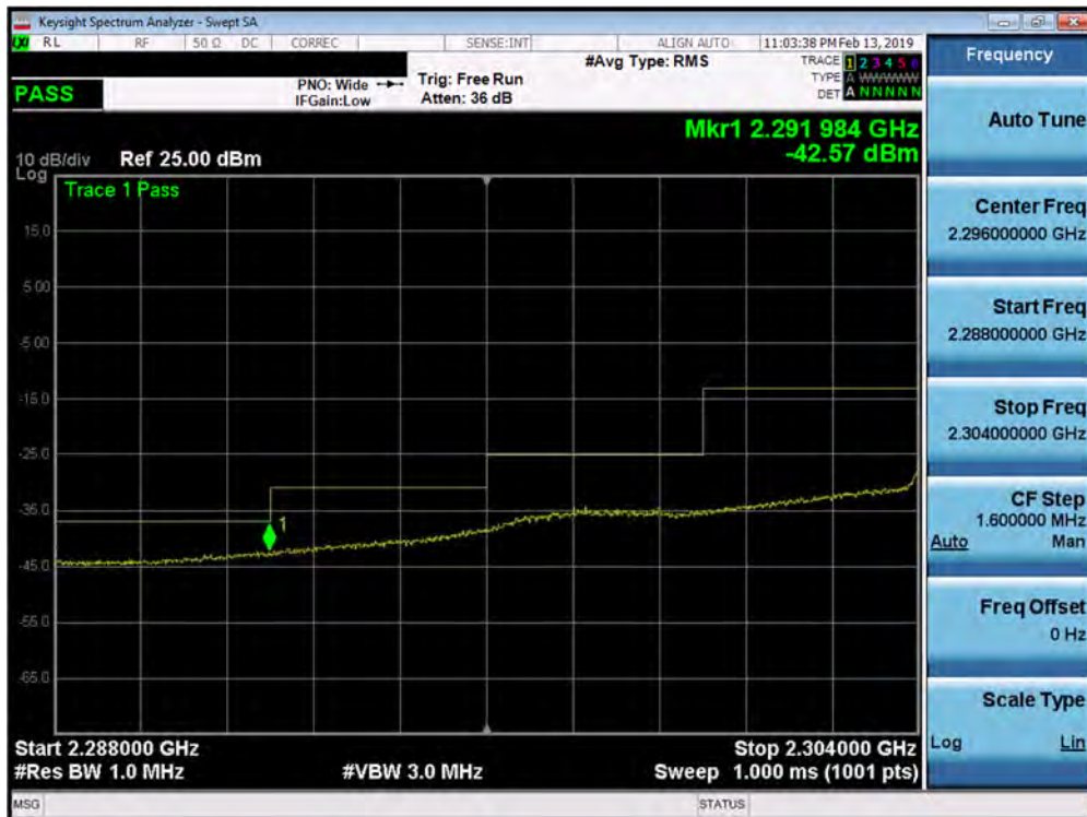
Plot 7-290. Lower Extended Band Edge Plot (Band 30 - 10.0MHz QPSK - Full RB Configuration)
