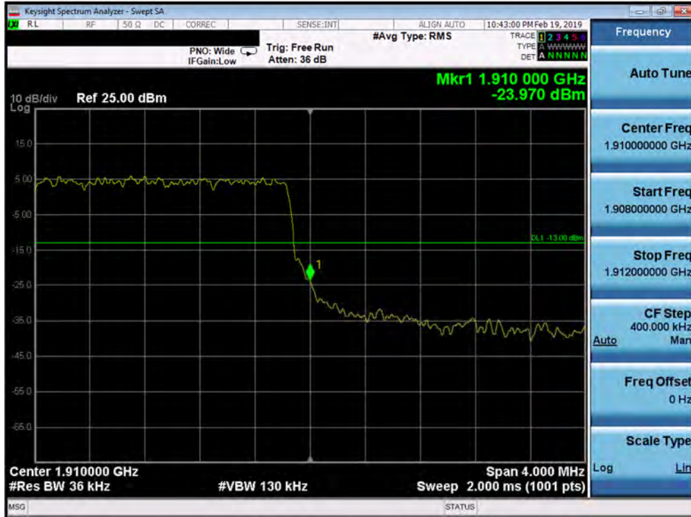
Plot 7-267. Upper Band Edge Plot (Band 2 - 3.0MHz QPSK - Full RB Configuration)
