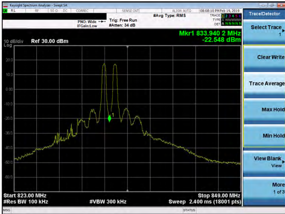
Plot 7-366. Conducted Spurious Plot (Band 5 – 10.0MHz QPSK – PCC 1/49 SCC 1/0 – Mid Channel)
