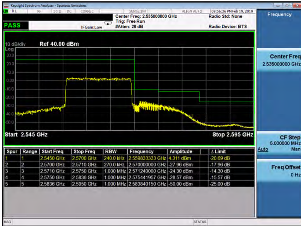
Plot 7-298. Upper ACP Plot (Band 7 - 15.0MHz QPSK - Full RB Configuration)
