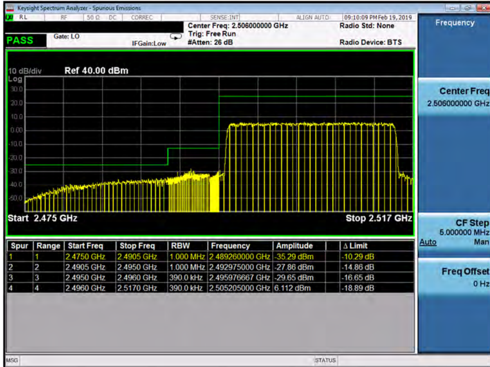
Plot 7-307. Lower ACP Plot (Band 41 PC3 - 20.0MHz QPSK - Full RB Configuration)
