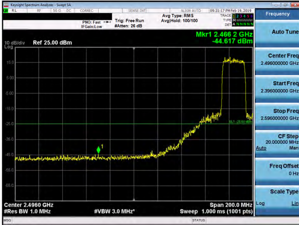
Plot 7-315. Lower ACP Plot (Band 38 - 20.0MHz QPSK - Full RB Configuration)
