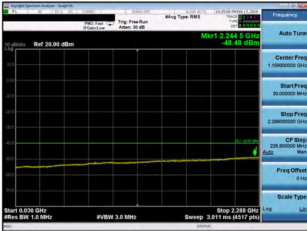
Plot 7-172. Conducted Spurious Plot (Band 30 - 5.0MHz QPSK - RB Size 1, RB Offset 0 - Low Channel)
