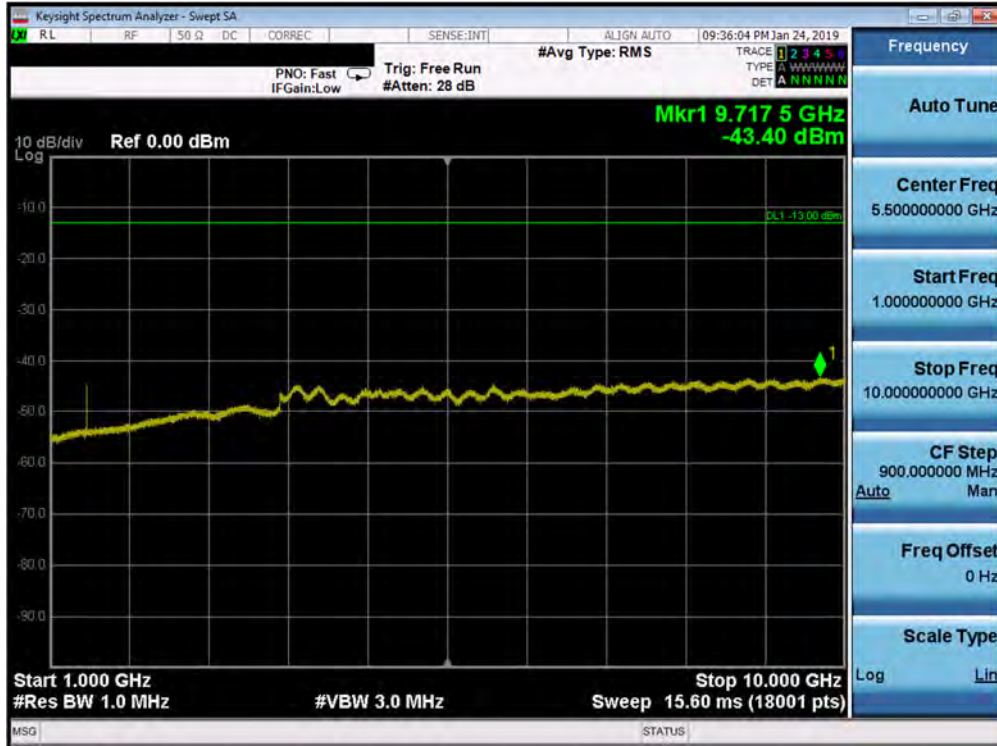
Plot 7-141. Conducted Spurious Plot (Band 12 - 10.0MHz QPSK - RB Size 1, RB Offset 0 - High Channel)
