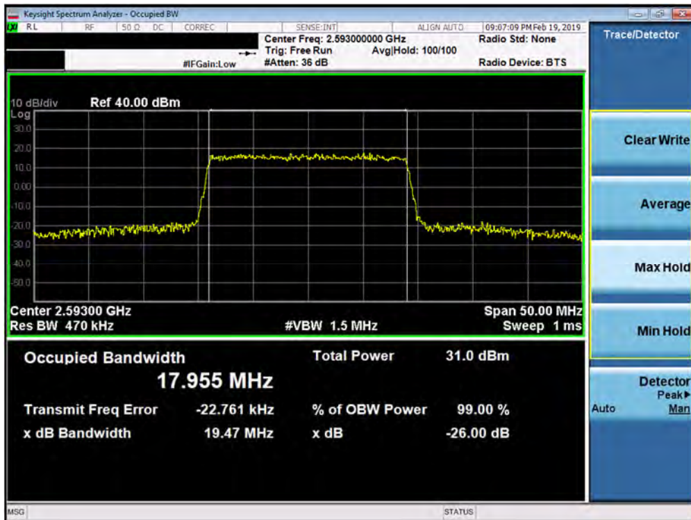
Plot 7-130. Occupied Bandwidth Plot (Band 41 PC3 / Band 38 - 20.0MHz 16-QAM - Full RB Configuration)
