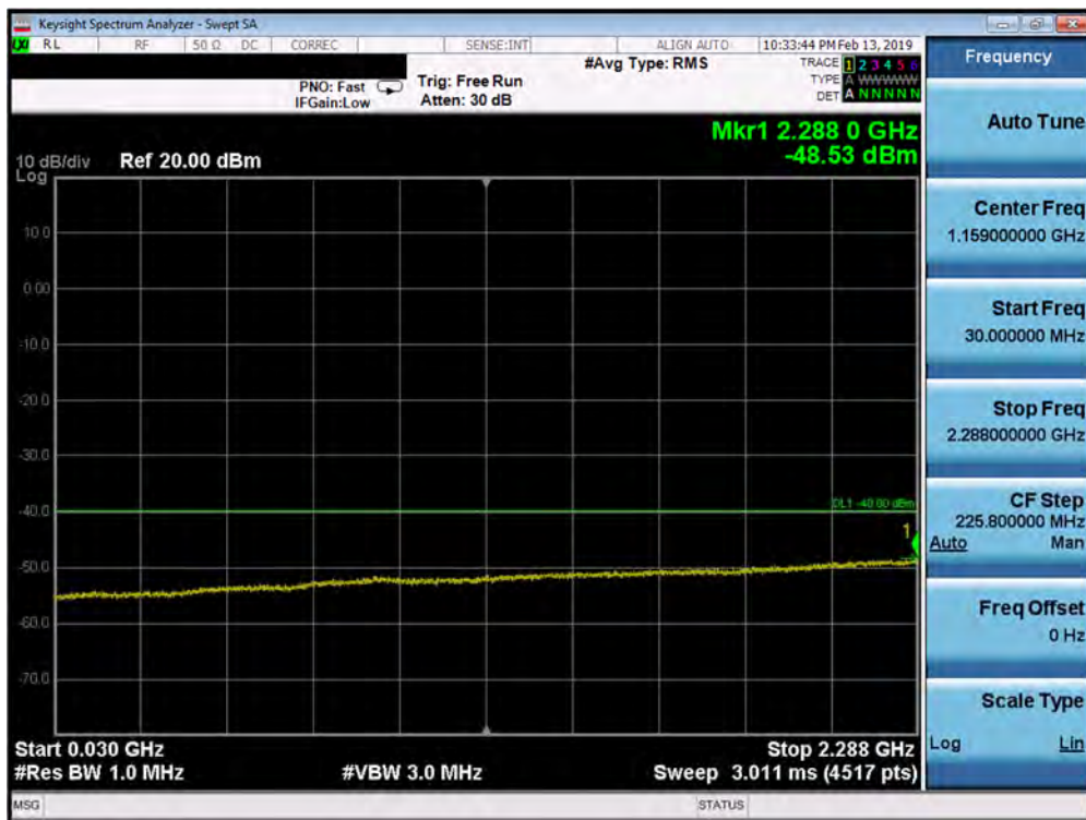
Plot 7-175. Conducted Spurious Plot (Band 30 - 5.0MHz QPSK - RB Size 1, RB Offset 0 - Mid Channel)
