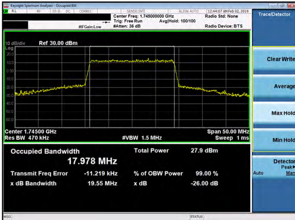
Plot 7-68. Occupied Bandwidth Plot (Band 66/4 - 20.0MHz 256-QAM - Full RB Configuration)
