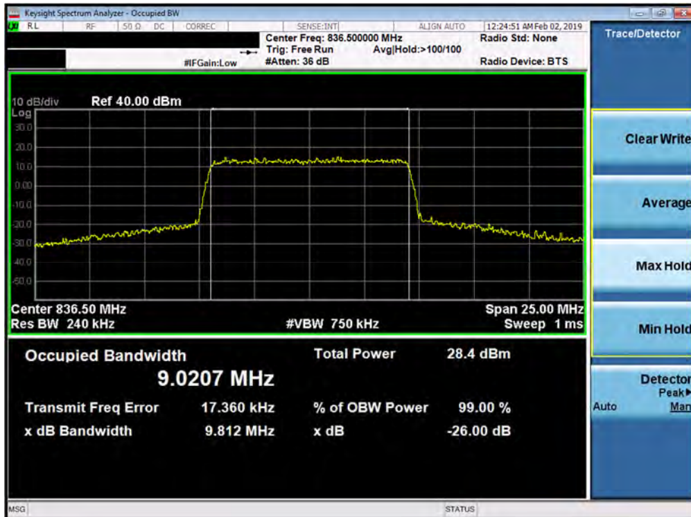
Plot 7-40. Occupied Bandwidth Plot (Band 26/5 - 10.0MHz 256-QAM - Full RB Configuration)
