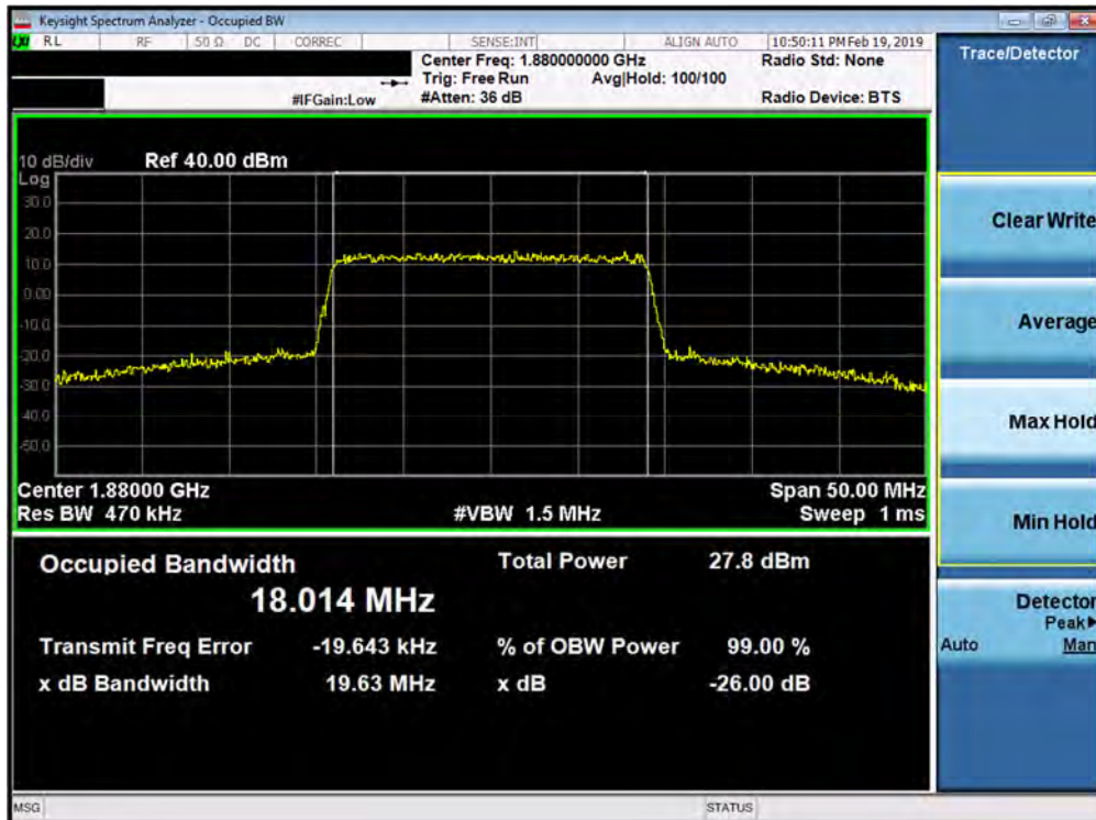
Plot 7-92. Occupied Bandwidth Plot (Band 2 - 20.0MHz 256-QAM - Full RB Configuration)
