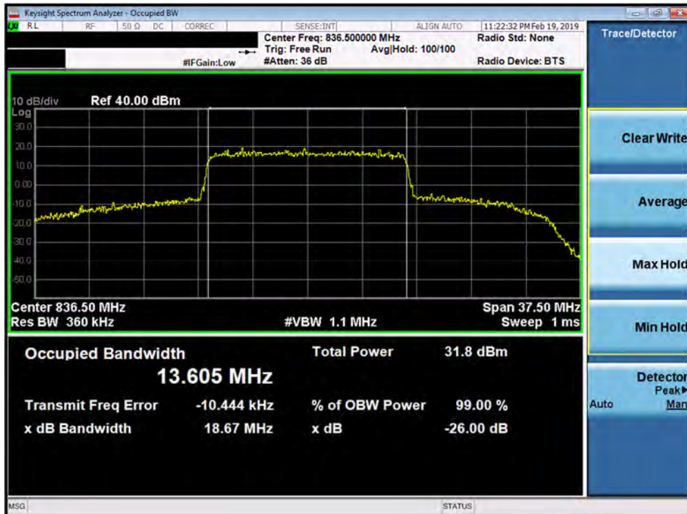
Plot 7-42. Occupied Bandwidth Plot (Band 26 - 15.0MHz 16-QAM - Full RB Configuration)
