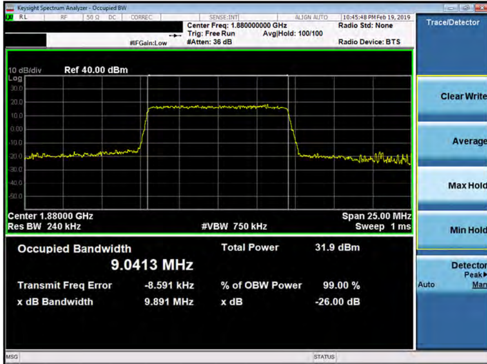
Plot 7-81. Occupied Bandwidth Plot (Band 2 - 10.0MHz QPSK - Full RB Configuration)
