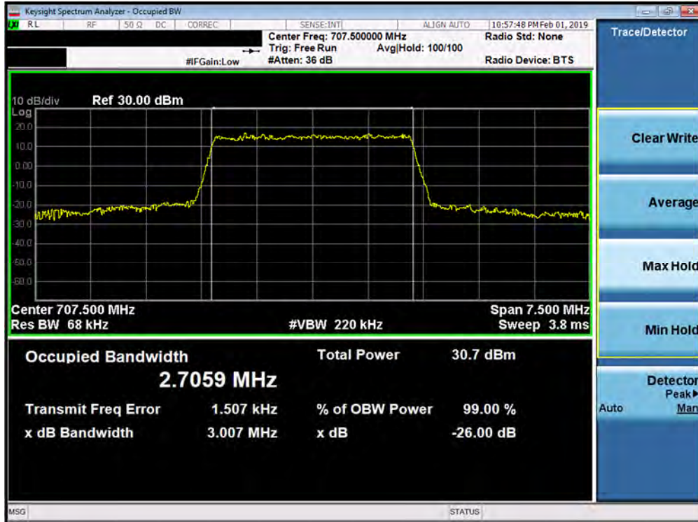
Plot 7-7. Occupied Bandwidth Plot (Band 12 - 3.0MHz 64-QAM - Full RB Configuration)
