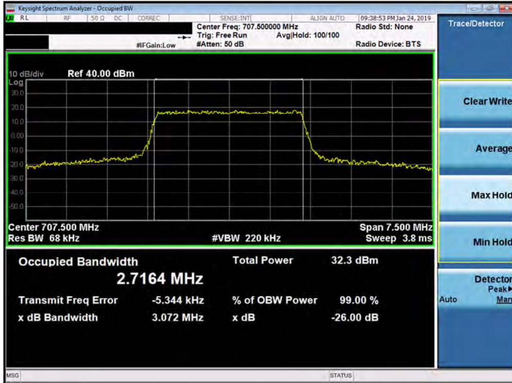
Plot 7-5. Occupied Bandwidth Plot (Band 12 - 3.0MHz QPSK - Full RB Configuration)
