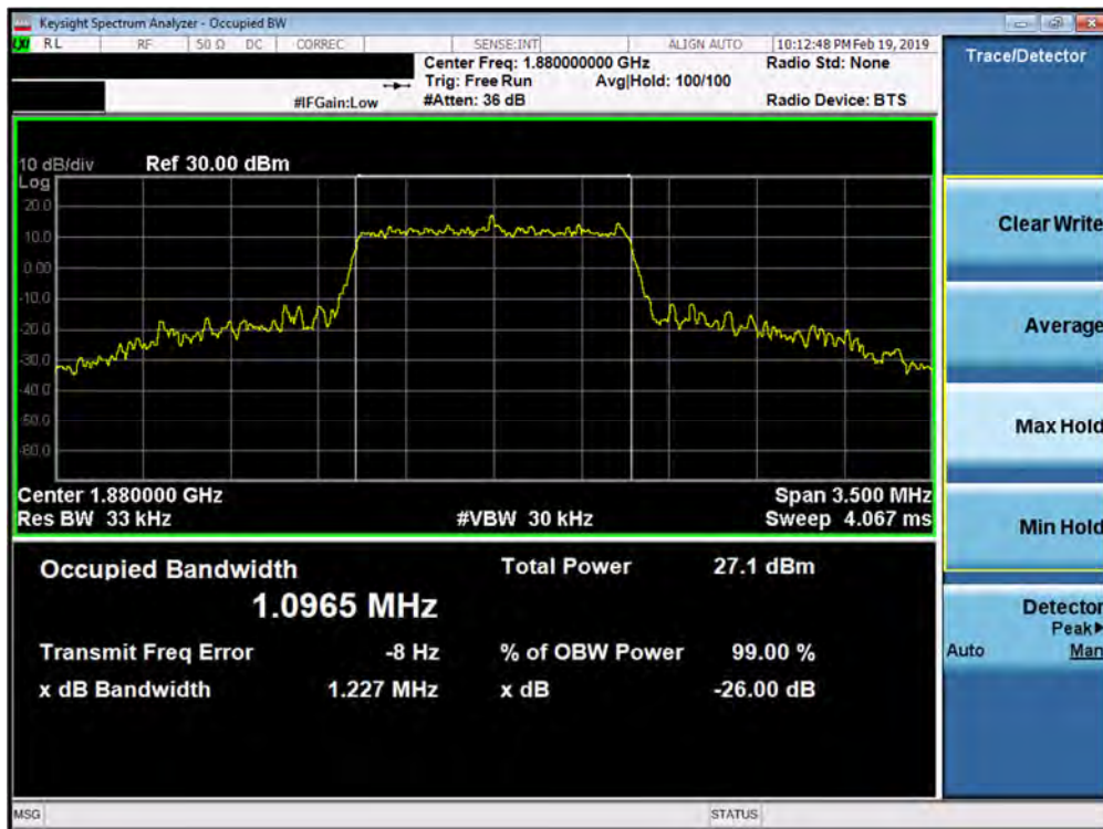
Plot 7-72. Occupied Bandwidth Plot (Band 2 - 1.4MHz 256-QAM - Full RB Configuration)
