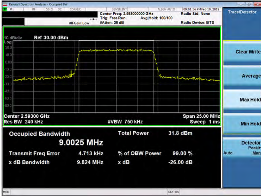
Plot 7-121. Occupied Bandwidth Plot (Band 41 PC3 / Band 38 - 10.0MHz QPSK - Full RB Configuration)
