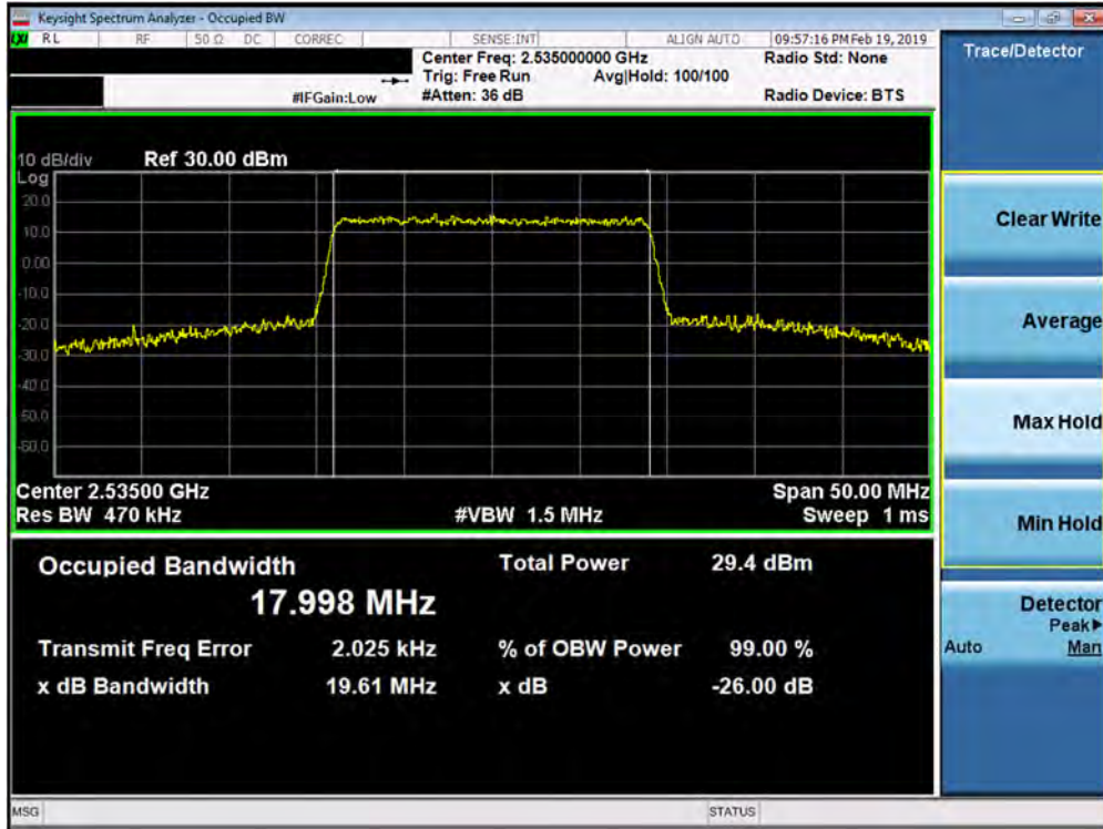
Plot 7-115. Occupied Bandwidth Plot (Band 7 - 20.0MHz 64-QAM - Full RB Configuration)
