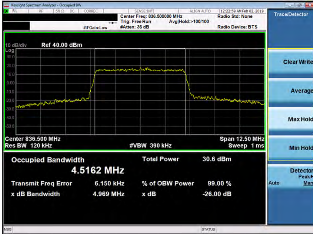
Plot 7-35. Occupied Bandwidth Plot (Band 26/5 - 5.0MHz 64-QAM - Full RB Configuration)
