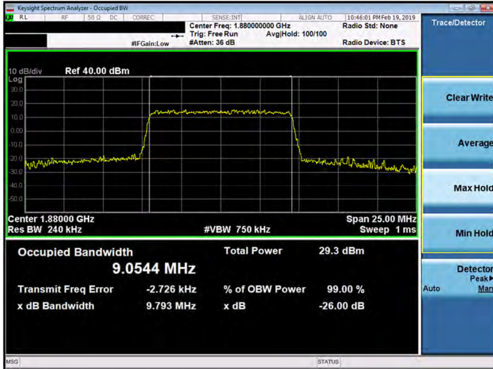
Plot 7-83. Occupied Bandwidth Plot (Band 2 - 10.0MHz 64-QAM - Full RB Configuration)
