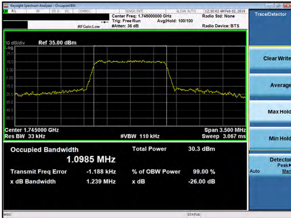
Plot 7-46. Occupied Bandwidth Plot (Band 66/4 - 1.4MHz 16-QAM - Full RB Configuration)
