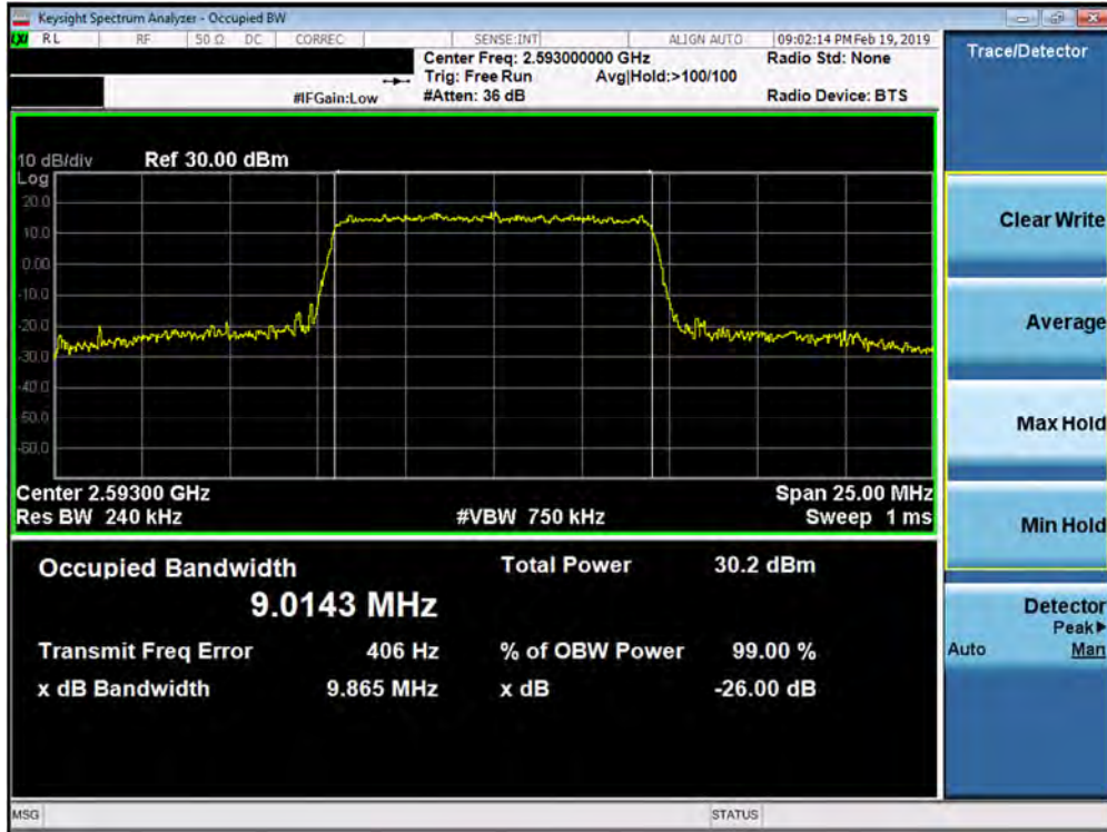
Plot 7-123. Occupied Bandwidth Plot (Band 41 PC3 / Band 38 - 10.0MHz 64-QAM - Full RB Configuration)
