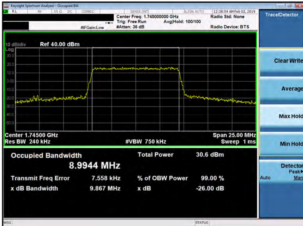
Plot 7-58. Occupied Bandwidth Plot (Band 66/4 - 10.0MHz 16-QAM - Full RB Configuration)
