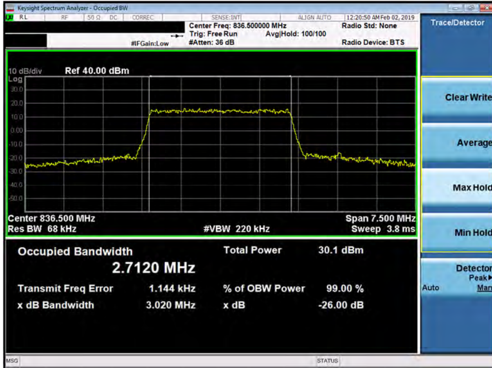
Plot 7-31. Occupied Bandwidth Plot (Band 26/5 - 3.0MHz 64-QAM - Full RB Configuration)
