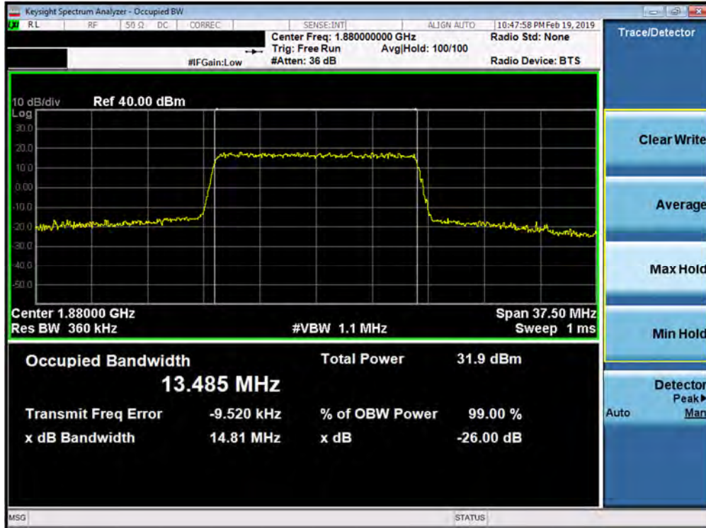
Plot 7-85. Occupied Bandwidth Plot (Band 2 - 15.0MHz QPSK - Full RB Configuration)
