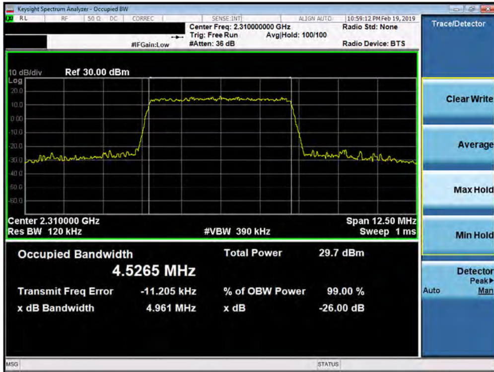
Plot 7-95. Occupied Bandwidth Plot (Band 30 – 5.0MHz 64-QAM - Full RB Configuration)
