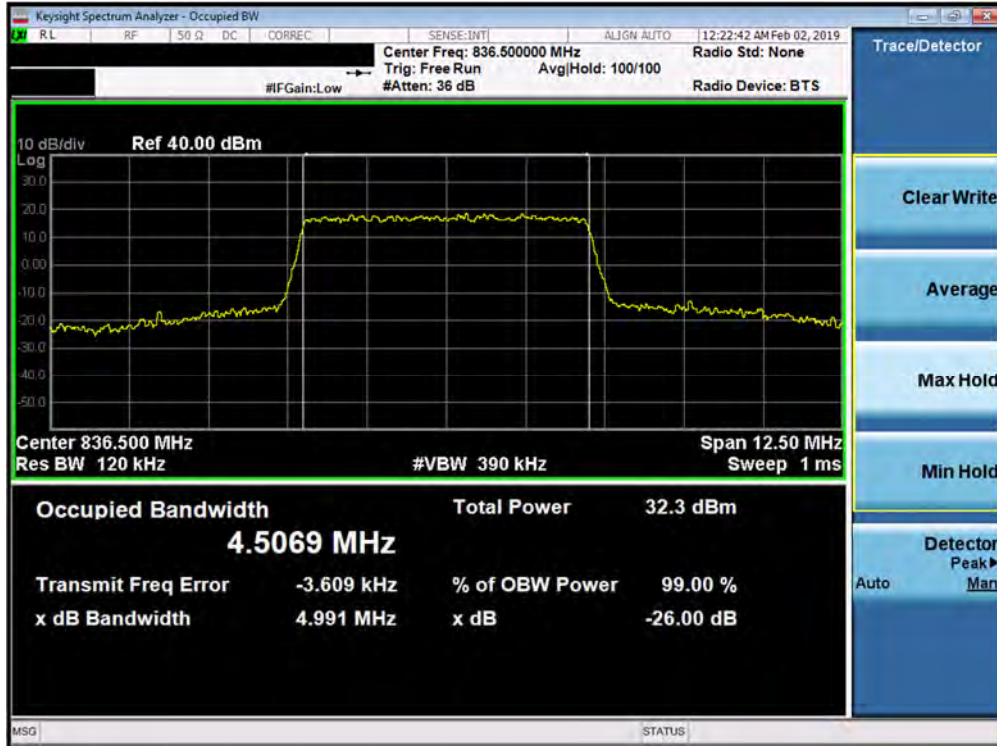
Plot 7-33. Occupied Bandwidth Plot (Band 26/5 - 5.0MHz QPSK - Full RB Configuration)
