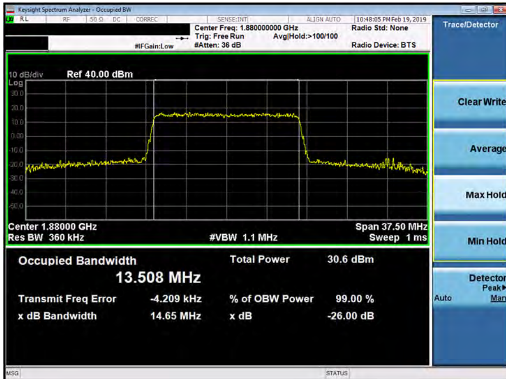
Plot 7-86. Occupied Bandwidth Plot (Band 2 - 15.0MHz 16-QAM - Full RB Configuration)
