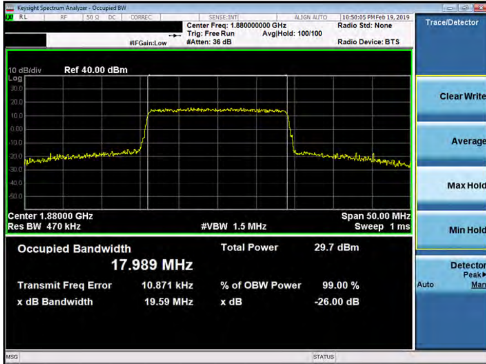
Plot 7-91. Occupied Bandwidth Plot (Band 2 - 20.0MHz 64-QAM - Full RB Configuration)
