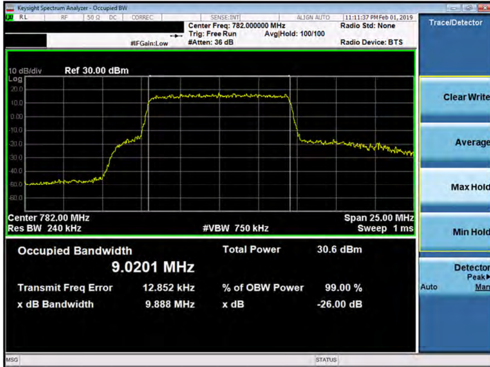
Plot 7-23. Occupied Bandwidth Plot (Band 13 - 10.0MHz 64-QAM - Full RB Configuration)
