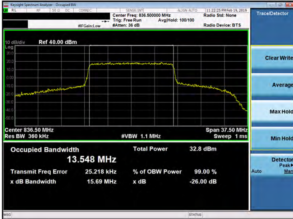
Plot 7-41. Occupied Bandwidth Plot (Band 26 - 15.0MHz QPSK - Full RB Configuration)
