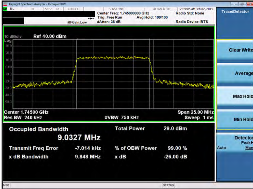
Plot 7-59. Occupied Bandwidth Plot (Band 66/4 - 10.0MHz 64-QAM - Full RB Configuration)
