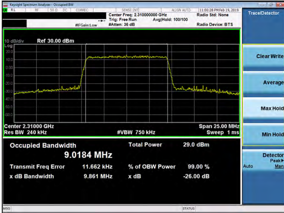
Plot 7-99. Occupied Bandwidth Plot (Band 30 - 10.0MHz 64-QAM - Full RB Configuration)
