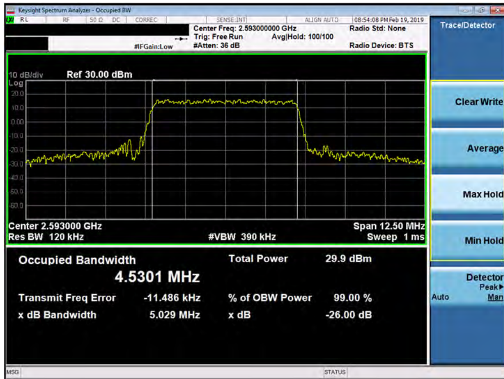
Plot 7-119. Occupied Bandwidth Plot (Band 41 PC3 / Band 38 – 5.0MHz 64-QAM - Full RB Configuration)
