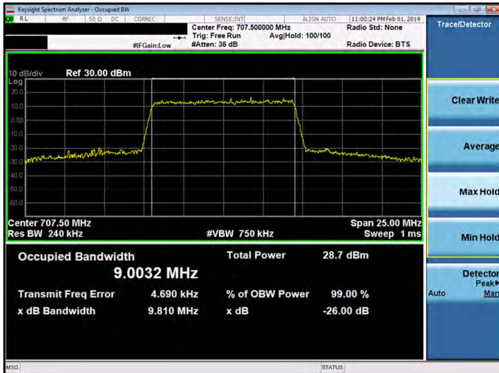
Plot 7-16. Occupied Bandwidth Plot (Band 12 - 10.0MHz 256-QAM - Full RB Configuration)
