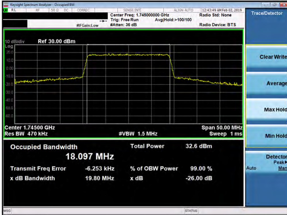
Plot 7-65. Occupied Bandwidth Plot (Band 66/4 - 20.0MHz QPSK - Full RB Configuration)
