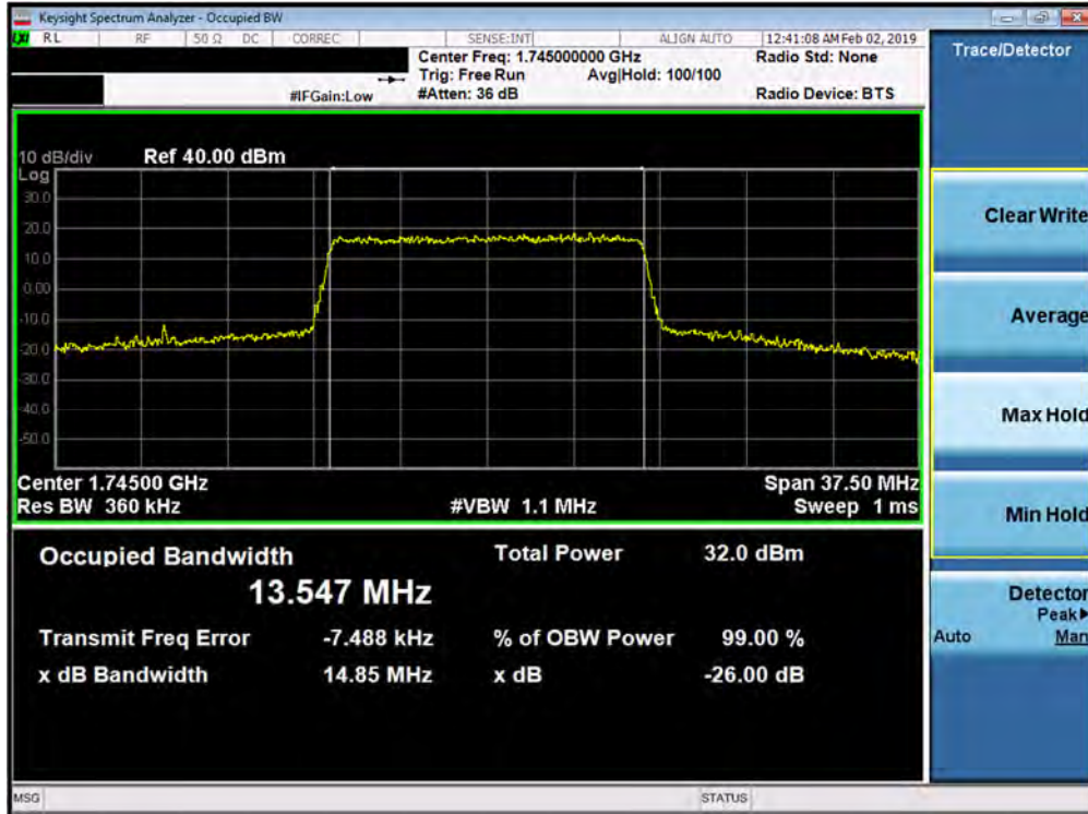
Plot 7-61. Occupied Bandwidth Plot (Band 66/4 - 15.0MHz QPSK - Full RB Configuration)
