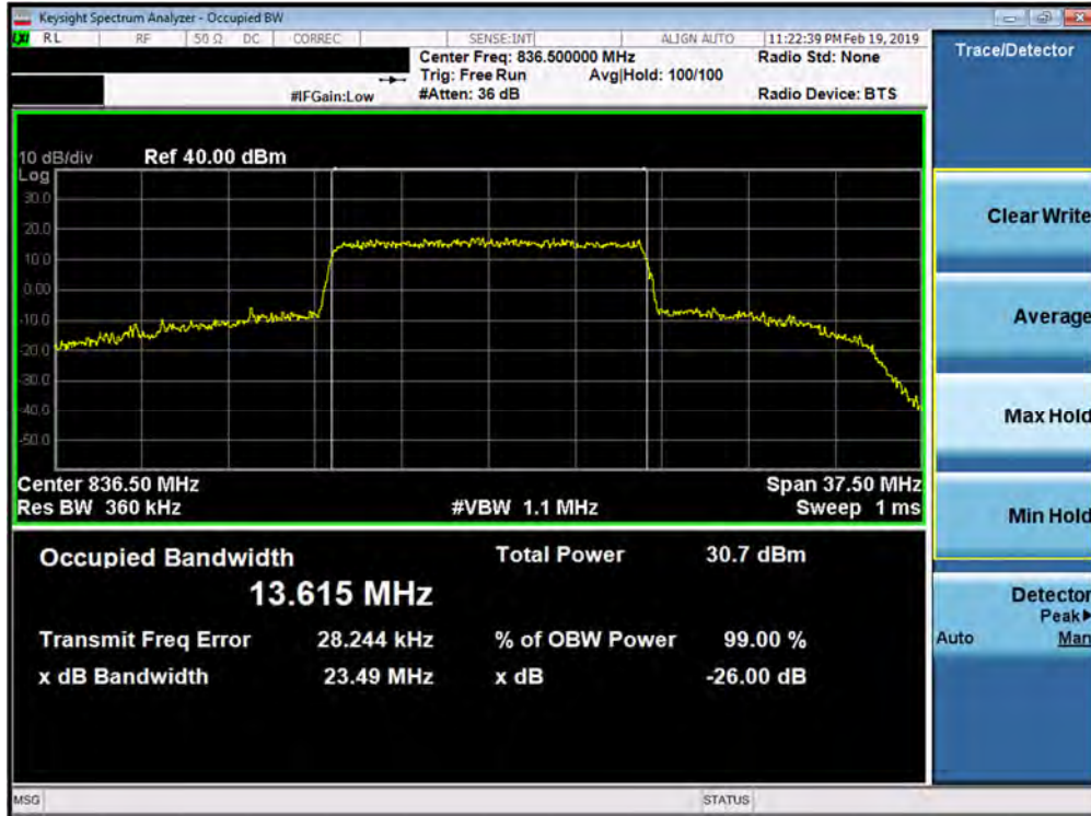
Plot 7-43. Occupied Bandwidth Plot (Band 26 - 15.0MHz 64-QAM - Full RB Configuration)
