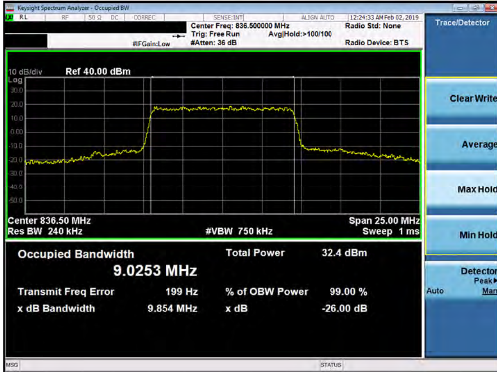
Plot 7-37. Occupied Bandwidth Plot (Band 26/5 - 10.0MHz QPSK - Full RB Configuration)
