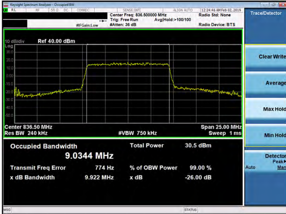
Plot 7-39. Occupied Bandwidth Plot (Band 26/5 - 10.0MHz 64-QAM - Full RB Configuration)
