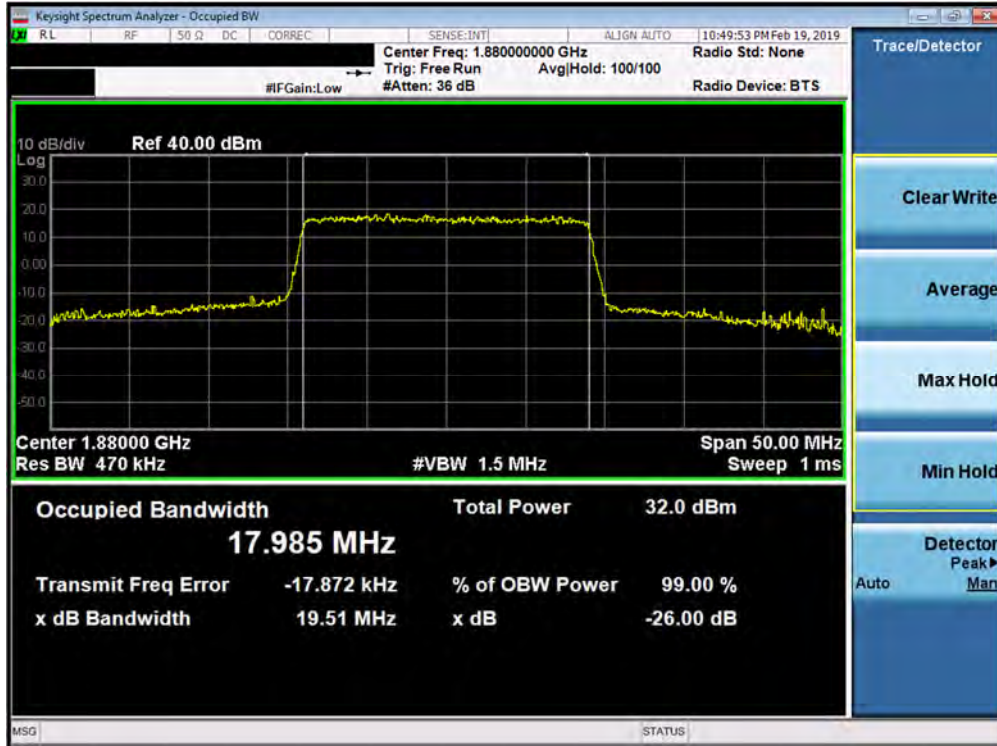
Plot 7-89. Occupied Bandwidth Plot (Band 2 - 20.0MHz QPSK - Full RB Configuration)
