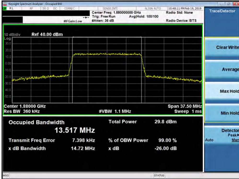
Plot 7-87. Occupied Bandwidth Plot (Band 2 - 15.0MHz 64-QAM - Full RB Configuration)
