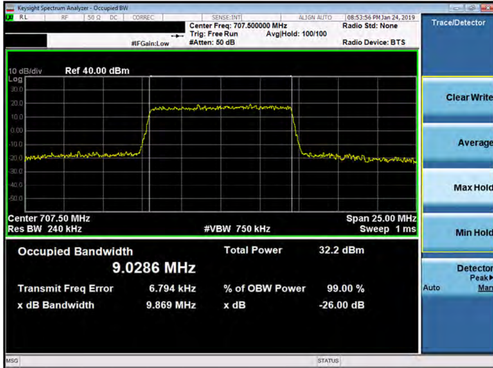
Plot 7-13. Occupied Bandwidth Plot (Band 12 - 10.0MHz QPSK - Full RB Configuration)
