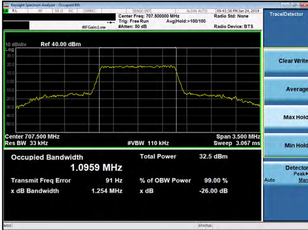
Plot 7-1. Occupied Bandwidth Plot (Band 12 - 1.4MHz QPSK - Full RB Configuration)
