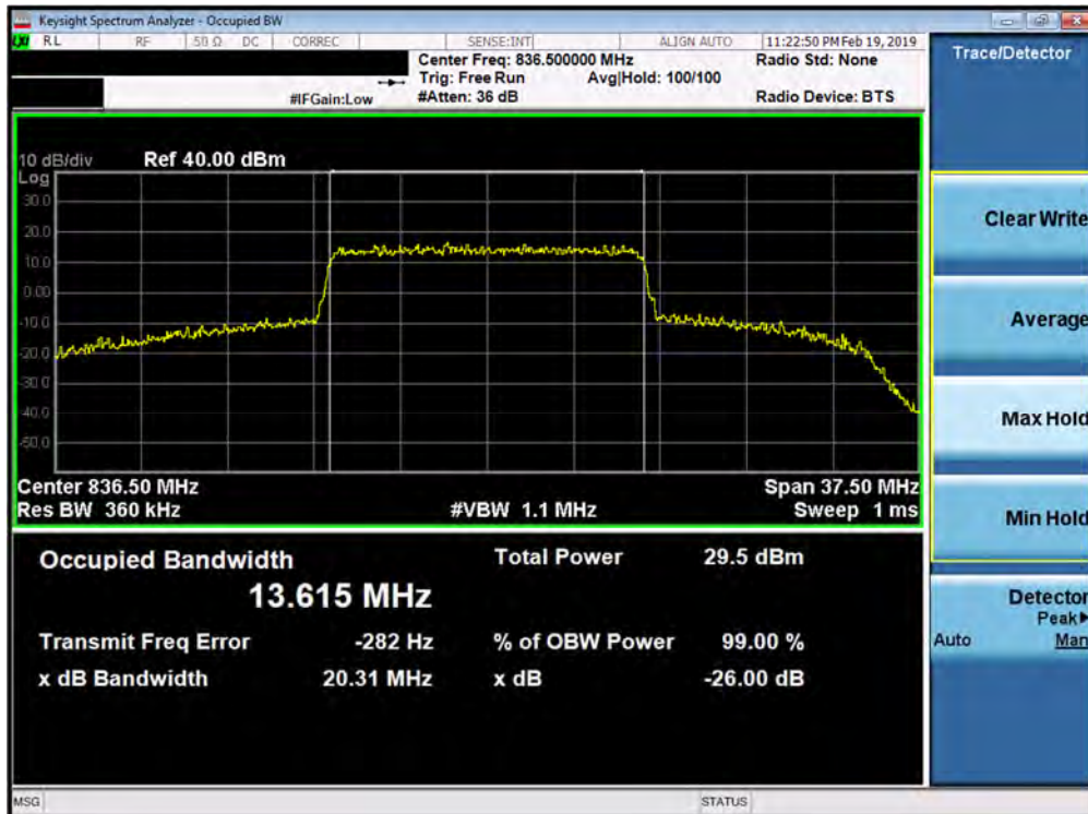
Plot 7-44. Occupied Bandwidth Plot (Band 26 - 15.0MHz 256-QAM - Full RB Configuration)
