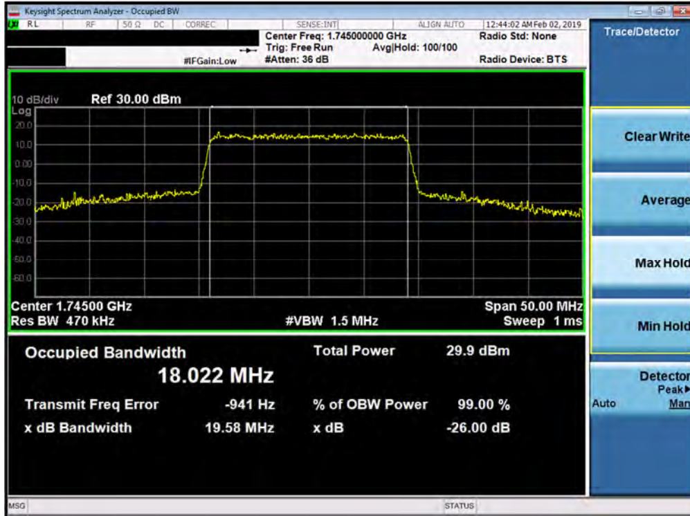
Plot 7-67. Occupied Bandwidth Plot (Band 66/4 - 20.0MHz 64-QAM - Full RB Configuration)
