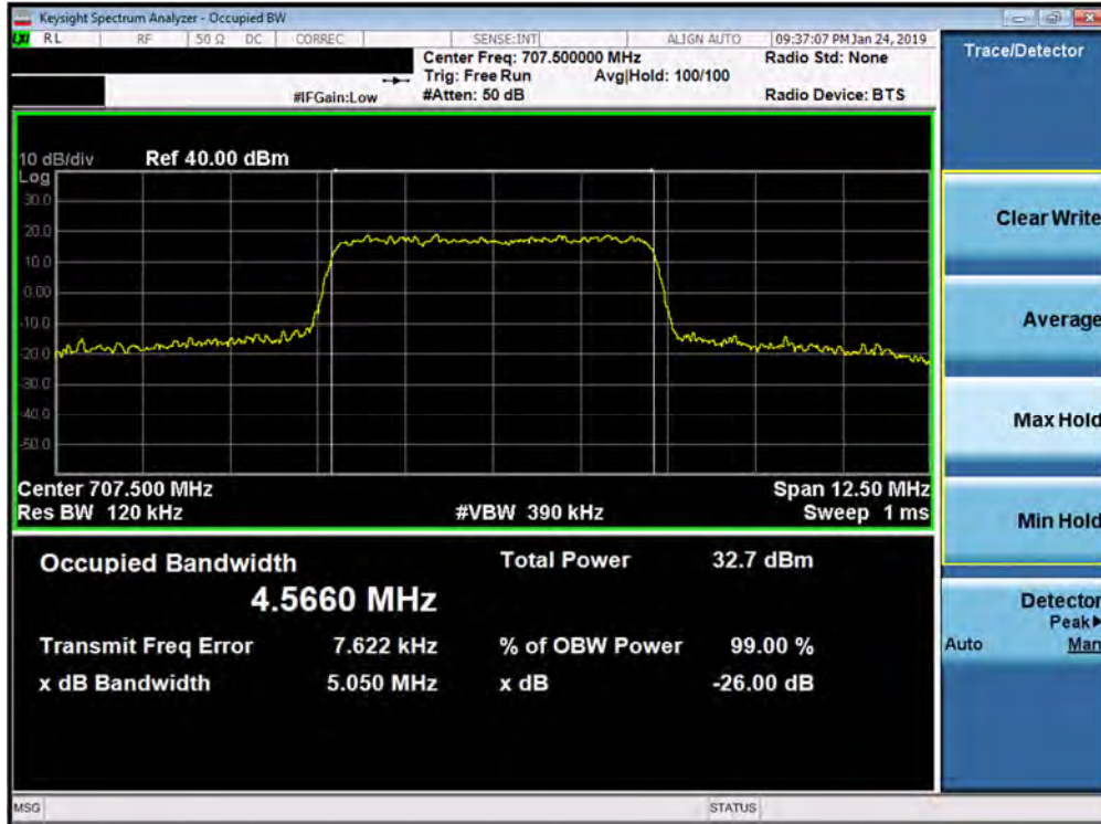
Plot 7-9. Occupied Bandwidth Plot (Band 12 - 5.0MHz QPSK - Full RB Configuration)
