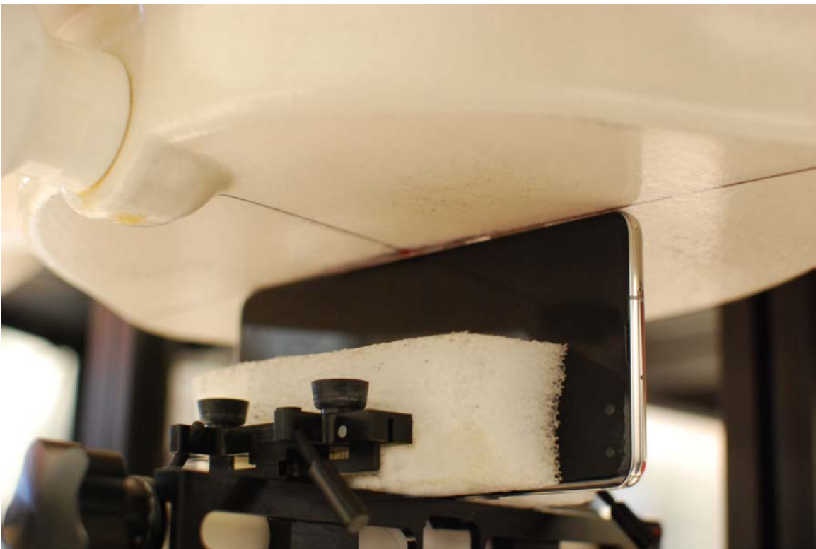
SAR Test Setup Photo 20 – Left Side at 0 mm
