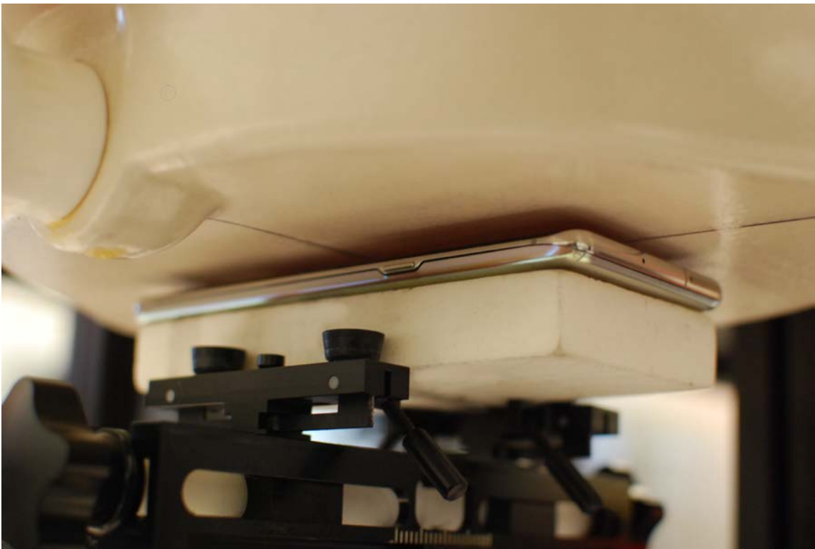
SAR Test Setup Photo 10 – Front Side at 5 mm
