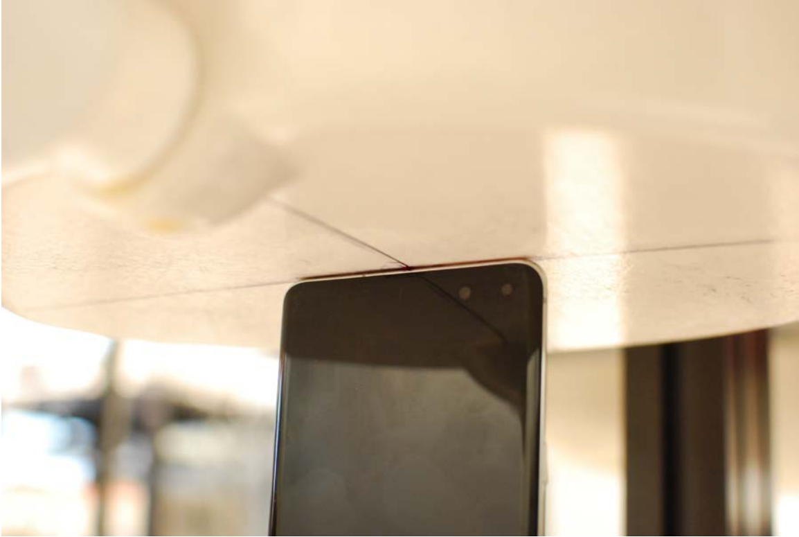
SAR Test Setup Photo 13 – Top Side at 0 mm
