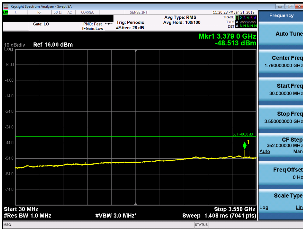
Plot 7-20. Conducted Spurious Plot (Band 48 - 20.0MHz QPSK - RB Size 1, RB Offset 0 - Mid Channel)
