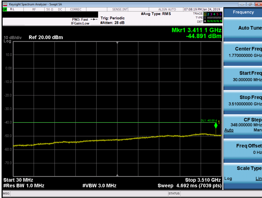
Plot 7-17. Conducted Spurious Plot (Band 48 - 20.0MHz QPSK - RB Size 1, RB Offset 0 - Low Channel)
