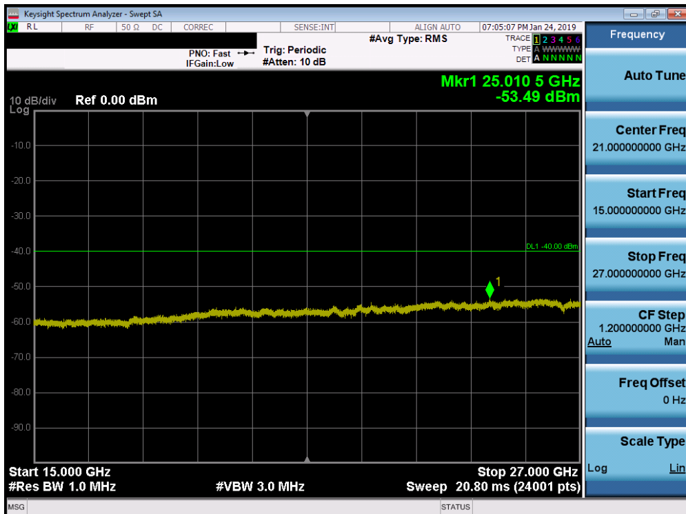
Plot 7-22. Conducted Spurious Plot (Band 48 - 20.0MHz QPSK - RB Size 1, RB Offset 0 - Mid Channel)
