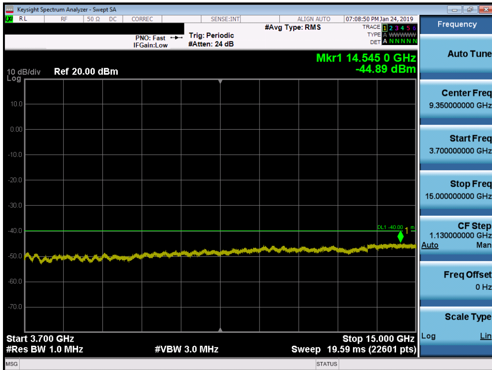
Plot 7-18. Conducted Spurious Plot (Band 48 - 20.0MHz QPSK - RB Size 1, RB Offset 0 - Low Channel)
