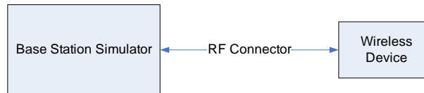
Figure 9-4 Power Measurement Setup
