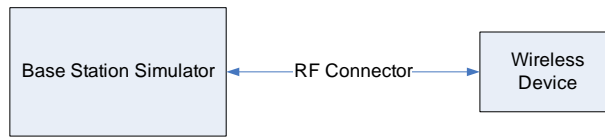
Figure 9-1 Power Measurement Setup
