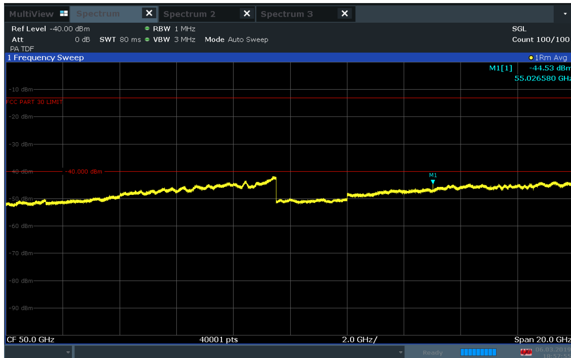
Plot 7-136. K Patch Radiated Spurious Plot 40-60 GHz (1CC QPSK Low Channel V Beam)
