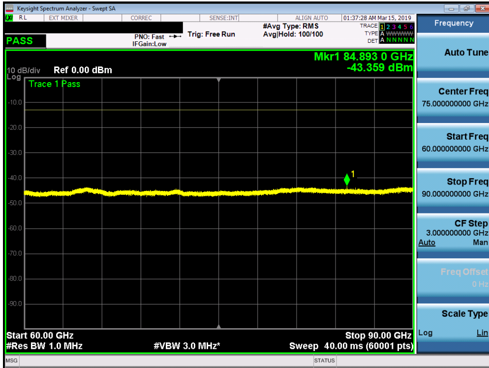
Plot 7-175. L Patch Radiated Spurious Plot 60-90 GHz (1CC QPSK High Channel H Beam)
