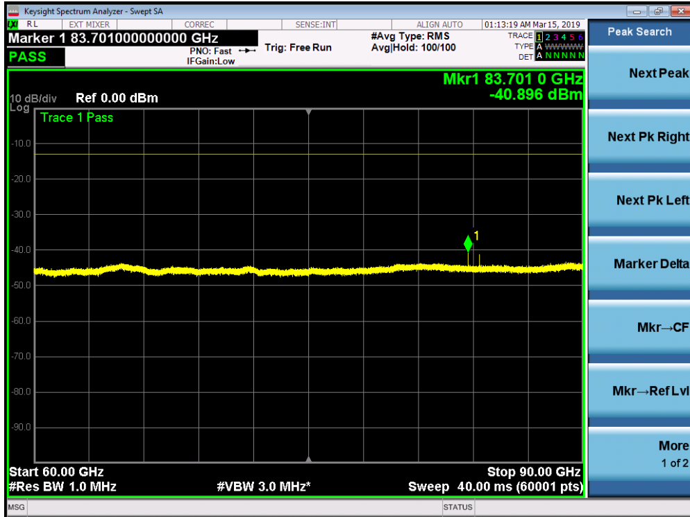
Plot 7-177. L Patch Radiated Spurious Plot 60-90 GHz (1CC QPSK Mid Channel V Beam)
