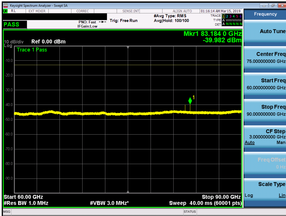
Plot 7-176. L Patch Radiated Spurious Plot 60-90 GHz (1CC QPSK Low Channel V Beam)
