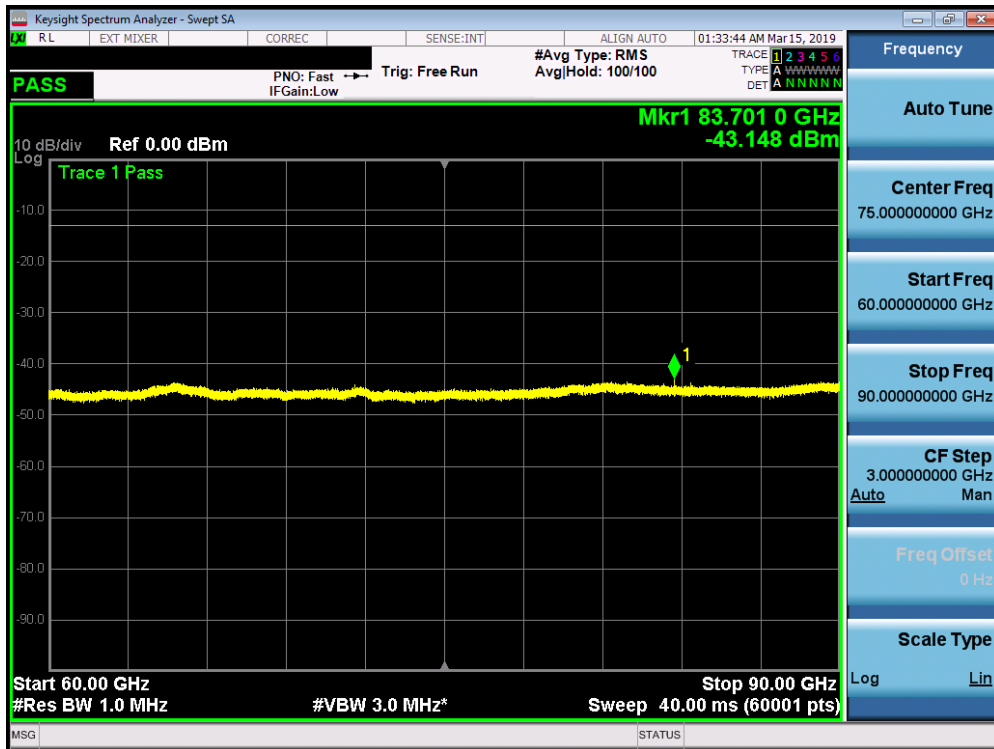
Plot 7-174. L Patch Radiated Spurious Plot 60-90 GHz (1CC QPSK Mid Channel H Beam)
