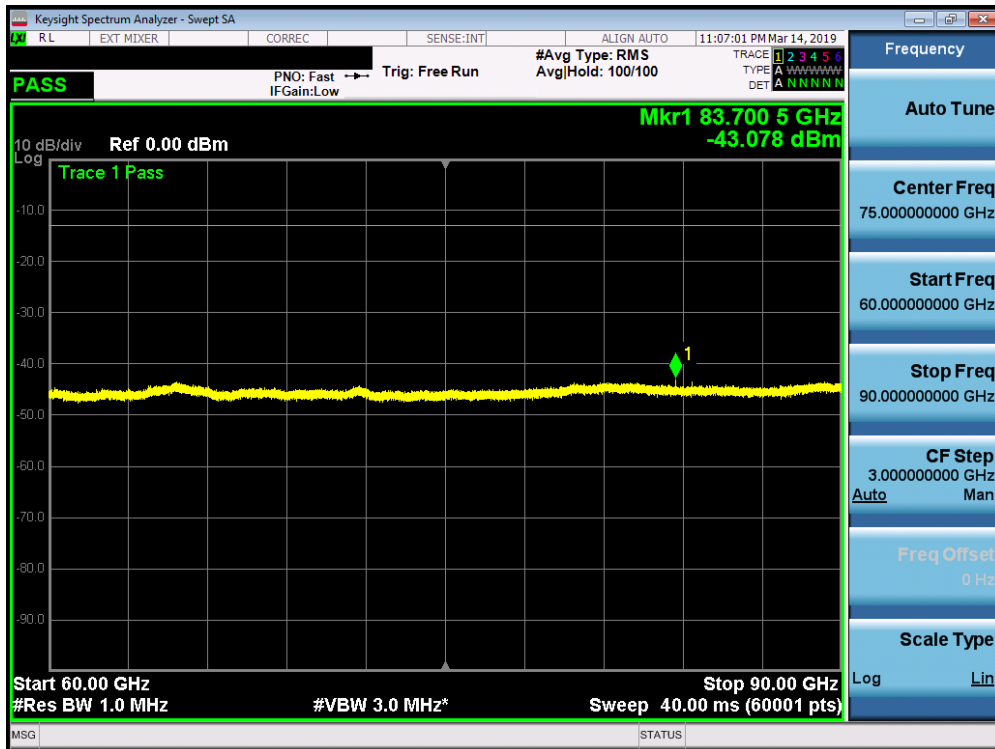
Plot 7-140. K Patch Radiated Spurious Plot 60-90 GHz (1CC QPSK Mid Channel H Beam)
