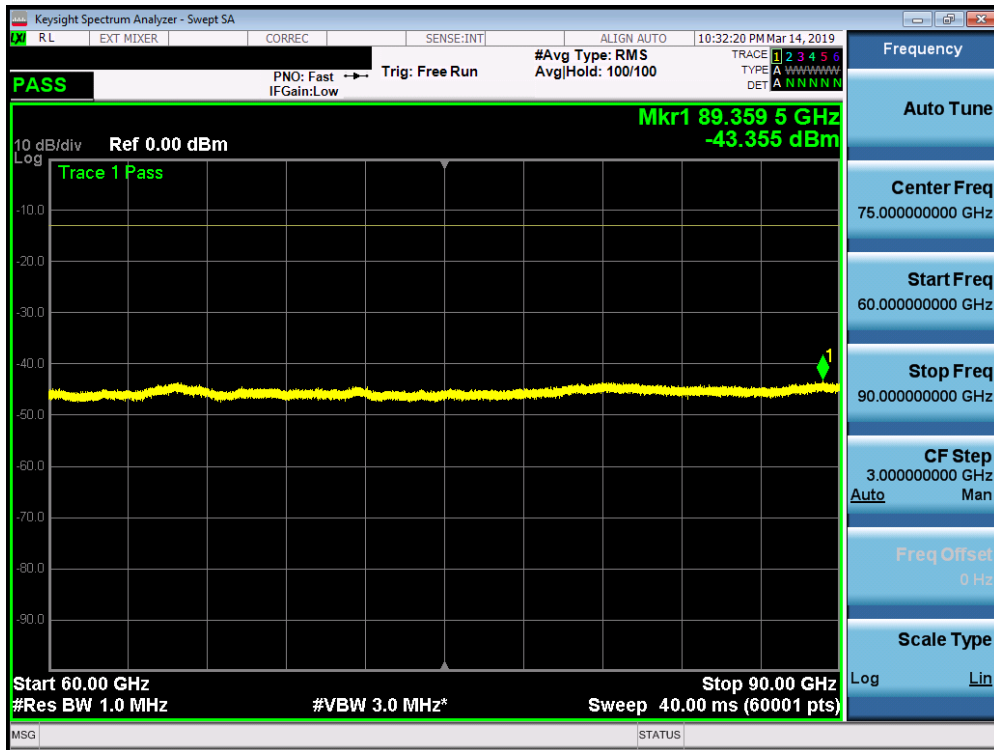
Plot 7-108. J Patch Radiated Spurious Plot 60-90 GHz (1CC 16QAM Low Channel V Beam)
