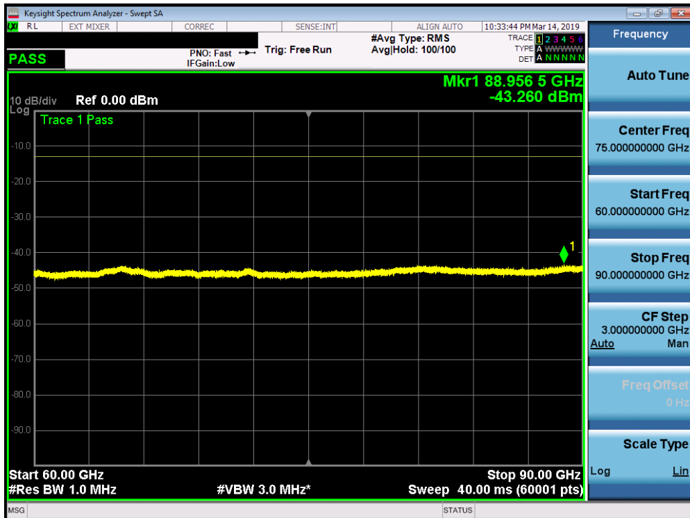
Plot 7-110. J Patch Radiated Spurious Plot 60-90 GHz (1CC 16QAM High Channel V Beam)
