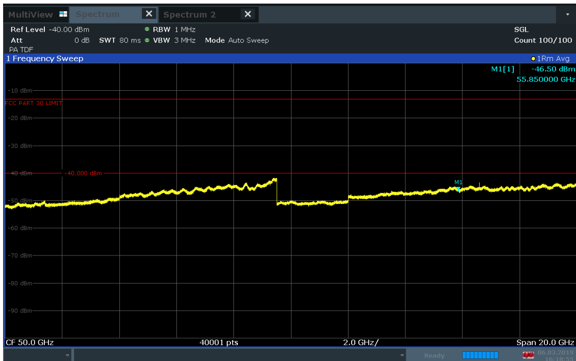
Plot 7-70. J Dipole Radiated Spurious Plot 40-60 GHz (1CC 16QAM High Channel V Beam)
