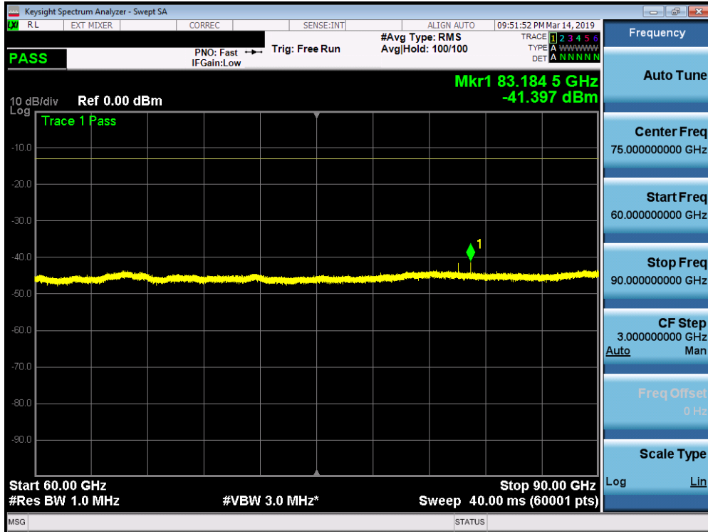
Plot 7-71. J Dipole Radiated Spurious Plot 60-90 GHz (1CC 16QAM Low Channel H Beam)
