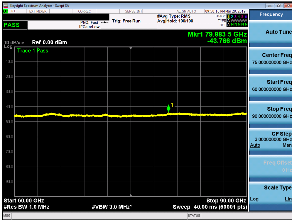
Plot 7-147. K Patch Radiated Spurious Plot 60-90 GHz (1CC QPSK High Channel H Beam)
