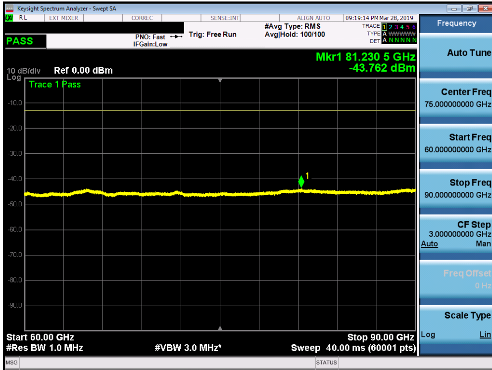
Plot 7-107. J Patch Radiated Spurious Plot 60-90 GHz (1CC QPSK High Channel H Beam)
