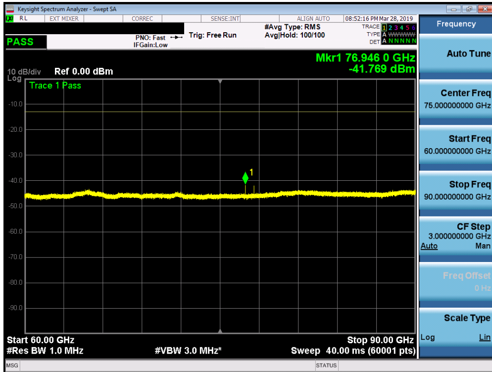
Plot 7-66. J Dipole Radiated Spurious Plot 60-90 GHz (1CC QPSK Mid Channel H Beam)
