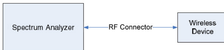
Figure 7-1. Test Instrument & Measurement Setup
