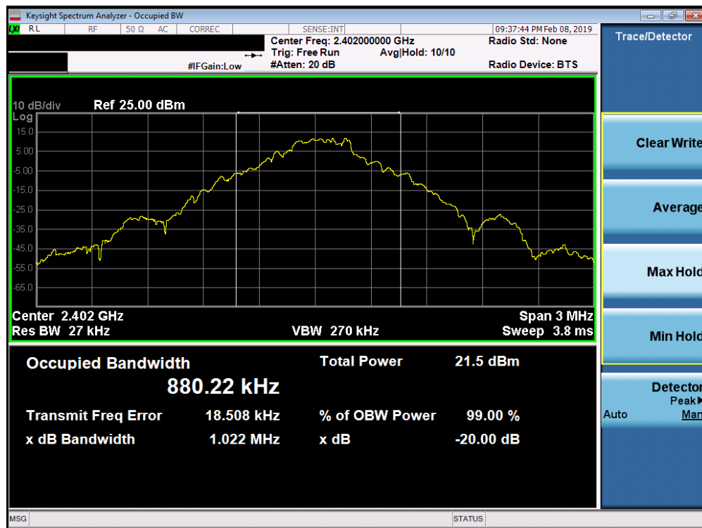
Plot 7-1. 20dB Bandwidth Plot (Bluetooth, 1Mbps – Ch. 0)
