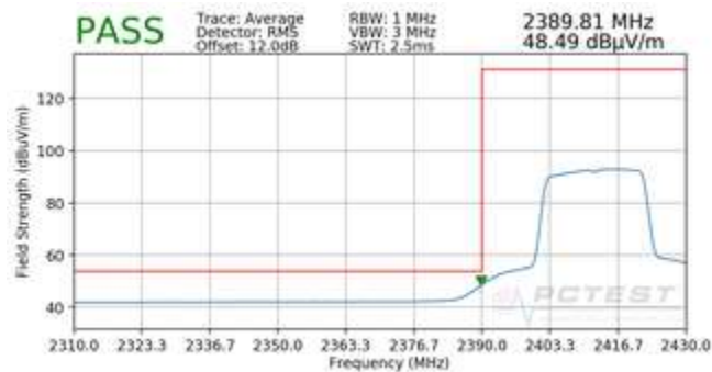
Plot 7-87. Radiated Restricted Band Edge Measurement SISO ANT1 with WCP (Average – 242 Tones)
