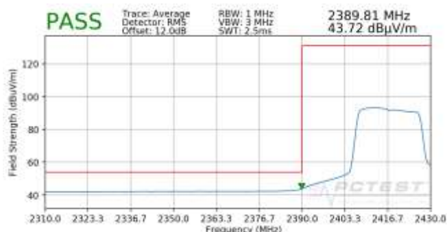
Plot 7-95. Radiated Restricted Lower Band Edge Measurement SISO ANT2 (Average – 242 Tones)
