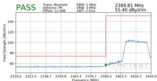
Plot 7-96. Radiated Restricted Lower Band Edge Measurement SISO ANT2 (Peak – 242 Tones)
