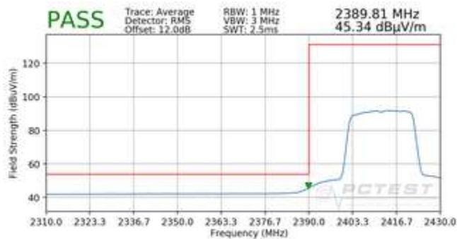
Plot 7-115. Radiated Restricted Band Edge Measurement MIMO with WCP (Average – 242 Tones)
