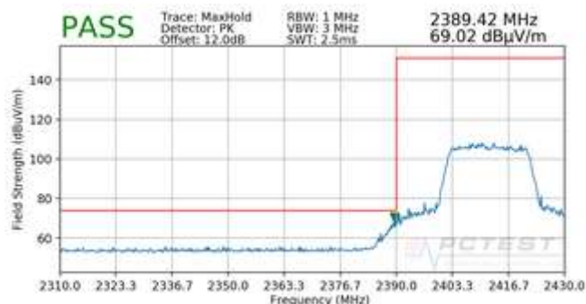
Plot 7-80. Radiated Restricted Lower Band Edge Measurement SISO ANT1 (Peak – 242 Tones)
