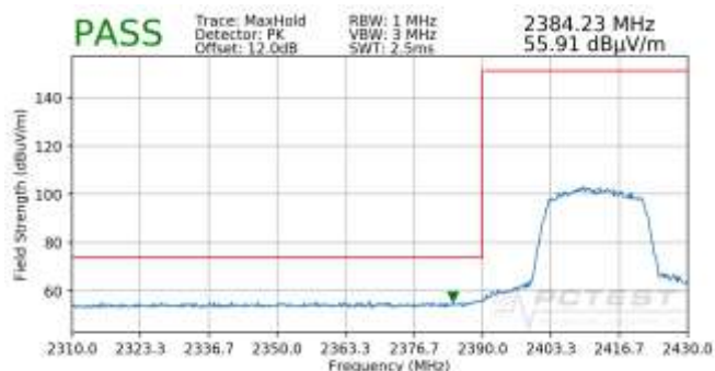
Plot 7-94. Radiated Restricted Lower Band Edge Measurement SISO ANT2 (Peak – 242 Tones)
