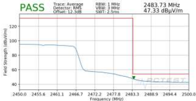
Plot 7-97. Radiated Restricted Upper Band Edge Measurement SISO ANT2 (Average – 242 Tones)
