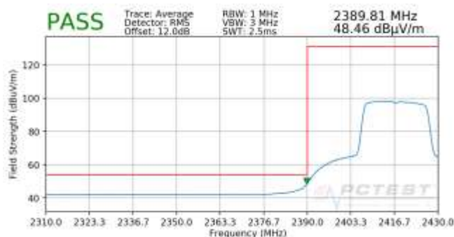
Plot 7-81. Radiated Restricted Lower Band Edge Measurement SISO ANT1 (Average – 242 Tones)
