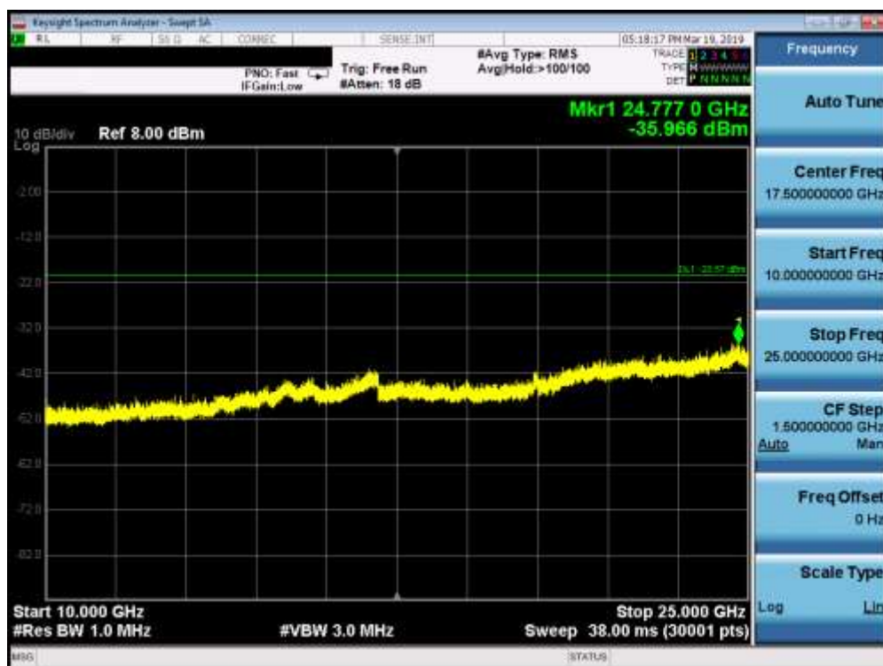
Plot 7-32. Conducted Spurious Plot SISO ANT1 (802.11ax OFDMA– 26 Tones – Ch. 11)
