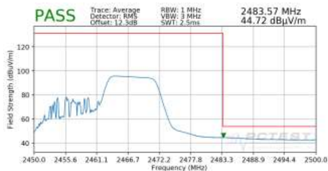
Plot 7-91. Radiated Restricted Upper Band Edge Measurement SISO ANT2 (Average – 106 Tones)
