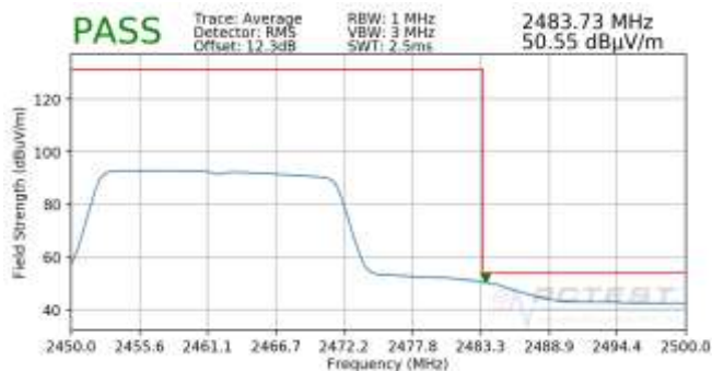
Plot 7-99. Radiated Restricted Upper Band Edge Measurement SISO ANT2 (Average – 242 Tones)
