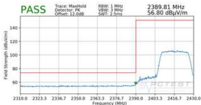
Plot 7-110. Radiated Restricted Lower Band Edge Measurement MIMO (Peak – 242 Tones)
