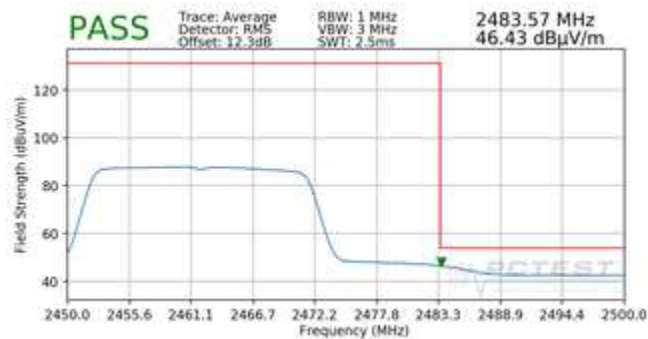
Plot 7-101. Radiated Restricted Band Edge Measurement SISO ANT2 with WCP (Average – 242 Tones)
