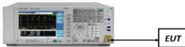
Figure 7-1. Test Instrument & Measurement Setup
