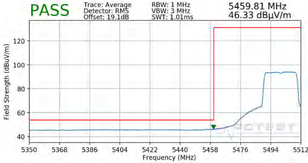
Plot 7-338. Radiated Lower Band Edge Plot SISO ANT2 (Average – UNII Band 2C – 242 Tones)
