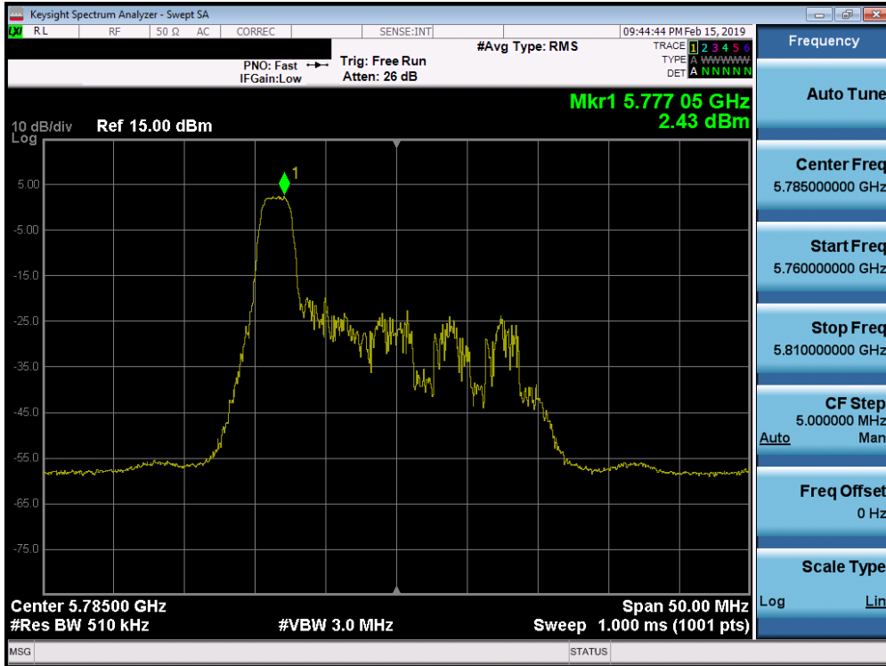
Plot 7-266. Power Spectral Density Plot MIMO ANT2 (20MHz BW 802.11ax – 26 Tones (UNII Band 3) – Ch. 157)
