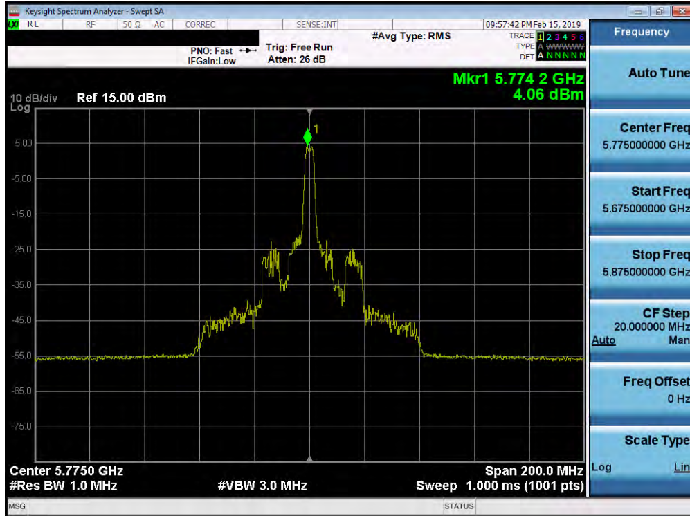
Plot 7-270. Power Spectral Density Plot MIMO ANT2 (80MHz BW 802.11ax – 26 Tones (UNII Band 3) – Ch. 155)
