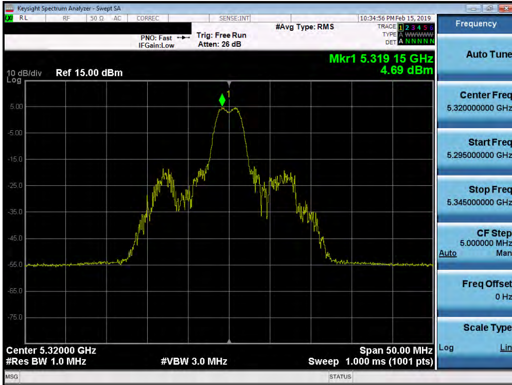
Plot 7-225. Power Spectral Density Plot MIMO ANT1 (20MHz BW 802.11ax – 26 Tones (UNII Band 2A) – Ch. 64)
