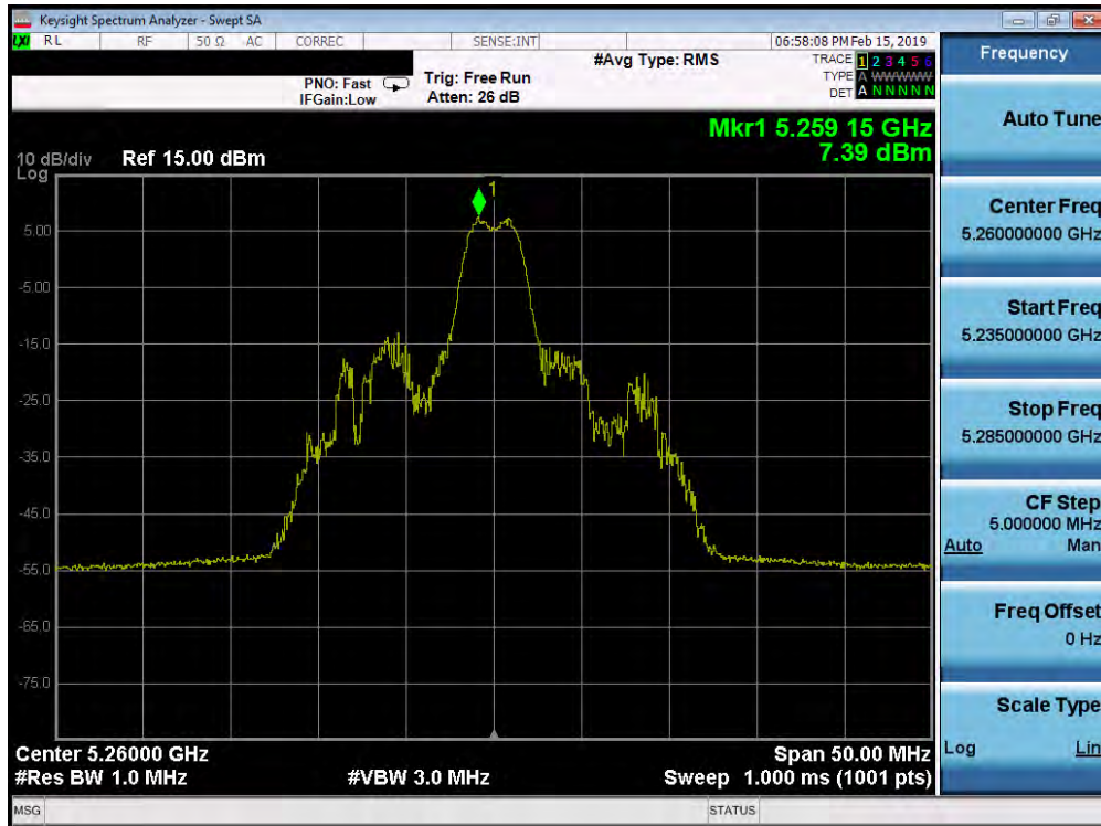
Plot 7-169. Power Spectral Density Plot SISO ANT2 (20MHz BW 802.11ax – 26 Tones (UNII Band 2A) – Ch. 52)
