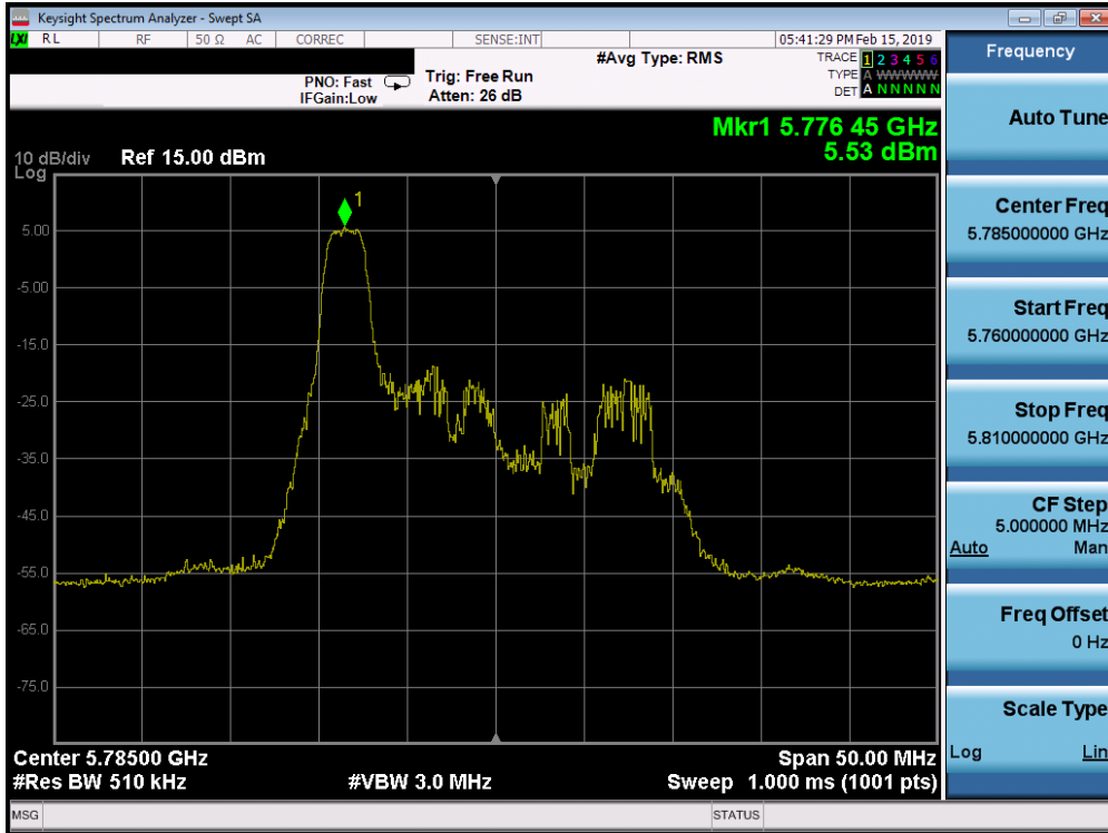
Plot 7-131. Power Spectral Density Plot SISO ANT1 (20MHz BW 802.11ax – 26 Tones (UNII Band 3) – Ch. 157)
