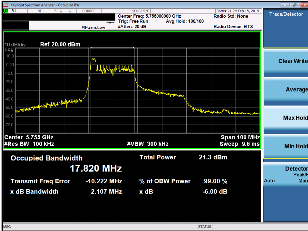
Plot 7-88. 6dB Bandwidth Plot SISO ANT1 (40MHz BW 802.11ax – 26 Tones (UNII Band 3) – Ch. 151)
