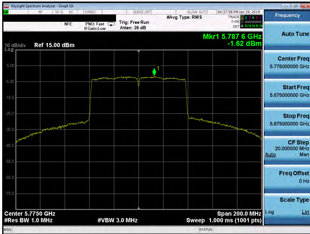
Plot 7-197. Power Spectral Density Plot SISO ANT1 (80MHz BW 802.11ac (UNII Band 3) – Ch. 155)
