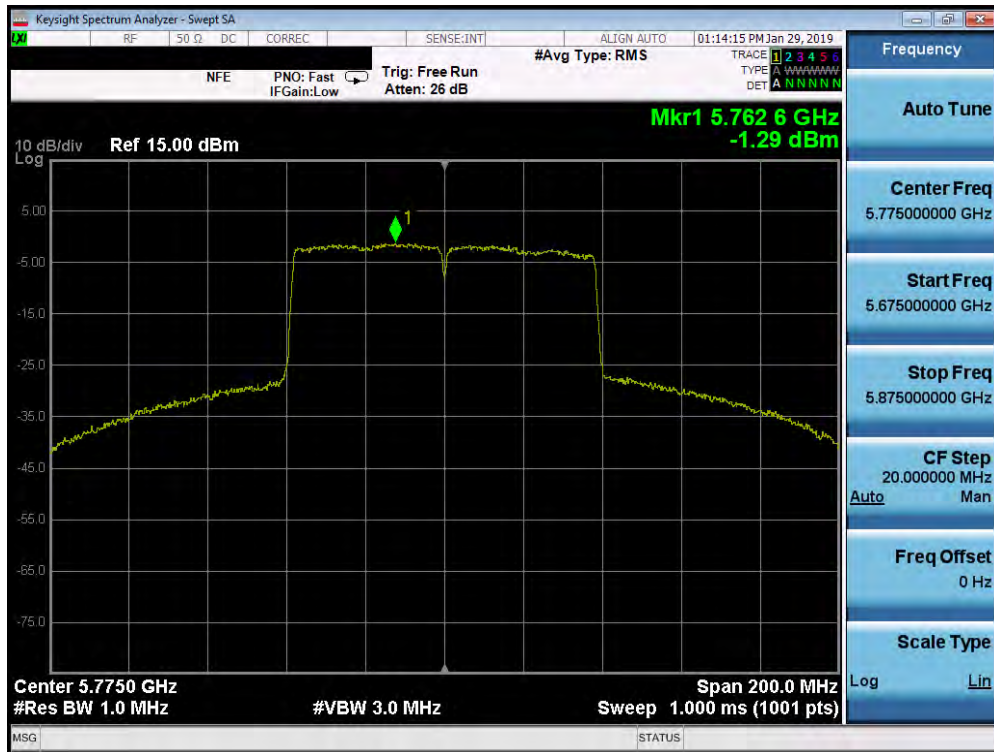
Plot 7-263. Power Spectral Density Plot SISO ANT2 (80MHz BW 802.11ac (UNII Band 3) – Ch. 155)
