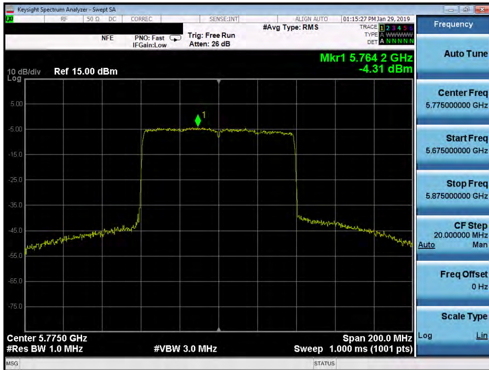
Plot 7-264. Power Spectral Density Plot SISO ANT2 (80MHz BW 802.11ax (UNII Band 3) – Ch. 155)
