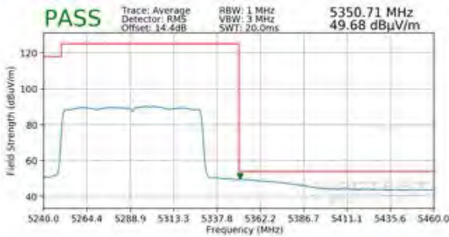
Plot 7-312. Radiated Upper Band Edge Plot SISO ANT1 (Average – UNII Band 2A)
