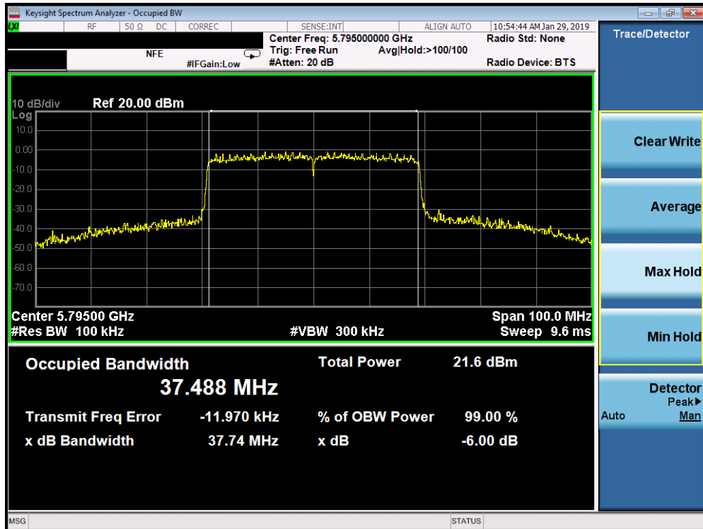
Plot 7-115. 6dB Bandwidth Plot SISO ANT1 (40MHz BW 802.11ax (UNII Band 3) – Ch. 159)
