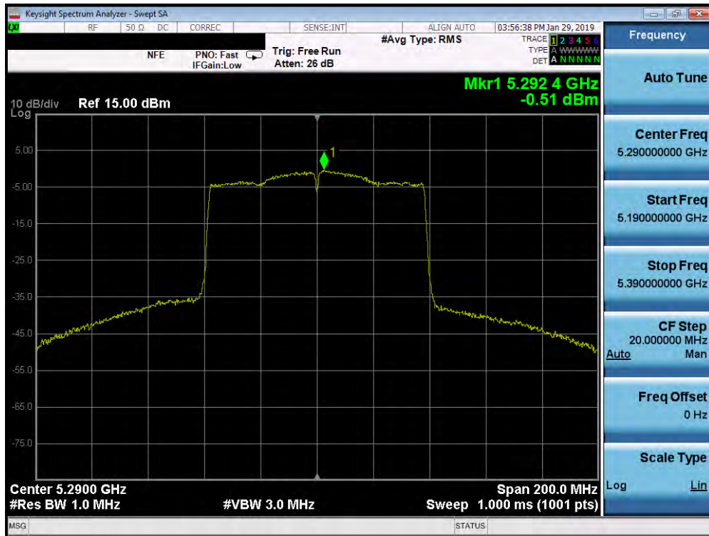
Plot 7-161. Power Spectral Density Plot SISO ANT1 (80MHz BW 802.11ac (UNII Band 2A) – Ch. 58)
