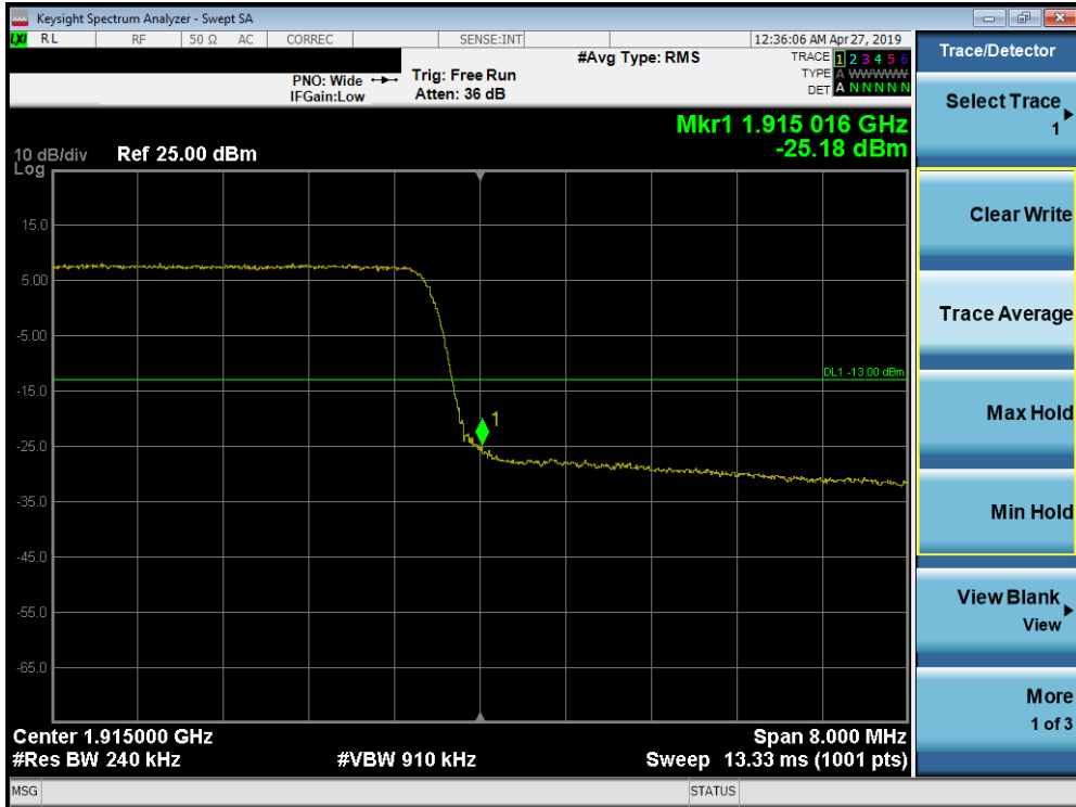
Plot 7-324. Upper Band Edge Plot (Band 25 - 10.0MHz QPSK - Full RB Configuration)
