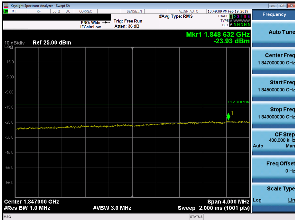
Plot 7-327. Lower Extended Band Edge Plot (Band 25/2- 15.0MHz QPSK - Full RB Configuration)
