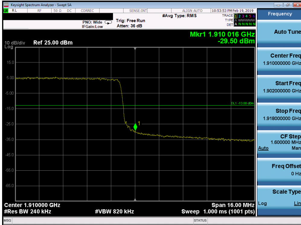
Plot 7-334. Upper Band Edge Plot (Band 2 - 20.0MHz QPSK - Full RB Configuration)
