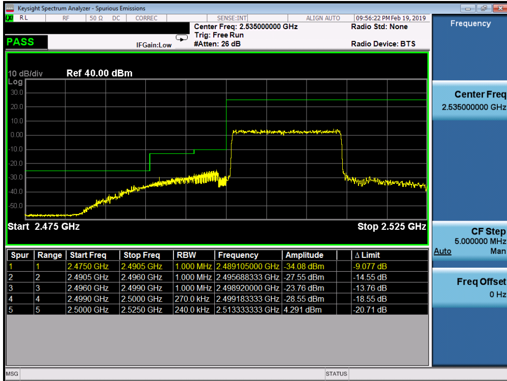
Plot 7-342. Lower ACP Plot (Band 7 - 15.0MHz QPSK - Full RB Configuration)
