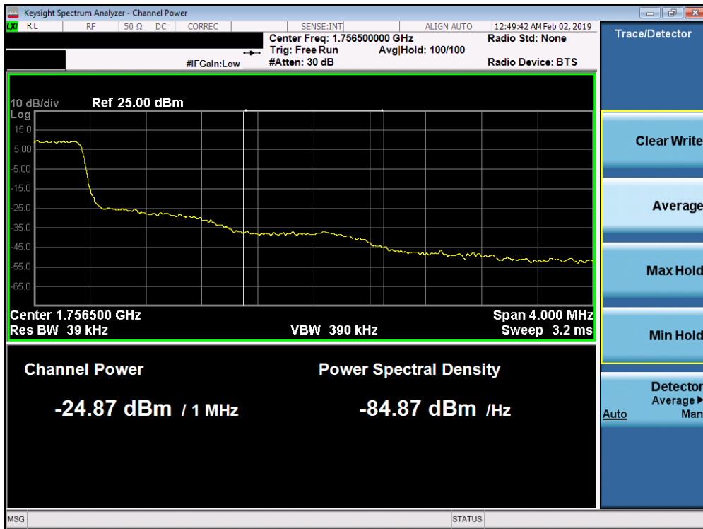
Plot 7-269. Upper Extended Band Edge Plot (Band 4 - 1.4MHz QPSK - Full RB Configuration)
