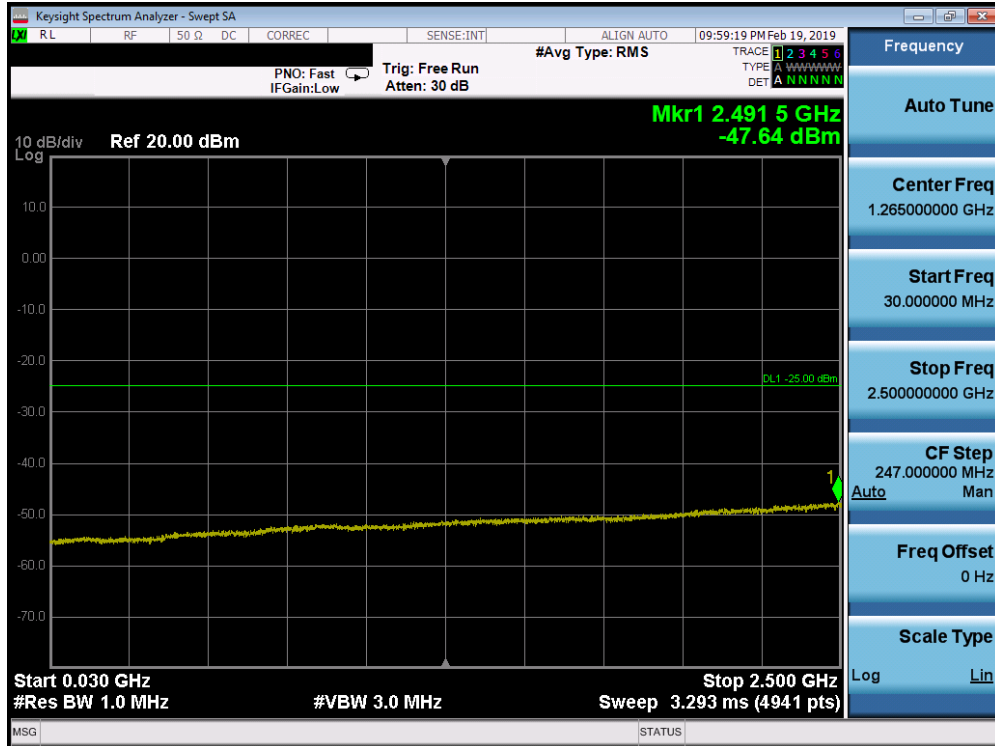
Plot 7-211. Conducted Spurious Plot (Band 7 - 20.0MHz QPSK - RB Size 1, RB Offset 0 - High Channel)
