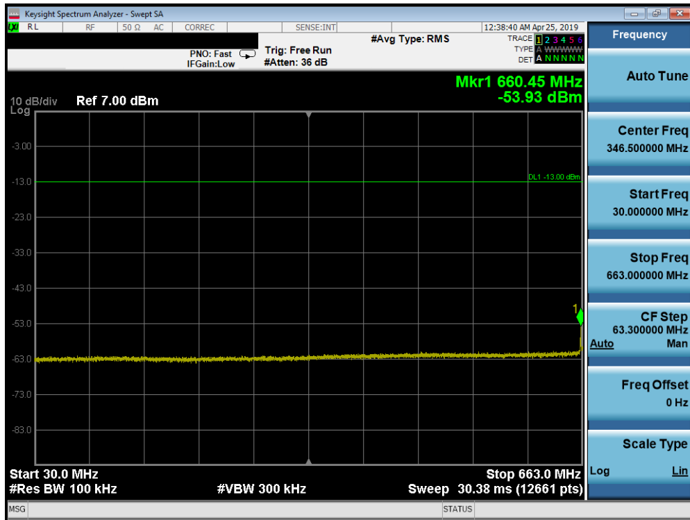
Plot 7-160. Conducted Spurious Plot (Band 71 - 20.0MHz QPSK - RB Size 1, RB Offset 0 - Mid Channel)
