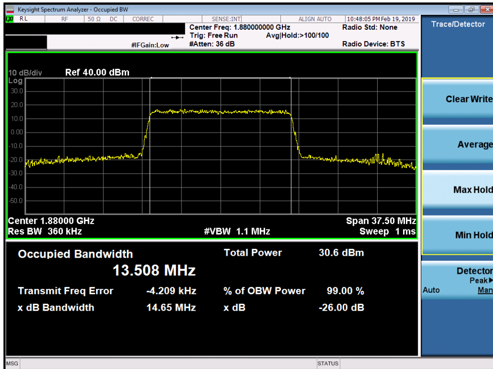
Plot 7-102. Occupied Bandwidth Plot (Band 25/2 - 15.0MHz 16-QAM - Full RB Configuration)
