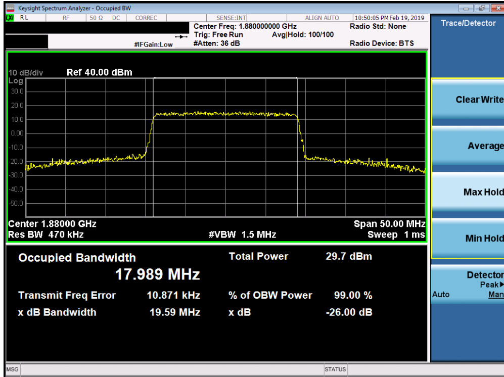
Plot 7-107. Occupied Bandwidth Plot (Band 25/2 - 20.0MHz 64-QAM - Full RB Configuration)
