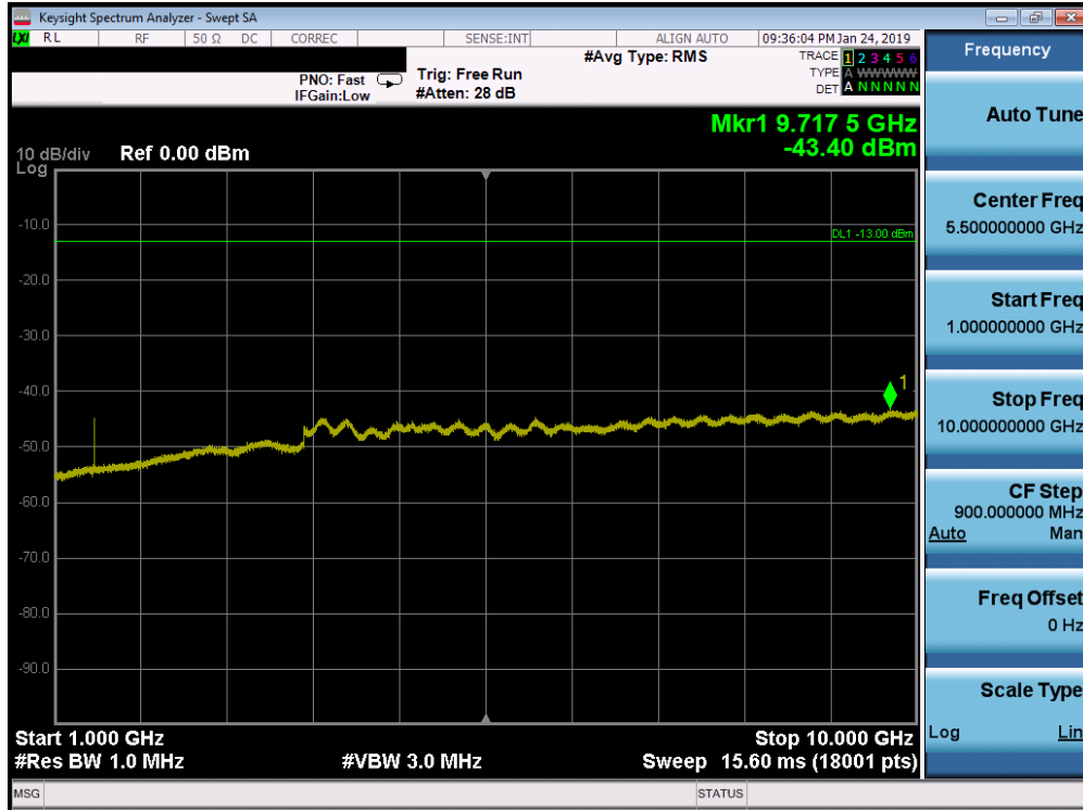
Plot 7-174. Conducted Spurious Plot (Band 12 - 10.0MHz QPSK - RB Size 1, RB Offset 0 - High Channel)
