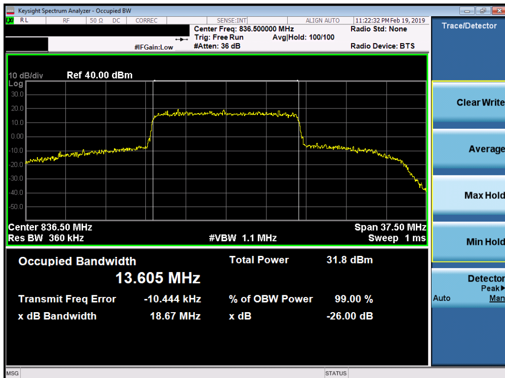
Plot 7-58. Occupied Bandwidth Plot (Band 26 - 15.0MHz 16-QAM - Full RB Configuration)
