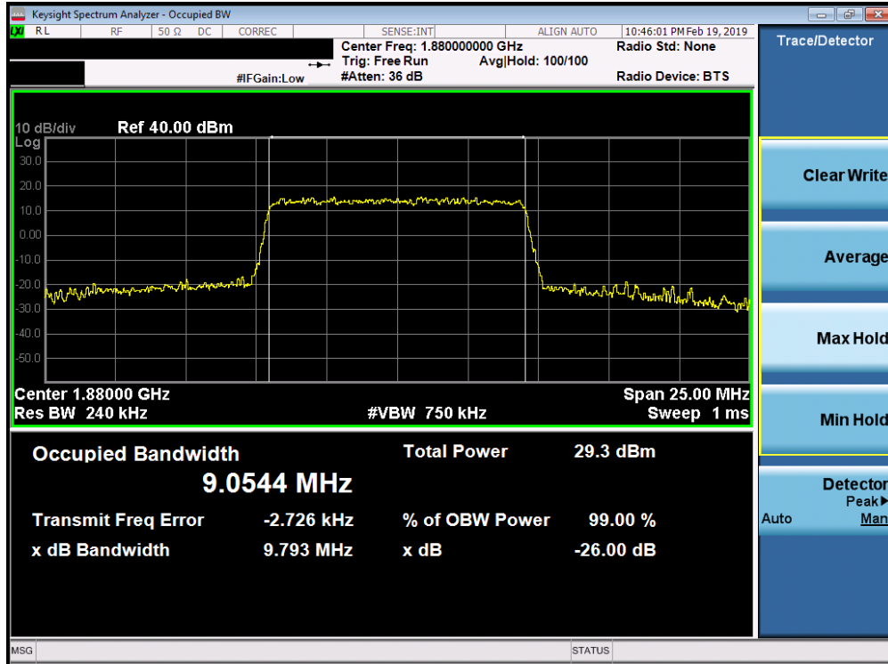
Plot 7-99. Occupied Bandwidth Plot (Band 25/2 - 10.0MHz 64-QAM - Full RB Configuration)
