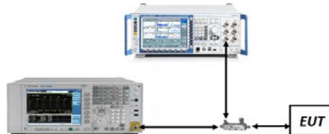
Figure 7-3. Test Instrument & Measurement Setup
