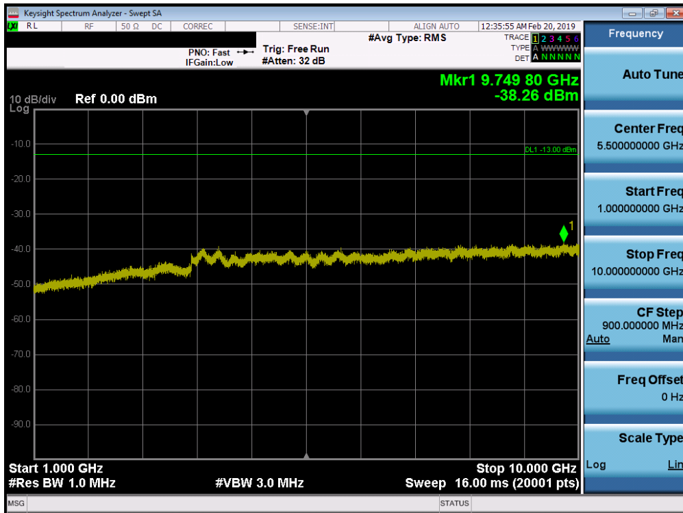
Plot 7-31. Conducted Spurious Plot (LTE Band 26, 15MHz QPSK – RB Size 1, RB Offset 0 – Mid Channel)
