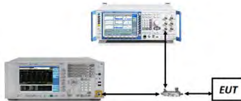
Figure 7-4. Test Instrument & Measurement Setup
