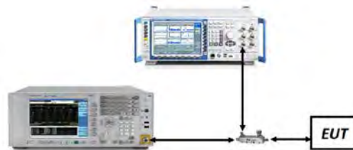
Figure 7-3. Test Instrument & Measurement Setup
