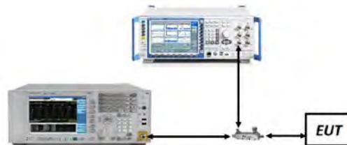
Figure 7-2. Test Instrument & Measurement Setup
